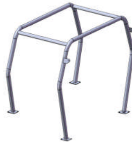
Four-Point Roll-Cage for Extra and Dual Cab Utilities
