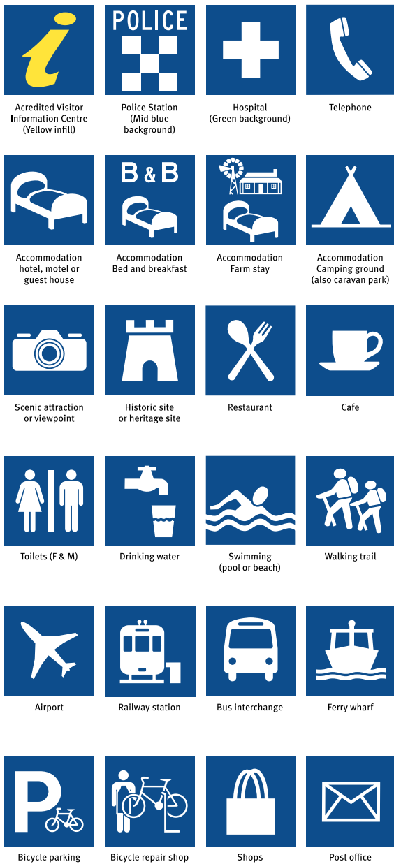
Figure 18: Recommended logos for use on cycle network facilities and services signage. See Figure 18 for examples of use. Logos are white on a dark blue (standard services colour) background. Logos shown are relevant to signing cycle routes. For additional logos refer to MUTCD and Australian Standard AS1742.
