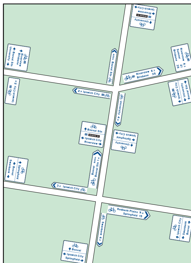
Figure 12: Detail signing for intersection c and the Booval focal point intersection. Detail from Figure 11. Ipswich City to Brisbane route is Level of Signing (LOS) C1. All other principal routes are shown LOS C2.
