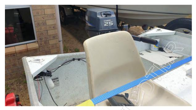
Outboard fitted to the vessel, tiller steer
