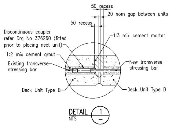
Note: threads are to suit both new and existing bars. Existing thread to be verified on site prior to design development for widening works).
