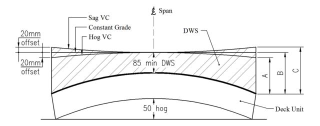
Thickness of DWS at kerb at abutments and piers (crowned pavement).
