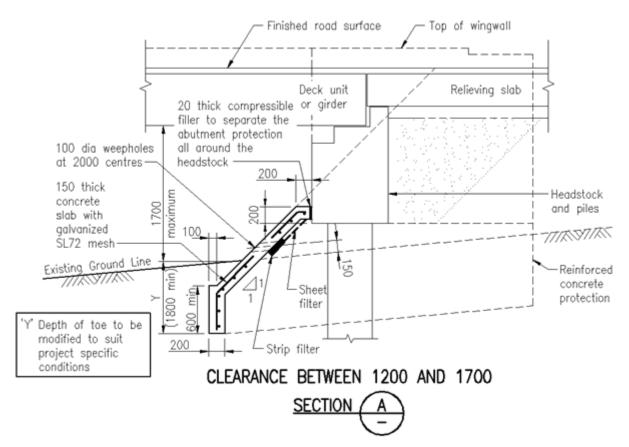
Figure 13.7-3 Inspection Height between 1200 mm and 1700 mm
