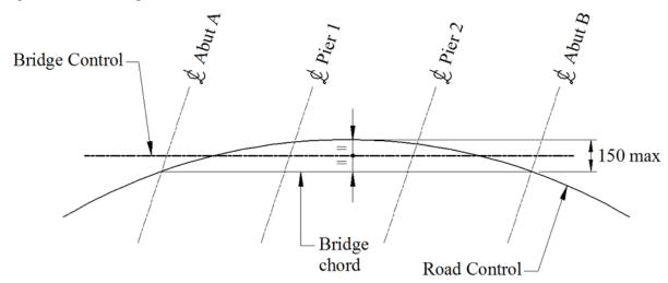
Figure 10.4-2 - Bridge Offset 150 mm Maximum
