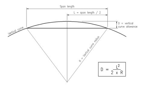
On a sag VC, an additional allowance is added to the deck thickness. Therefore the deck thickness at the abutments and piers is the minimum deck thickness at midspan, plus the hog, minus the pre-camber, plus the VC allowance. A check of the additional deck thickness shall be undertaken to ensure overloading of the abutments and piers does not occur. Refer Figure 17.9-1 *Vertical Curve Allowance*.
