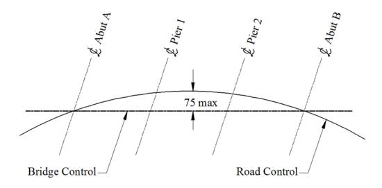
Bridge offset from the chord to the Road Control is greater than 75 mm but less than 150 mm
