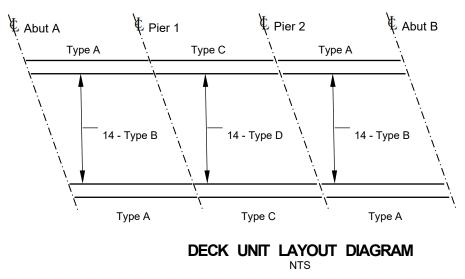
For girder bridges these details are shown on the Miscellaneous Details drawing when the diagram is used to layout steelwork (bearing restraint plates) as well as the girders. Refer Figure 11.7(e) - Girder layout diagram.
