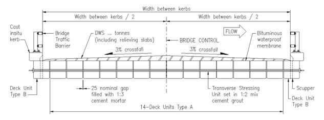
**Decks with Constant Crossfall or Superelevation.** Refer Figure 7.4-2 - Decks with Constant Crossfall/Superelevation.
