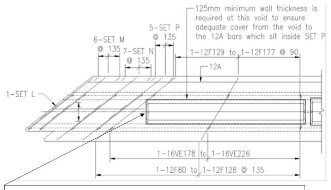
To reduce the chance of cracking, additional reinforcement is required near this face of the void at both ends of the girder.
