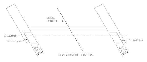
On skewed bridges the Drafter must check that the abutment side walls will not interfere with the transverse stressing of the deck units. The side wall may need to be terminated to provide sufficient working room between it and the jack. Refer Figure 12.4(e) *Abutment Side Wall and Transverse Stressing Jack Clearance*.
