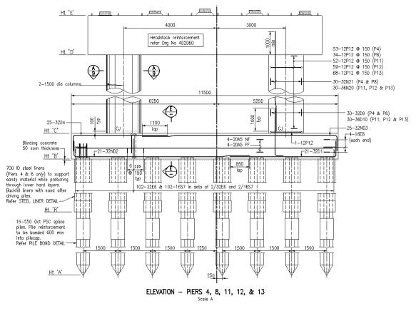
Figure 3.13-1 - Typical Reinforcement Detailing
