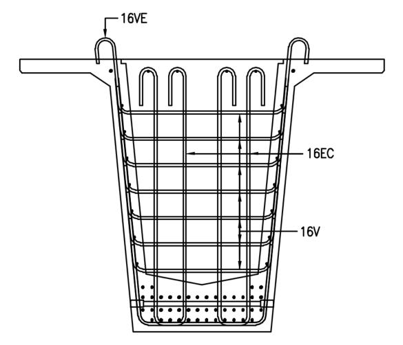
Figure 14.7(b) - Typical reinforcing set in diaphragms and around voids (1500 deep girders)
