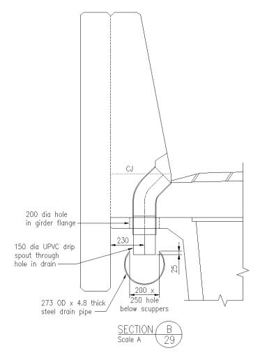
The drain pipe is supported by a steel drain bracket which passes through 20 mm diameter holes in the girder flange. Refer *Figure 14.10(a) - Plan view of hole layout* and *Figure 14.10(c) - 200 mm diameter holes in girder flange drain bracket.*
