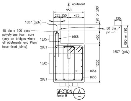
If the bridge deck has crossfall both ways from the bridge centreline and the abutment ballast wall ignores the crossfall, the relieving slab will require end thickening. The highest bar and lowest bars must be dimensioned on the abutment drawing. The starter bars shall all be the same size and shall be bonded a minimum of 500 mm into the ballast wall. Refer Transport and Main Road's Standard Drawings 1505 and 1506 and Figure 12.17(c) *Variable Relieving Slab Starter Bars*.
