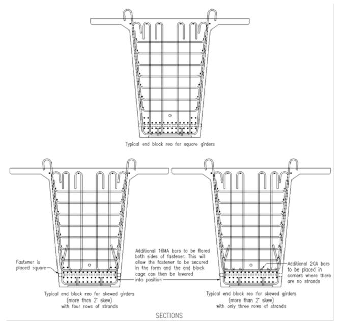
Figure 14.7(e) - Girder reinforcement around fastener (2)
