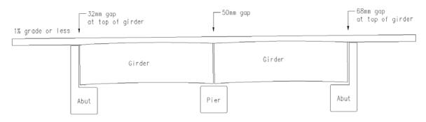
For bridges on a grade of 1% or less, the ends of the girders are not vertical, but are perpendicular to the bottom of the girder (after 100 days).
