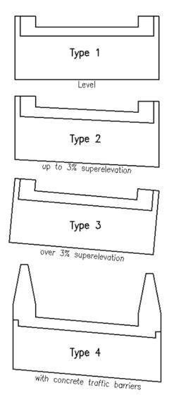
Figure 12.10(a) - Abutment headstock elevation options
