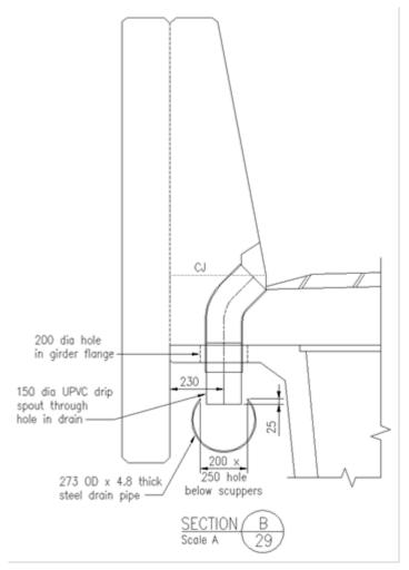
To reduce the chance of cracking around the 200 mm diameter holes, four trimmer bars shall be placed around each hole. Refer *Figure 14.10(d)* - *Trimmer reinforcement bars*.
