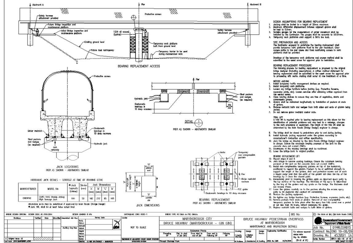
Jocking shall be imited to a height of 20mm maximum. Maximum differential displacement between adjacent girdere shall be kept to 3.5mm. Suitable gauges for the measurement of grider moviement shall be installed by the Contractor. The gauges shall be accurate to ±0.01mm. Temporary work platforms shall support a 5kPa ive load.
