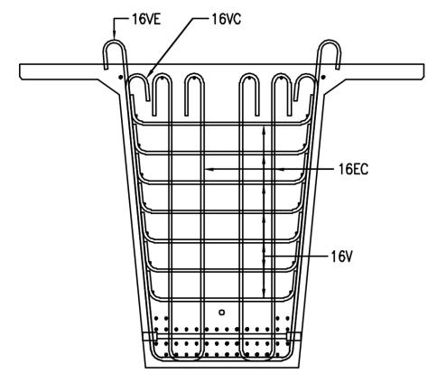
Figure 14.7(a) - Typical reinforcing set - end blocks
