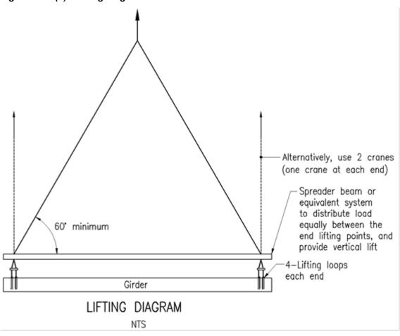
Figure 14.11(a) - Lifting diagram
