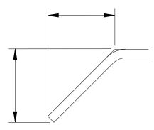
When the angle for a bar shape can be either acute or obtuse, for example bar shape U, the computer calculates the angle and dimension C.
