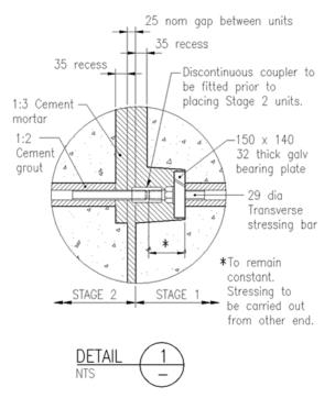
Figure 15.13-2 Recess for Stage Construction
