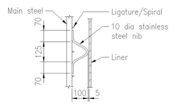
1 set of 4 stainless steel nibs (equally spaced around the circumference of the cage) to be welded securely to main steel at intervals of 4000 maximum on welded cages and 2500 maximum on unwelded cages. There must be at least 2 sets of stainless steel nibs per cage. Stainless steel nibs shall be placed approximately in line and straddle the ligature/spiral as shown
