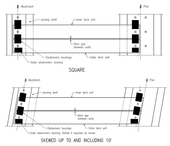
Figure 12.15(a) - Alignment of bearings on deck unit bridges skewed ≤10°
