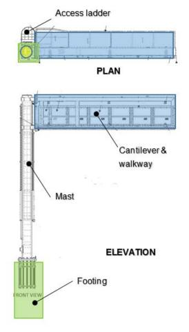
Figure 21.6(a) - Single Post Cantilever Gantry
