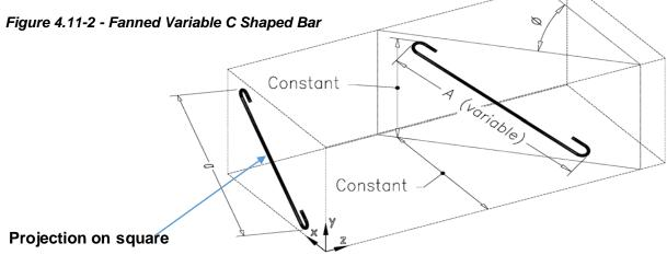
C bar without dimensions parallel to x and y axis cannot be solved by the steel program
