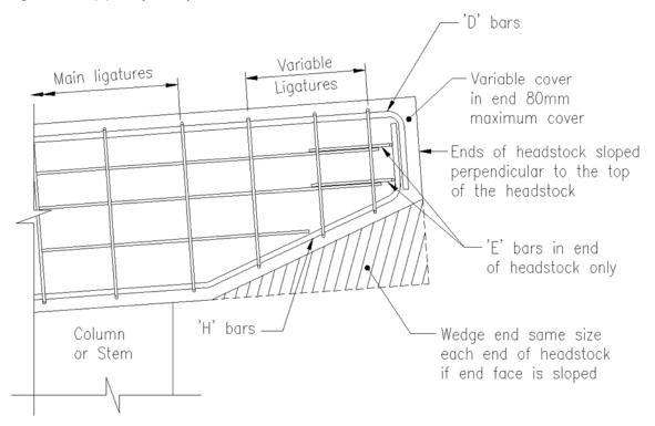
Figure 12.14(b) - Tapered pier headstocks – Reinforcement
