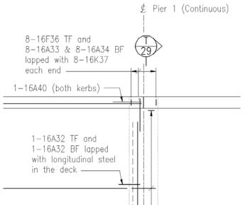
PLAN – DECK Multilayered Reinforcement
