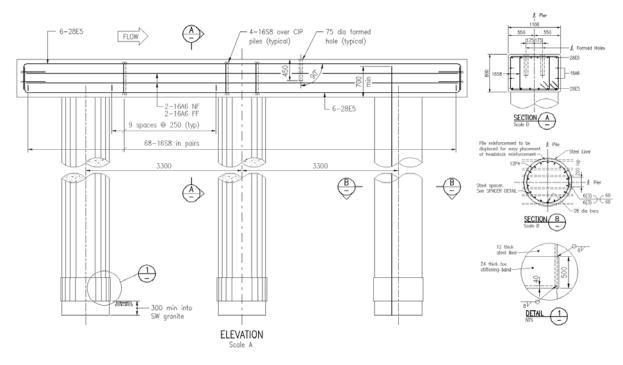
Figure 2.7-2 - Examples of Sections and Details
