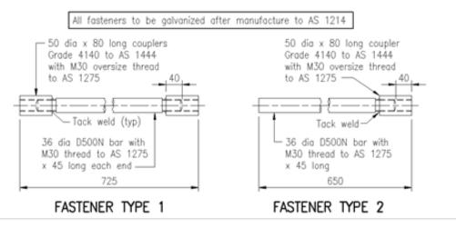
A detailed view (minimum scale of 1:10 on an A1 drawing) shall show how the fasteners, top attachment plate and reinforcing steel fit together in the end block.
