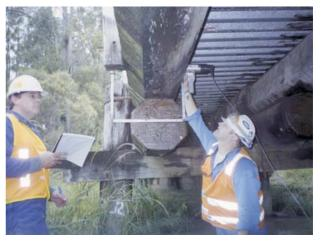
Figure 4b : "Lixi Profiler" in operation
