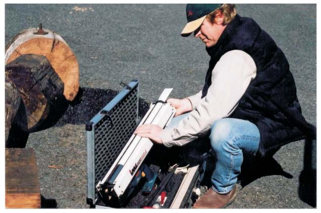
Figure 8- The "Resistograph" being loaded with paper to record the test.
