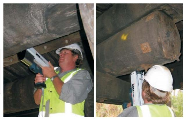
Figure 9a - Horizontal test using the "Resistograph" Figure 9b - Vertical test using the "Resistograph"
