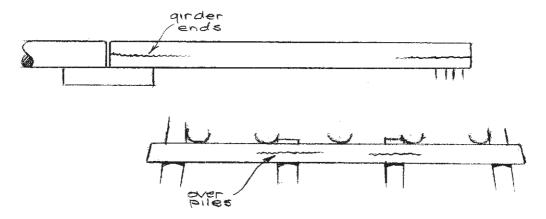
Figure 4.2(b) - Expected Shear Failure Locations
