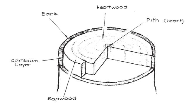
Figure 4.1(b) - Section - Tree Trunk
