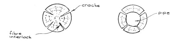
Figure 4.2(c) - Cracked Girder Sections
