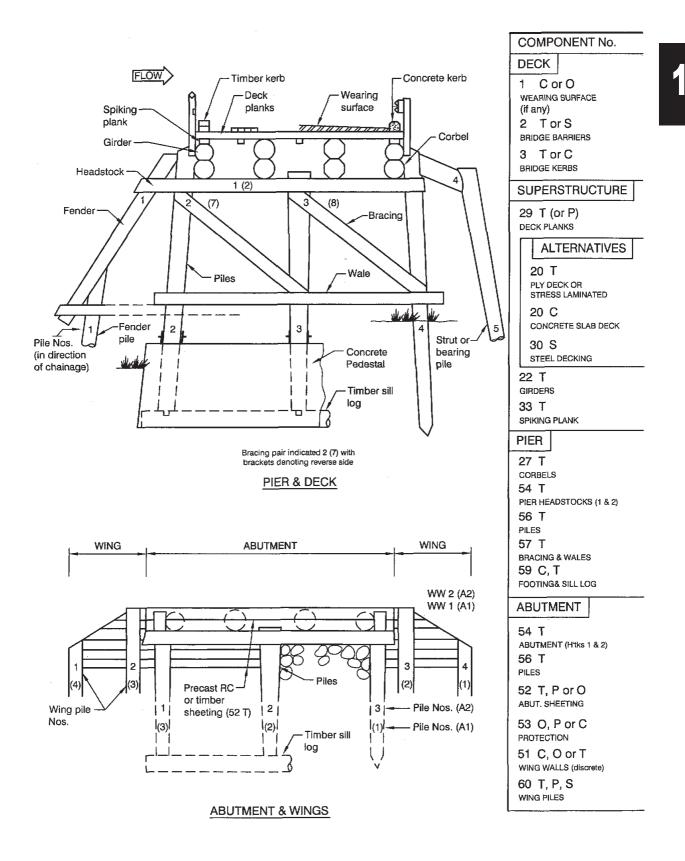
Figure 3.5(b)- Typical Timber Bridge
