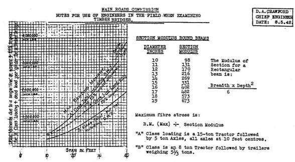
The above moments are those due to one line of wheels, and assume that the moments in the girders do not exceed those caused by one such line. Actually, if the decking is sound and well fitting, the moments on the girders may be less than those due to one line of wheels. It is possible however, in a wide bridge with few girders, for moments to occur in a girder <u>exceeding</u> those due to one line of wheels, for example, a 3-girder bridge more than 15' wide.
