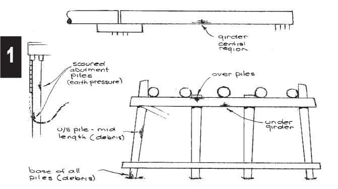
Figure 4.2(a) - Expected Bending Failure Locations
