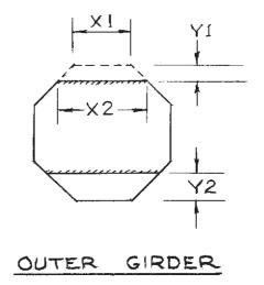
notch to this line causes 25% loss of section
