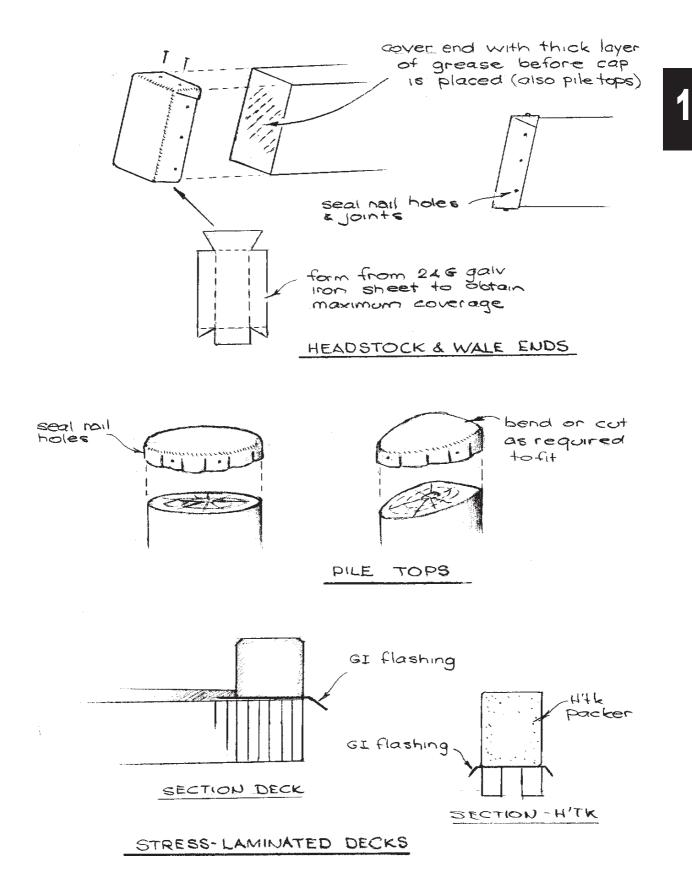
Figure 7.7(b) - Flashing
