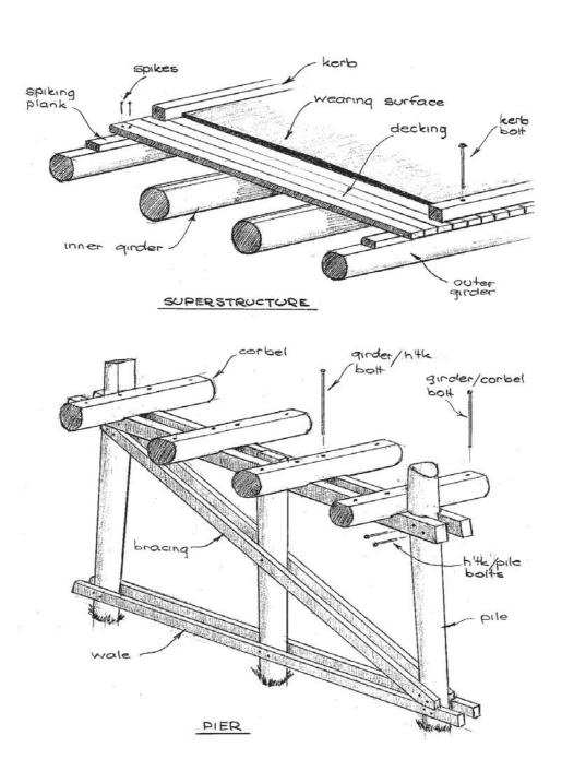
Figure 3.3(b) - Timber Bridge Details
