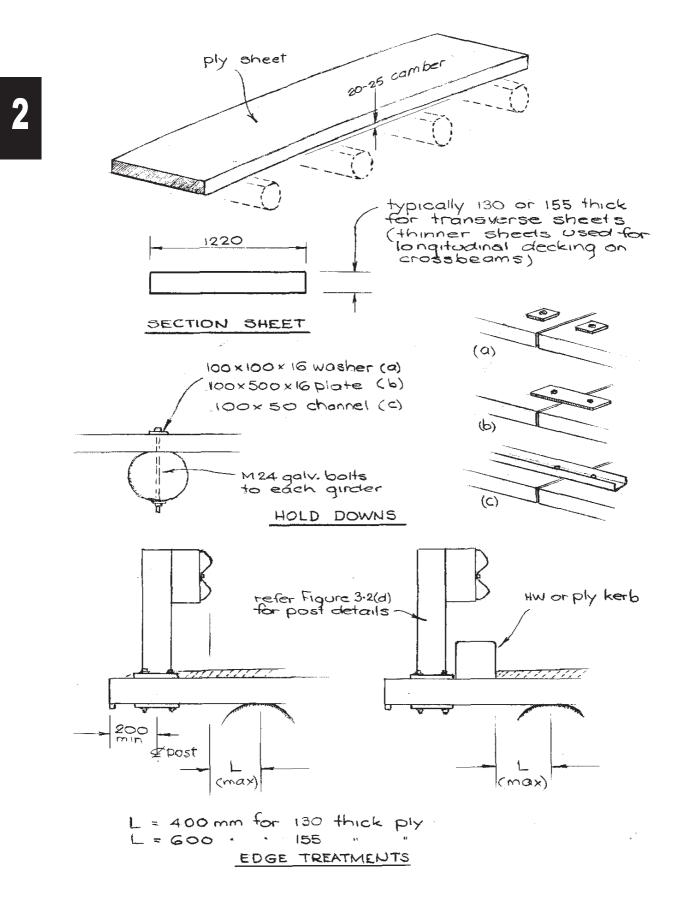
Figure 5.2(a) - Plywood Decking
