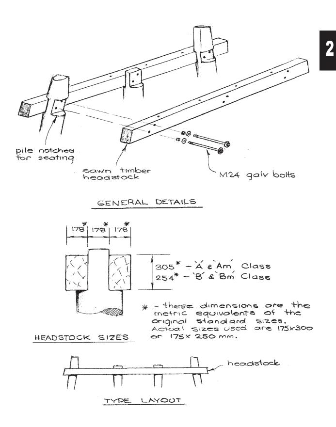
Figure 10.1 (a) - Timber Headstocks - Open Type
