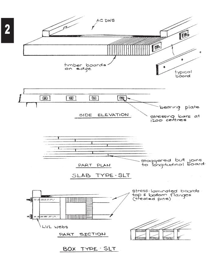
Figure 5.9(a) - Stress-laminated Timber Deck
