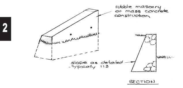
Figure 16.3 - Concrete / Masonry Wing
