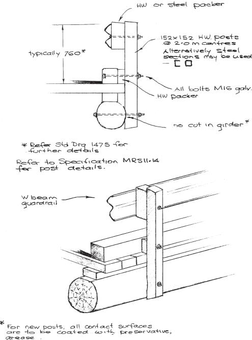
Figure 3.2(a) - Steel Guardrail Barrier
