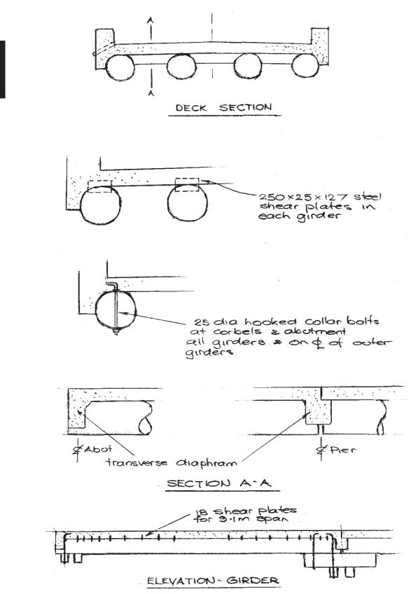
Figure 5.3(b) - Concrete Slab Deck - Type 2
