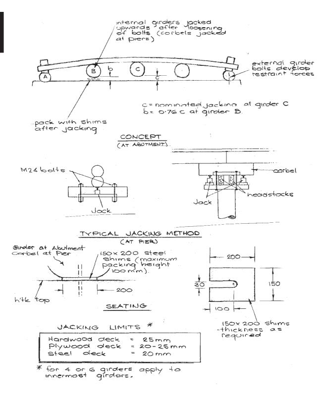
Figure 17.9 - Deck Recambering
