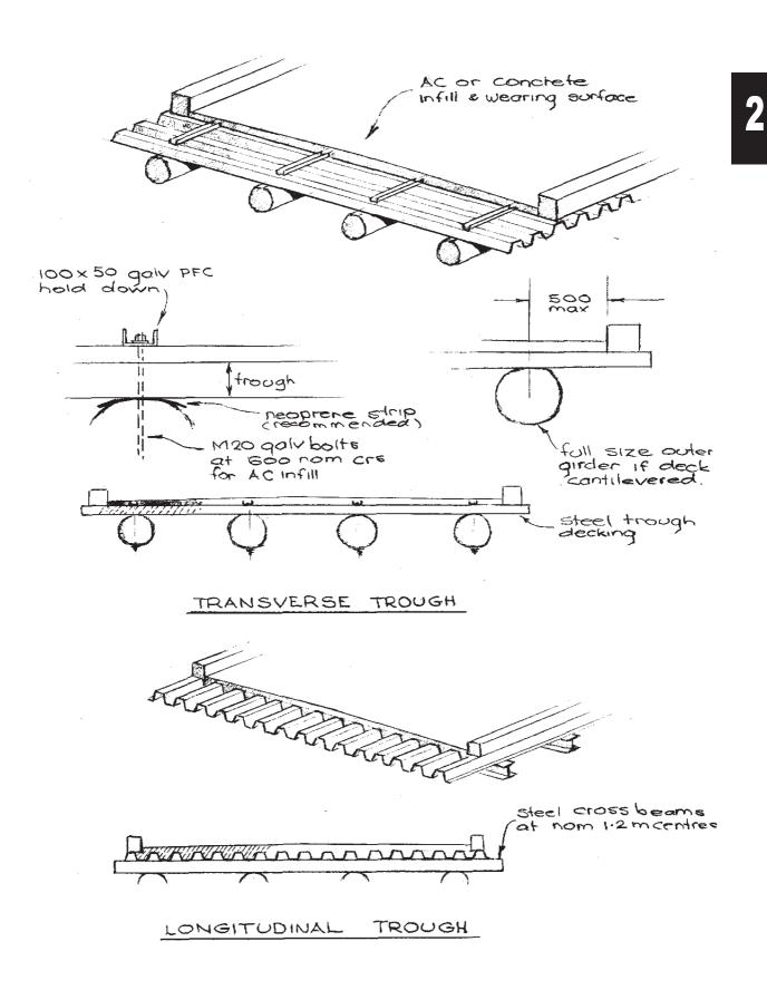
Figure 5.5(a) - Steel Trough Decking
