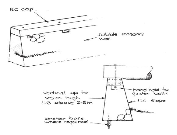
Figure 14.2 - Masonry Abutment
