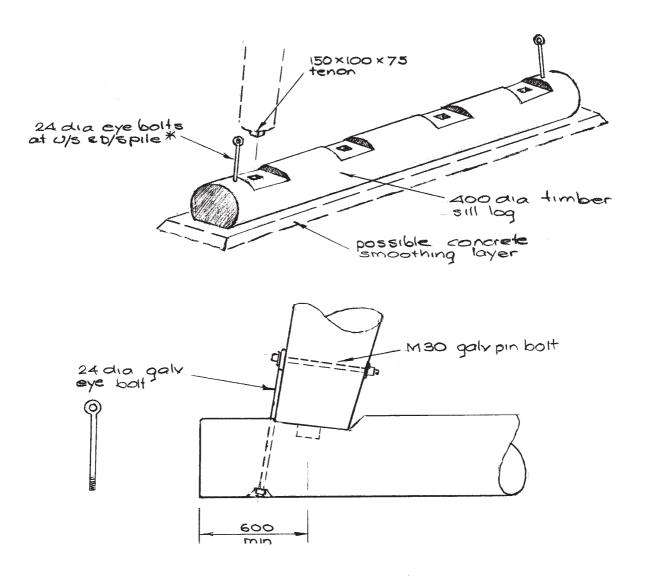
\* Note: additional hold downs from sill to foundations may be incorporated in high flood load situations.
