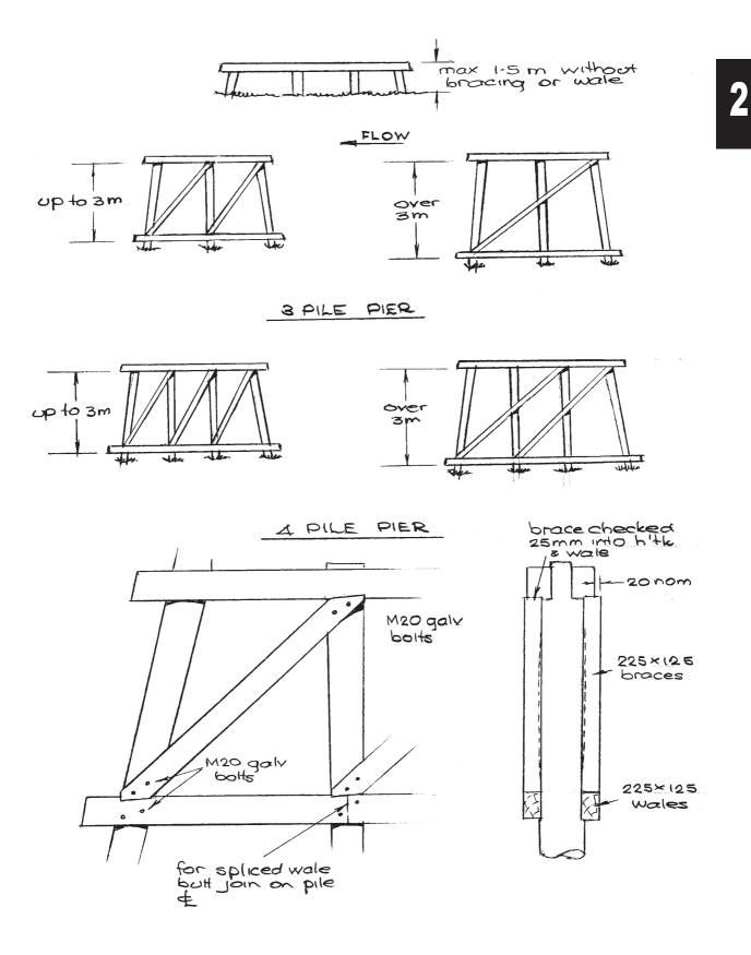
Figure 12.1 - Timber Bracing & Wales
