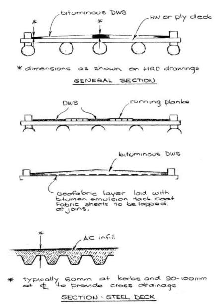
Figure 2.1 - Bituminous Wearing Surface
