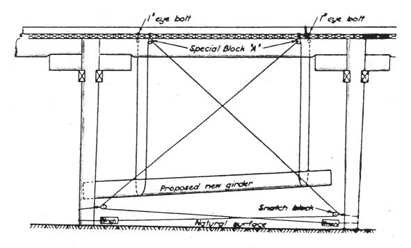
SHOWING METHOD OF LIFTING GIRDER
