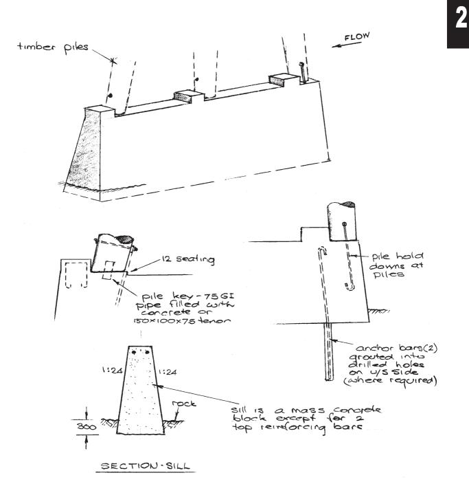
Figure 13.2 - Concrete Sill
