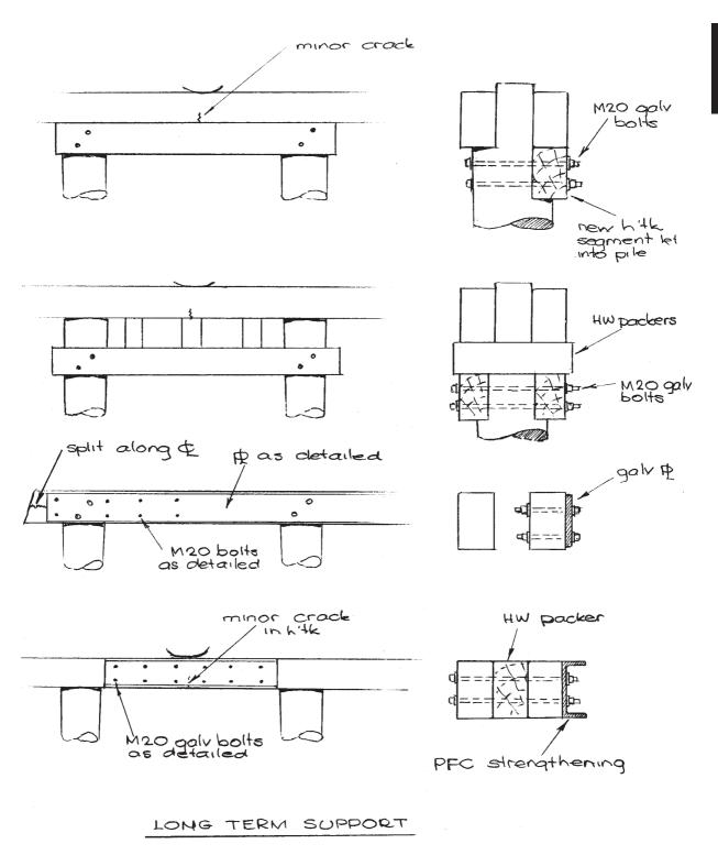
Figure 10.1(d) Headstocks - Supplementary Supports
