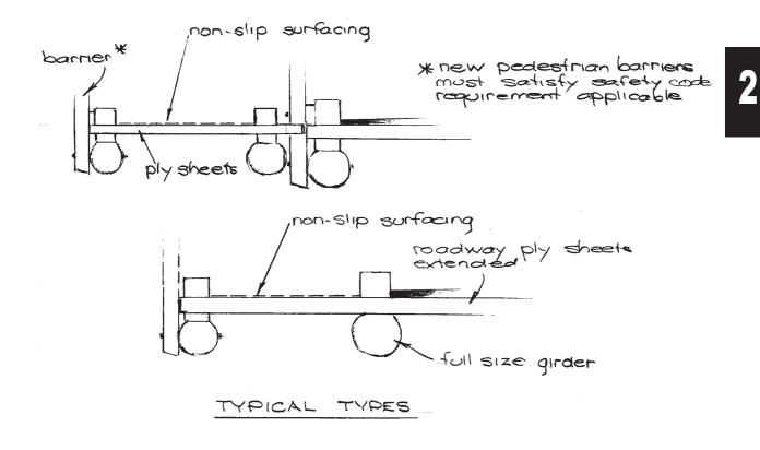
Figure 6.2 - Plywood Footpath
