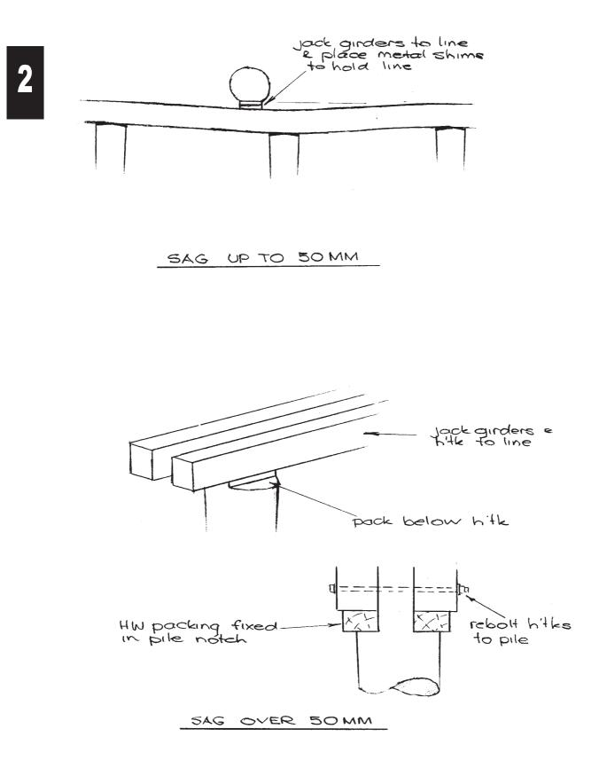
Figure 10.1(e) - Restoring Headstock Levels
