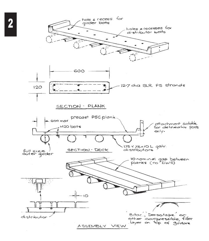
Figure 5.4 - PSC Plank Decking
