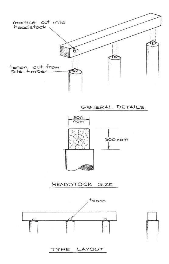
Figure 10.1(b) - Timber Headstock - Solid Type
