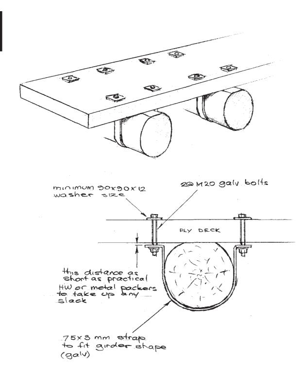
Figure 5.2(c) - Plywood Details 2
