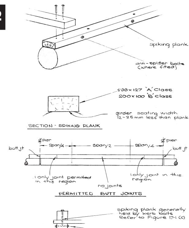
anti-splitter bolts (where fitted) - tefer to Figure 17.1(c)
