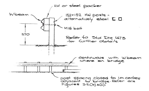
Figure 3.4 - Approach Guardrail
