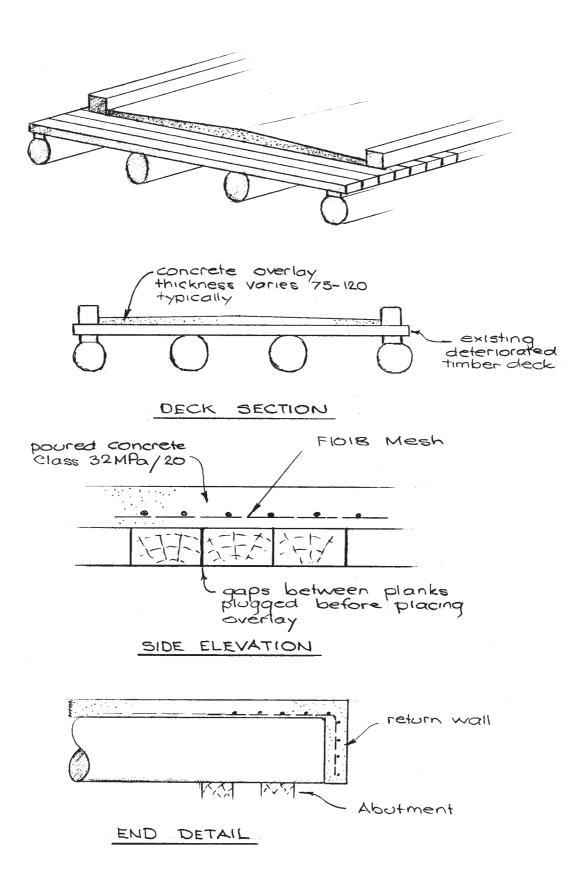
Figure 5.8 - Concrete Overlay
