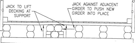
Figure 8.1(j) - Girder Erection 2
