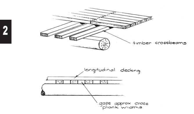
Figure 5.6 - Timber Crossbeams
