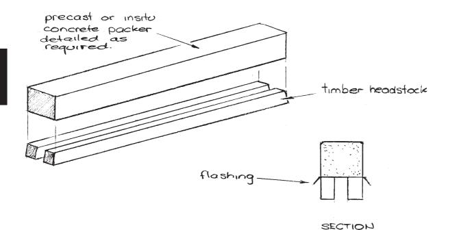
Figure 10.4 - Concrete Packers
