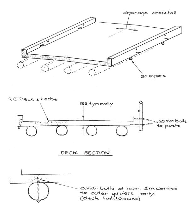
Figure 5.3(a) - Concrete Slab Deck - Type 1
