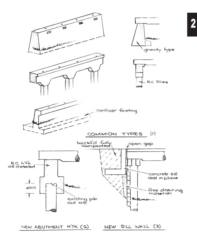
Figure 14.1 - Concrete Abutment
