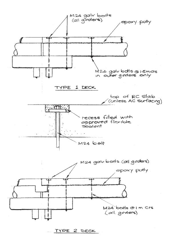
Figure 8.1(k) - Girders - RC Deck
