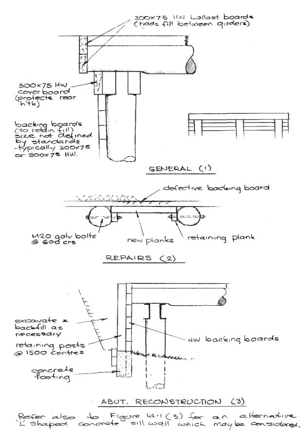
Figure 15.1 - Timber Backing Boards
