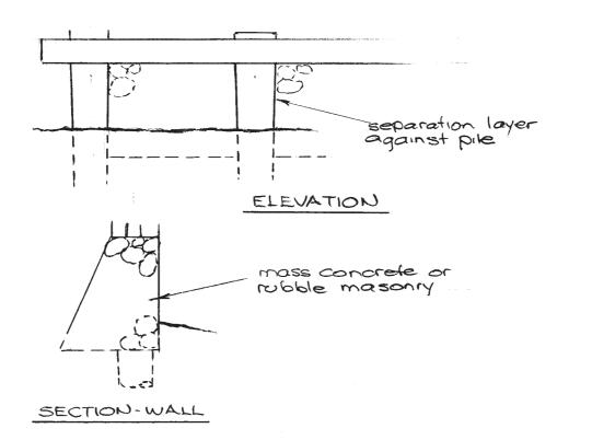
Figure 15.3 - Concrete / Masonry infill walls
