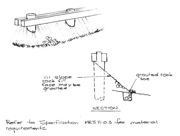
Figure 15.4 - Rock Fill Protection
