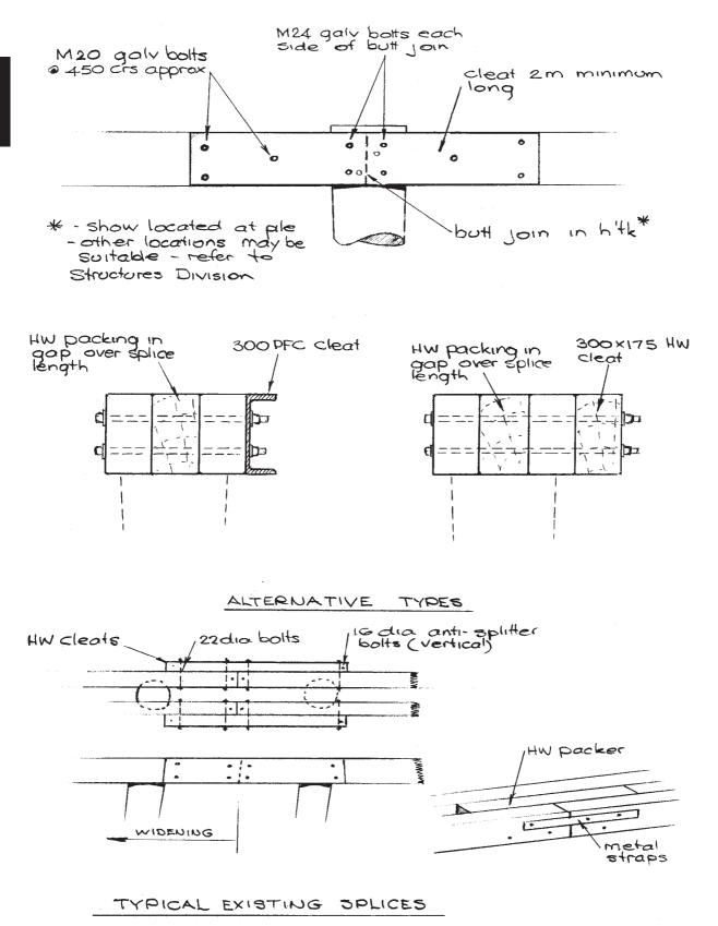
Figure 10.1(c) - Headstock Splicing
