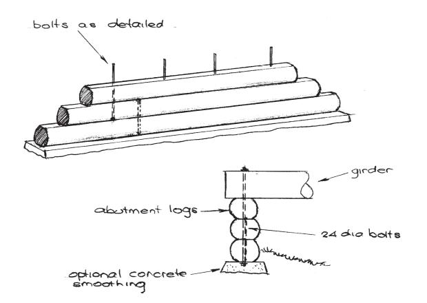
Figure 15.6 - Timber Sill Abutment
