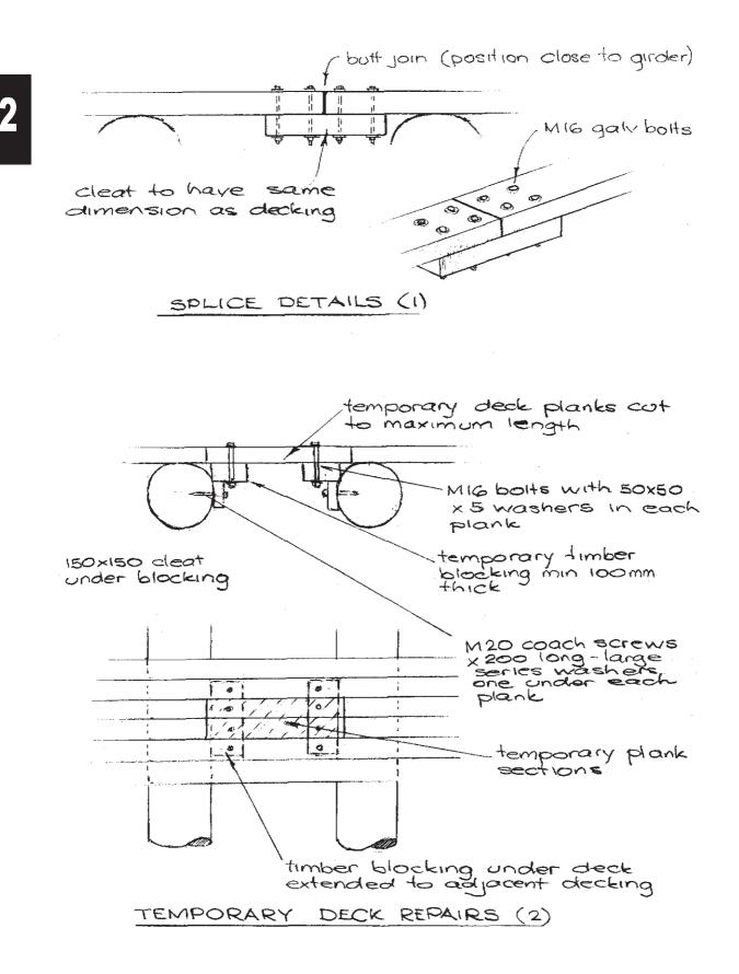
Figure 5.1(c) - Deck Repairs
