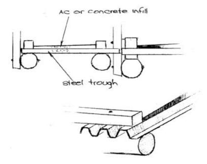
Figure 6.3 - Steel Trough Footpath
