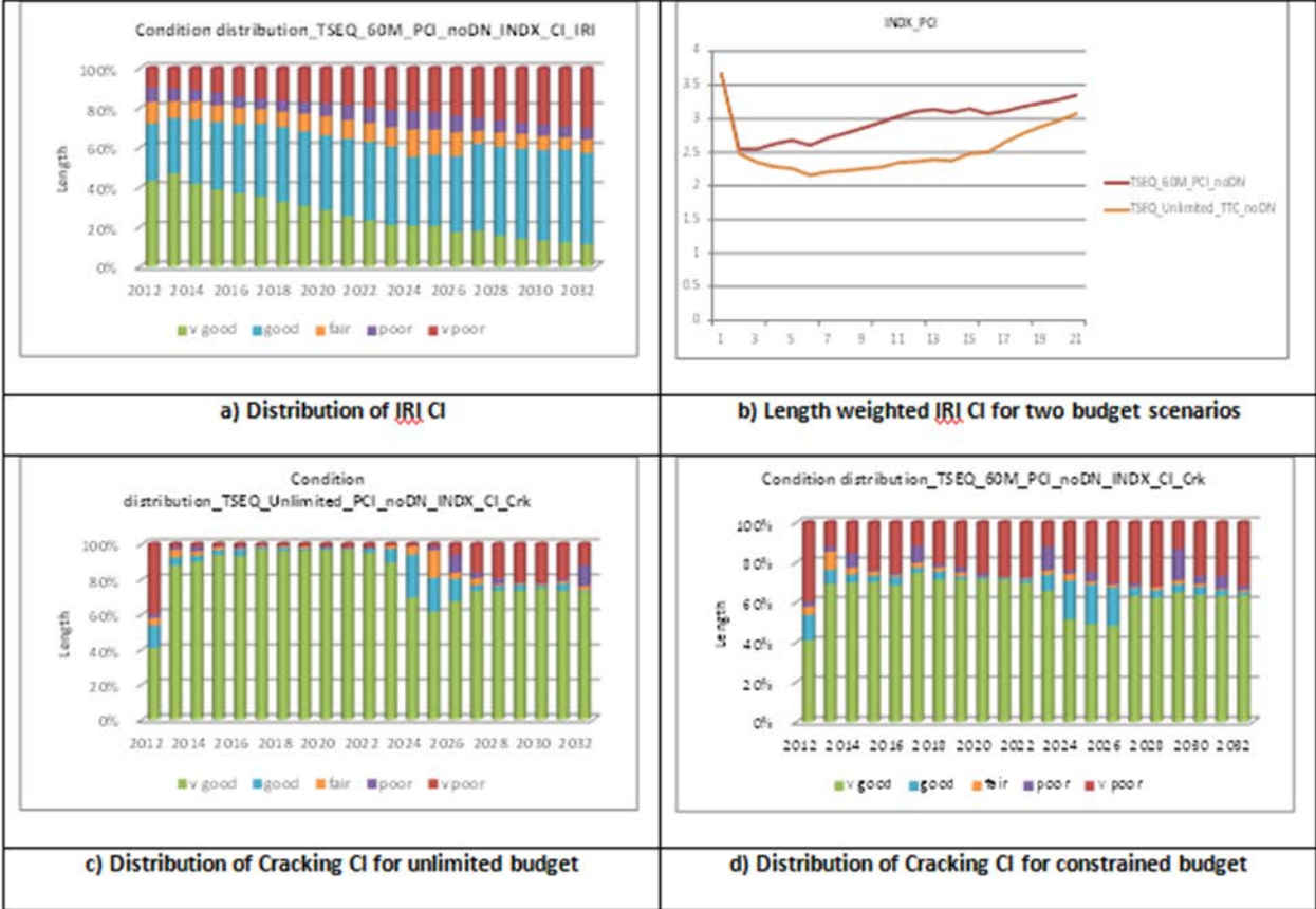
Figure 4: Example outputs showing predicted network condition
