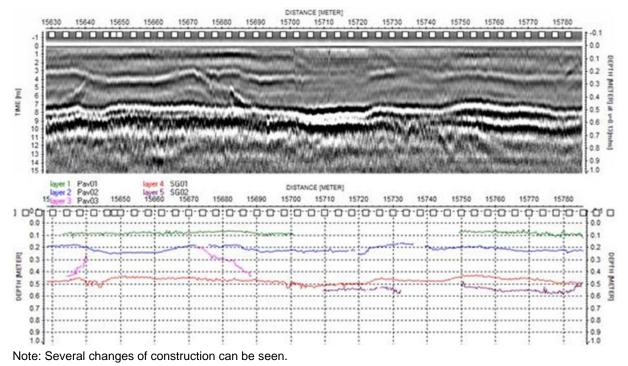
Figure 2.8.4(b) – Example of three-dimensional radargrams of a road pavement
