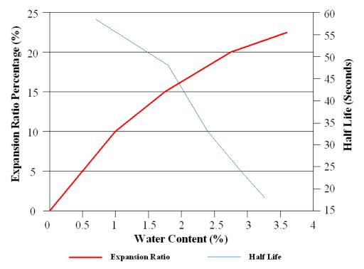
Figure 4.9.8.4.4 – Example of influence of water content on bitumen foaming properties
