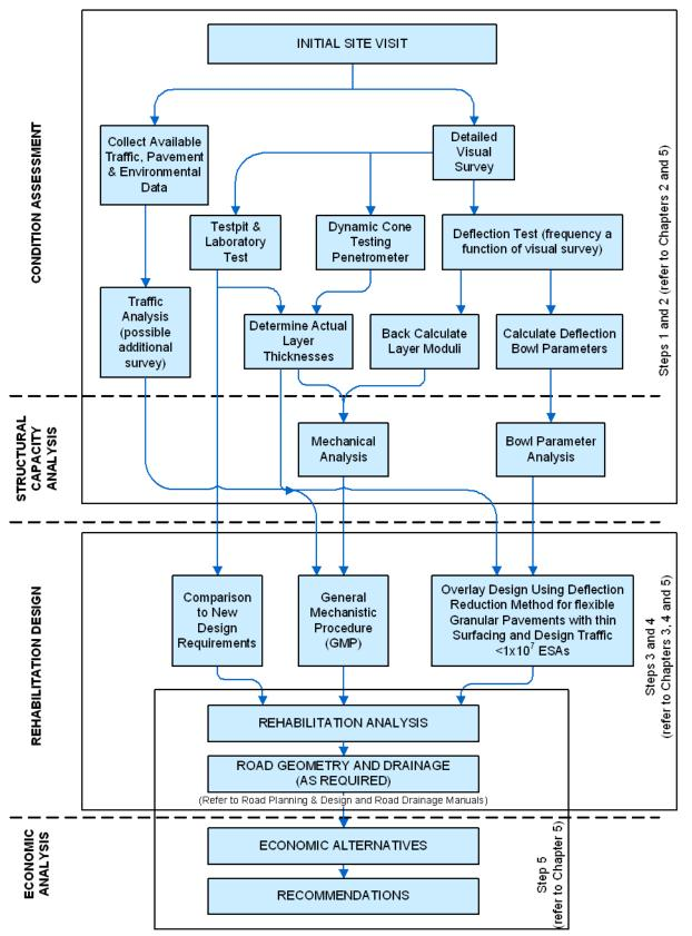
Figure 4.2 – Typical pavement rehabilitation process
