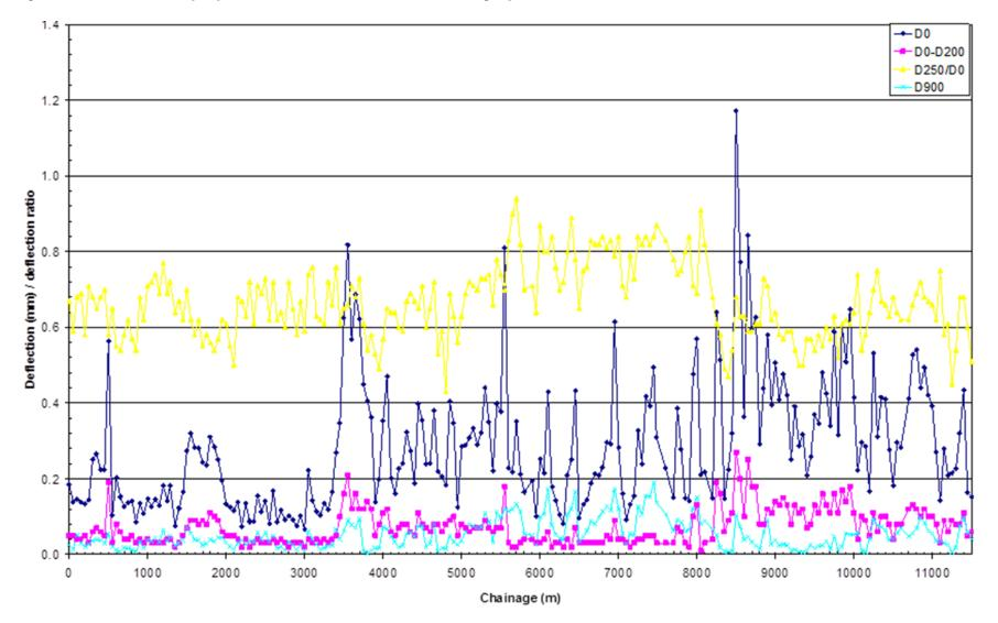
Figure 2.13.10.4.2 – Example plot of deflection results from a non-rigid pavement
