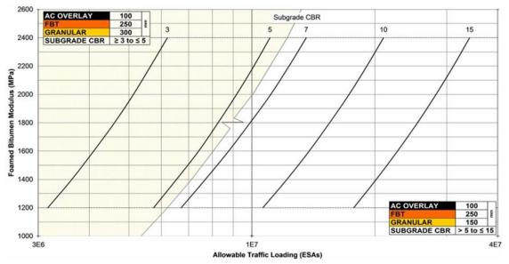
Figure C10(b) – South-east Queensland 100mm asphaltic concrete 300mm foamed bitumen treated material allowable traffic loading
