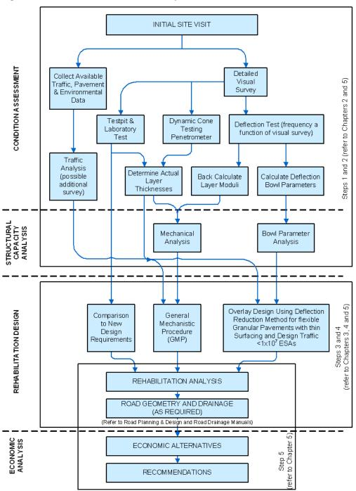
Figure 1.12 – Pavement rehabilitation system
