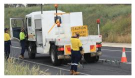
Figure 2.13.10.1(b) – An example of a deflectograph
