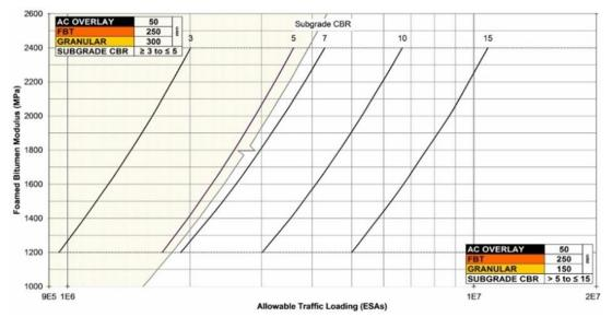
Figure C6(a) – Far north Queensland 50mm asphaltic concrete 250mm foamed bitumen treated material allowable traffic loading
