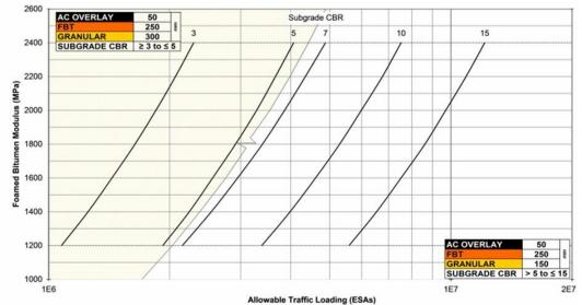
Figure C9(b) – South-east Queensland 50mm asphaltic concrete 300mm foamed bitumen treated material allowable traffic loading
