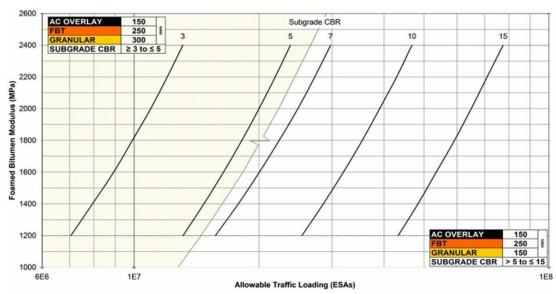
Figure C8(a) – Far north Queensland 150mm asphaltic concrete 250mm foamed bitumen treated material allowable traffic loading
