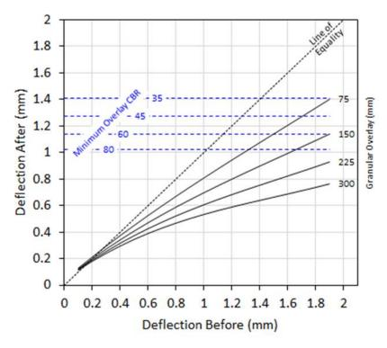
Figure C1.2(b) – Granular overlay design chart where all overlay material complies with MRS05 and MRTS05 and has a minimum California Bearing Ratio as indicated (subgrade CBR 15)
