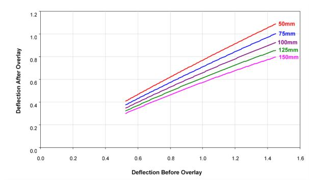
Figure C1.3(e) – Asphalt overlay deflection reduction design chart for weighted mean annual average pavement temperature Zone 3 and a heavy vehicle operating speed of 50 km/h
