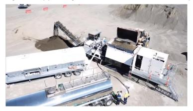
Figure 4.9.9(a) – Wirtgen KMA 220 exsitu foamed bitumen plant
