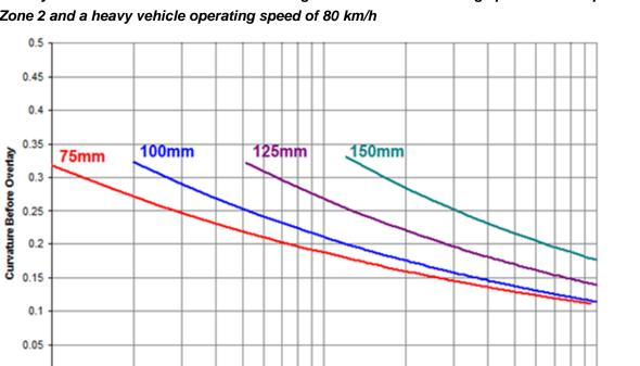
Figure C1.5(g) – Asphalt overlay curvature versus design traffic loading design chart for overlay thicknesses from 75–150mm for weighted mean annual average pavement temperature Zone 2 and a heavy vehicle operating speed of 80 km/h
