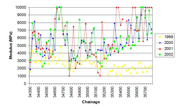
Figure 4.9.8.4.6(c) – Example of increase in back-calculated moduli of a foamed bitumen stabilised pavement
