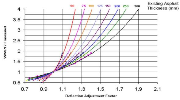
Figure 2.13.10.4.9.1(c) – Temperature correction for Benkelman Beam, deflectograph and normalised 40 kN falling weight deflectometer curvatures for a pavement with a thin asphalt surfacing or seal
