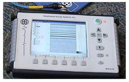
Figure 2.8.3(a) – Example of a single-channel portable ground penetrating radar control unit
