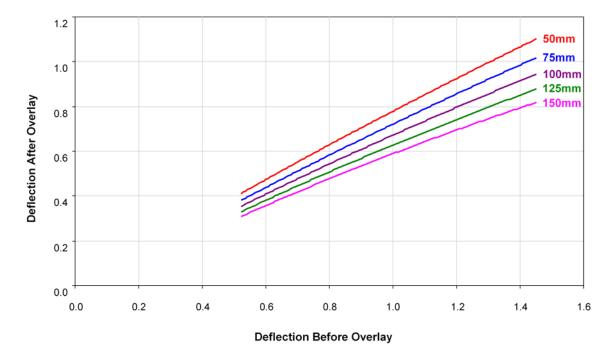
Figure C1.3(c) – Asphalt overlay deflection reduction design chart for weighted mean annual average pavement temperature Zone 2 and a heavy vehicle operating speed of 50 km/h
