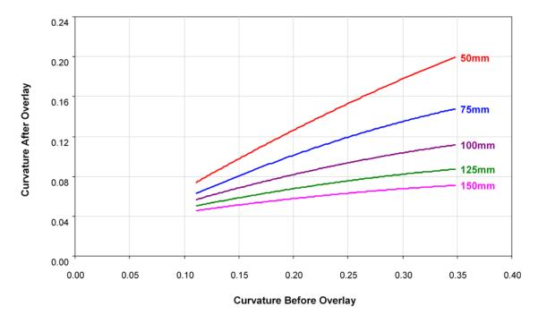
Figure C1.4(c) – Asphalt overlay curvature reduction design chart for weighted mean annual average pavement temperature Zone 2 and a heavy vehicle operating speed of 50 km/h
