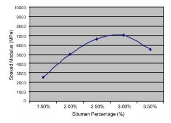
*Figure 4.9.8.5.1 – Example of influence of bitumen content on 'soaked' cured MATerials Testing Apparatus modulus*
