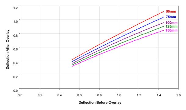
Figure C1.3(b) – Asphalt overlay deflection reduction design chart for weighted mean annual average pavement temperature Zone 1 and a heavy vehicle operating speed of 80 km/h
