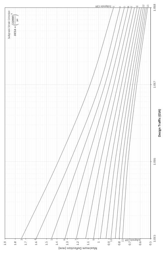
Figure C1.1(b) – Tolerable deflection for second design standard for falling weight deflector and Benkelman Beam with 40 kN loading
