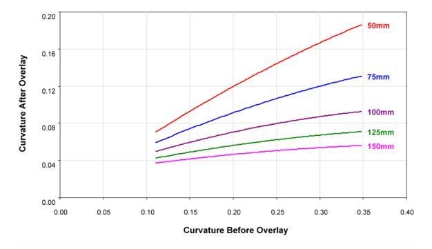
Figure C1.4(g) – Asphalt overlay curvature reduction design chart for weighted mean annual average pavement temperature Zone 4 and a heavy vehicle operating speed of 50 km/h
