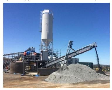
Figure 4.9.9(b) – Ammann exsitu foamed bitumen plant
