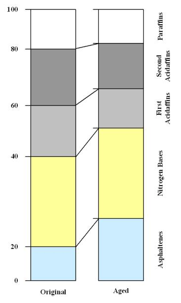
Figure 4.4.3.5 – Relative compositions of original and aged bitumen (not to scale)
