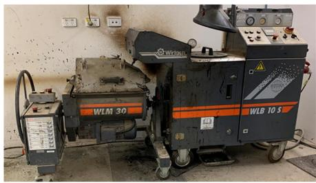
Figure 4.9.8.4.2(a) – Laboratory foaming process
