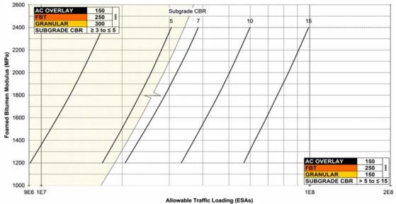
Figure C11(b) – South-east Queensland 150mm asphaltic concrete 300mm foamed bitumen treated material allowable traffic loading
