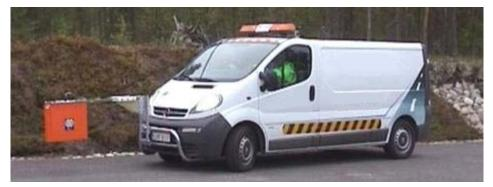
Most commercial GPR units are of the 'impulse' type (the GPR emits discrete bursts of energy into the pavement and measures the response after each).
