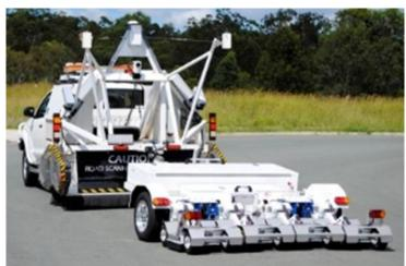
Figure 2.8.3(c) – Example of an air-coupled antenna mounted on the front of a vehicle
