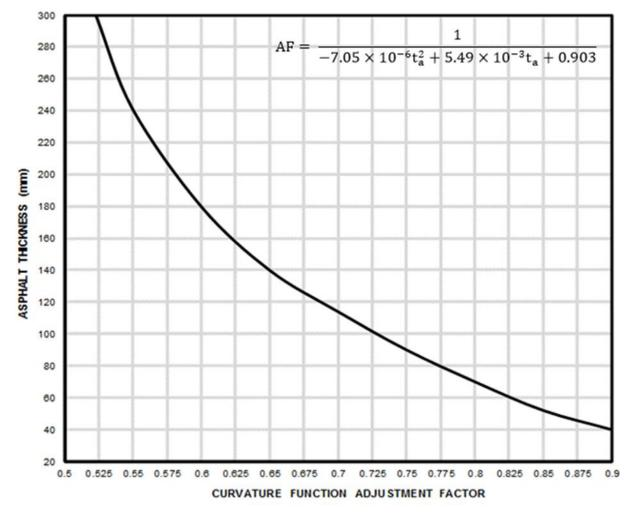
Figure 2.13.10.4.9.2(b) – Speed correction of curvature for Benkelman Beam and deflectograph results derived for a pavement with a thin asphalt surfacing or seal
