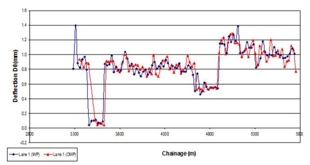
Figure 5.3.2.2 – An example of a  $D_0$  deflection profile with representative sections shown
