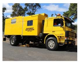
Figure 2.13.10.1(c) – An example of a falling weight deflectometer
