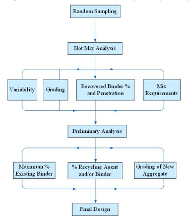
Figure 4.4.14.4.1 – Flow chart for hot in-place asphalt recycling mix design
