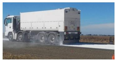
Figure 4.9.8.6.1(f) – Spreadrate test in operation
