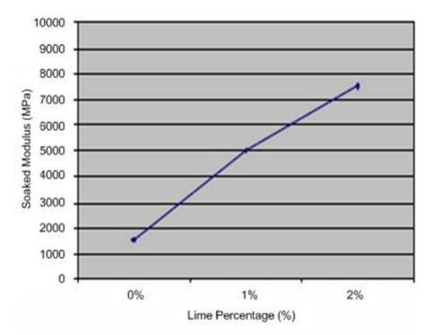
Figure 4.9.8.4.5 – Influence of lime on MATerial Testing Apparatus test results
