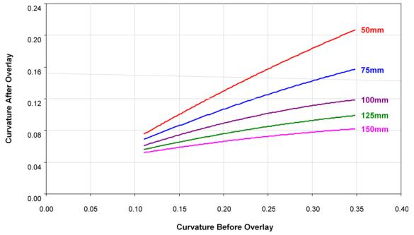
Figure C1.4(b) – Asphalt overlay curvature reduction design chart for weighted mean annual average pavement temperature Zone 1 and a heavy vehicle operating speed of 80 km/h
