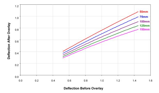
Figure C1.3(g) – Asphalt overlay deflection reduction design chart for weighted mean annual average pavement temperature Zone 4 and a heavy vehicle operating speed of 50 km/h
