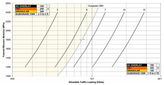
Figure C7(b) – Far north Queensland 100mm asphaltic concrete 300mm foamed bitumen treated material allowable traffic loading
