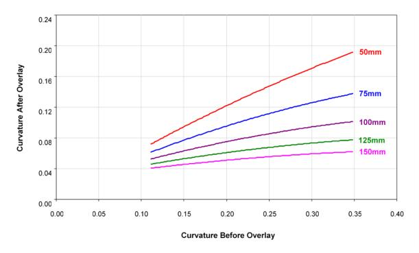
Figure C1.4(e) – Asphalt overlay curvature reduction design chart for weighted mean annual average pavement temperature Zone 3 and a heavy vehicle operating speed of 50 km/h
