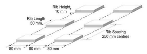
Figure 7.7.3(c) – Height measurement of the raised rib
