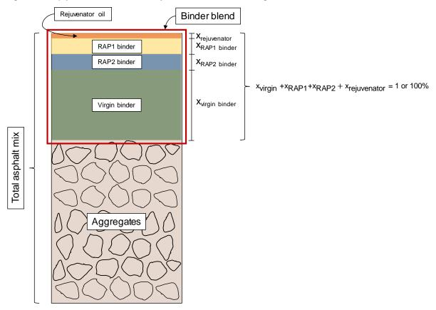
Figure 4.3.2(b) – Binder blend components schematic diagram
