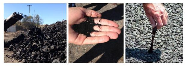
CRM binder is used extensively in sprayed sealing, with <u>MRTS11 Sprayed Bituminous Surfacing</u> (<u>Excluding Emulsion</u>) being updated to permit Contractors to substitute a CRM binder in many cases where a conventional polymer modified binder (PMB) is specified. CRM sealing binders can be either field or factory blended products and usually contain approximately 15% crumb rubber.
