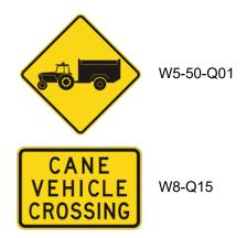
The Cane Vehicle Crossing (W5-50-Q01), CANE VEHICLE CROSSING (W8-Q15) signs may be used at locations where cane vehicles cross the roadway. Where cane vehicles are likely to cross multiple locations along a road, or travel along a road, see item (b).
