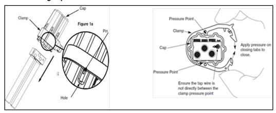
**INSTALL CAP** – Install cap by holding all wires and pushing the cap over the connection assembly until it goes no further.
