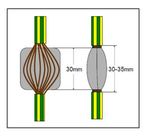
**REMOVE INSULATION** – 400 mm from the end of the cable, remove a 40 mm of green / yellow insulation exposing a 30–35 mm section of copper strands.
