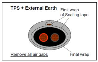
PLACE CABLES - Place the sealed sections of the earth and power cables together and press.
