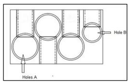
**SELECT HOLE** – Select hole in connector to suit cable size.
