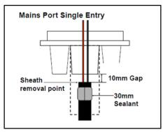
**APPLY TAPE** – Apply sealant tape to outer insulation.
