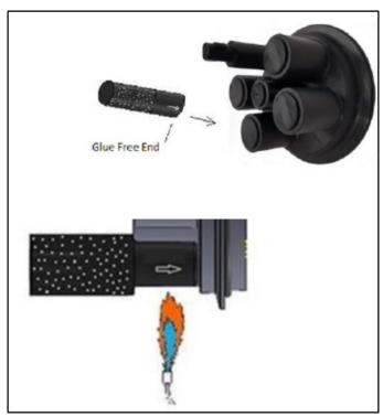
**SLEEVE** – Slide the glue-free end of the heat-shrink sleeve onto the prepared port.
