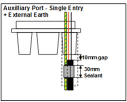
**COMBINE CABLES** – The external earth cable must be installed along with a TPS cable.
