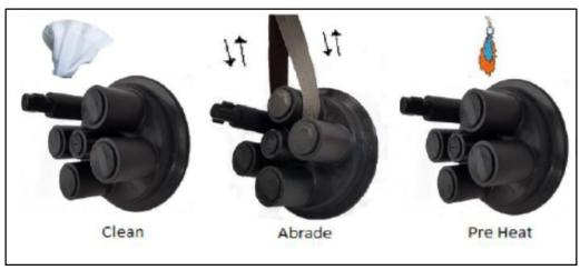
**CLEAN** – Knock out enclosure ports as required and wipe ports with a clean cloth.
