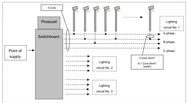
Figure 6.2.2 – Road light configuration example
