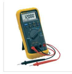
A dual impedance digital multimeter is recommended to confirm if any inducted voltages are present in high impedance CCTS that are de energised.
