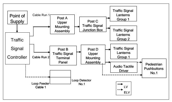
Figure 6.2.1 – Traffic signal configuration example
