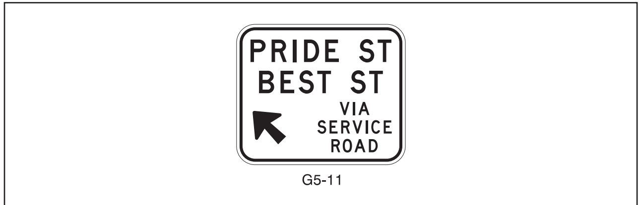
Figure 2.14 SIGNS FOR SERVICE ROAD OPENINGS
