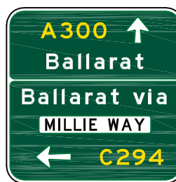
(b) On a narrow format list type ADS, e.g. Sign No. G1-6
