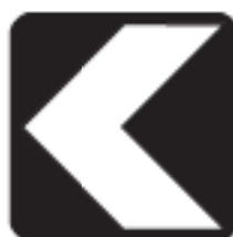
Unidirectional Hazard Marker
