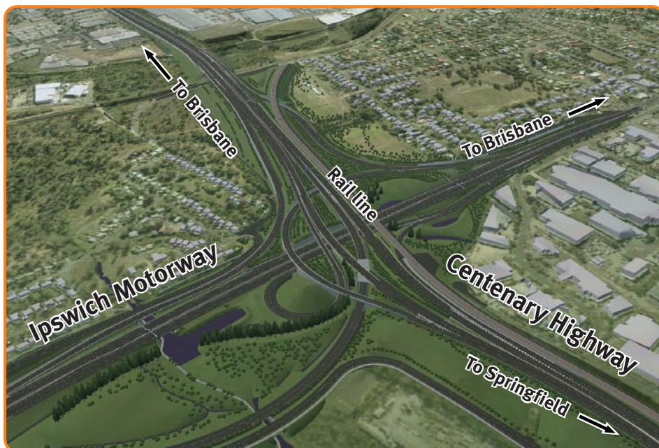
Multi-level system interchange: an artist's impression of the new Centenary Highway Interchange
