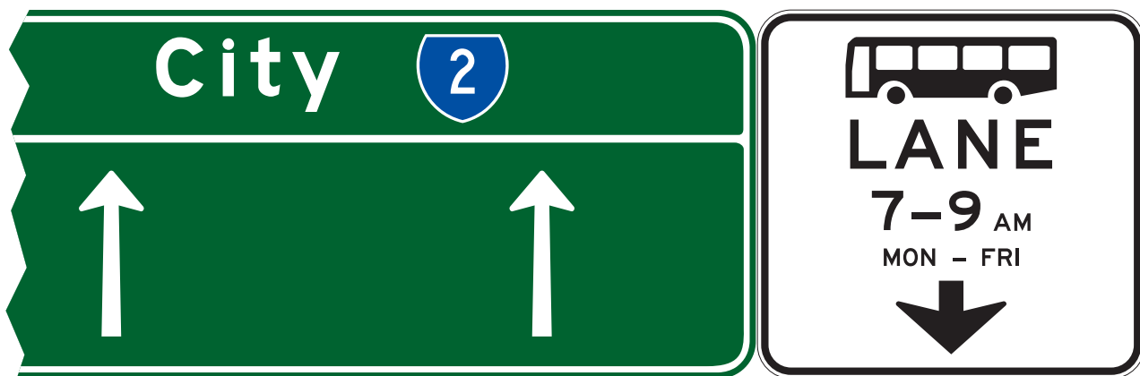
(c) Overhead mounted in conjunction with direction signs with arrows - part-time bus lane
