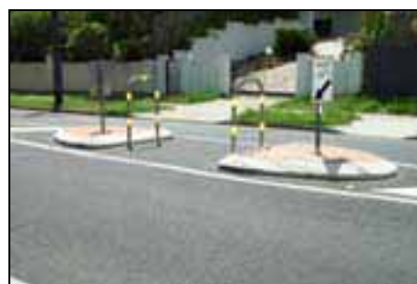
Typical Pedestrian Refuges
