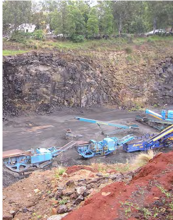
Basalt and igneous rocks comprise the majority of source rocks in the Strategic Quarries and Quarries of Interest. The basalt quarry in the photo is using a mobile 170 tph crushing plant in the pit. Note the soil and overburden in the foreground and the different (dark and light) basalt materials in the rockface indicating variable quality.
