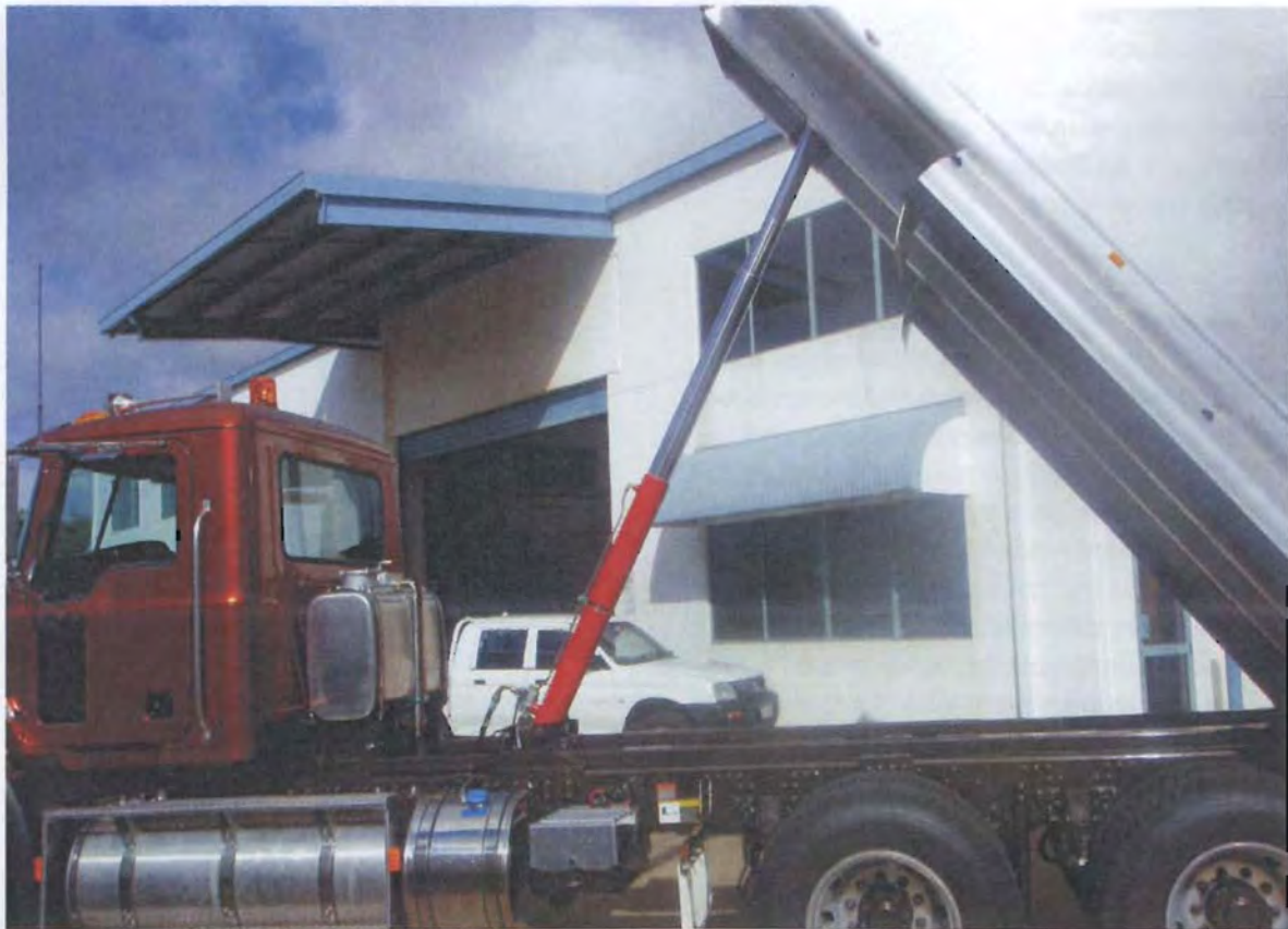
Figure 7. Lower red stage of the hoist is double acting
