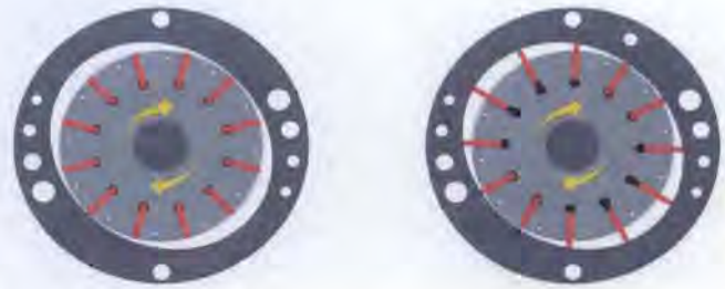
Figure 1. Left – vanes restrained in the standby energy saving position Right – standard vane pump operation position
