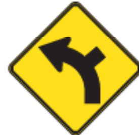
Side Road Junction on a Curve (L or R) (L version illustrated)
