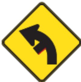
Side Road Junction on a Curve (L or R) (L version illustrated)
