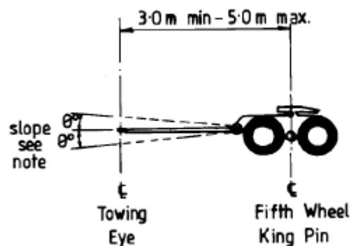
**Note:** Operating angle of drawbar to be within 5 degrees of horizontal when the assembled laden road train is standing on a level surface.
