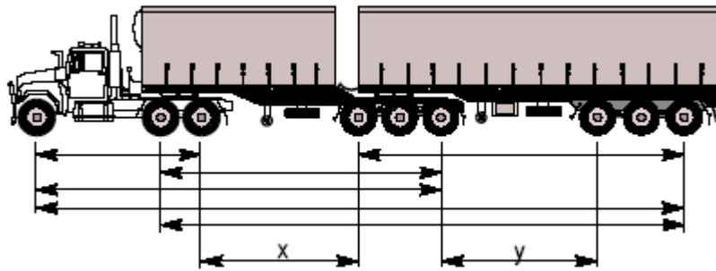
**Figure 2: B-double extreme axle spacing example**
