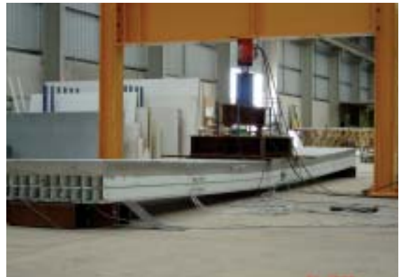
Figure 9 : \frac{2}{3} Scale Bridge Deck Load Testing
