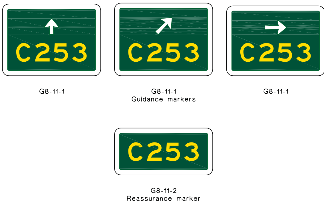
FIGURE 4.3 FREE STANDING GUIDANCE AND REASSURANCE MARKERS
