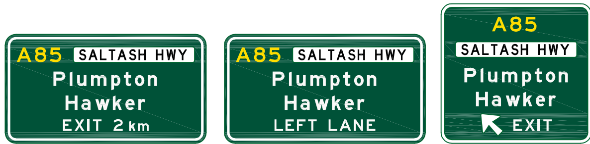
(a) Advanced exit and exit direction signs—expressway type roads
