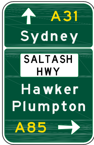
(a) Advance direction sign
