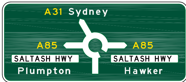
(f) On a G1-5 type diagrammatic ADS
