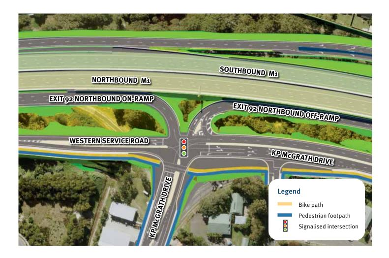
The new service road will continue south from Nineteenth Avenue and connect into a new signalised intersection joining KP McGrath Drive and the northbound on and off-ramps.
