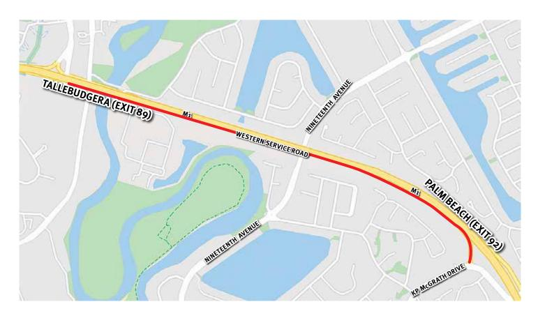
The upgrade will include constructing a new western service road, with one lane in each direction, between Tallebudgera (Exit 89) and Palm Beach (Exit 92), including a four-way signalised intersection with Nineteenth Avenue.
