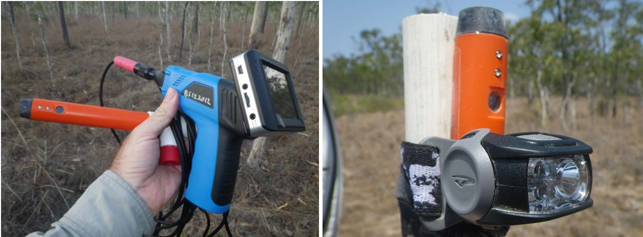
Figure 3 Modified Burrow Scope for Inspecting Tree Hollows
