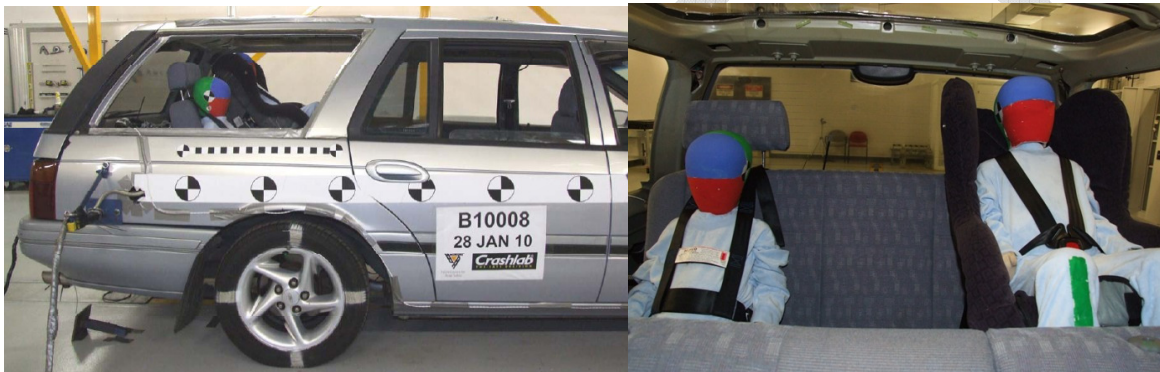
Figure B1. Test configuration for the frontal barrier test
