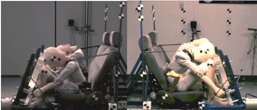
Figure B7. Typical crash test done under previous version of VSB 05. Note the dummies' head striking the seat in front of them.
