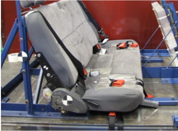
Figure B7. Seat fitted with anti submarining clip; these can be seen at the front and middle of the seat pan.
