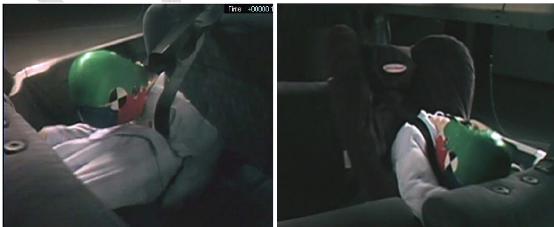
Figure B2. The point of maximum head forward excursion for P3 dummies seated directly on a category 2 seat (left) and on an AFFCR (right).
