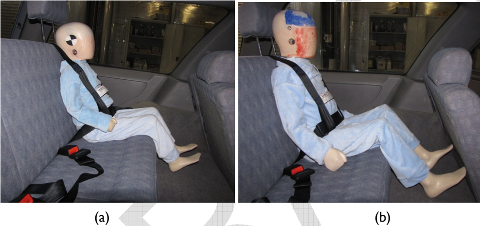
Figure B3. TNO P3 (a) and P6 (b) series dummies fitted to a VSB 05 Category 2 seat
