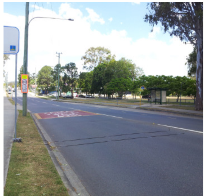
Figure 4.3: Example detection tubes on approach to a school zone
