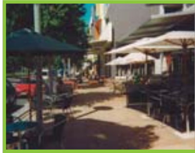
Figure D1-20 Unobstructed access paths are required on footpaths, preferably next to the property boundary (in this case, next to the shopfronts)
