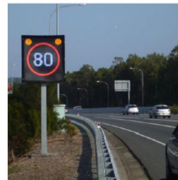
VARIABLE SPEED LIMIT SIGNS (VLS)
