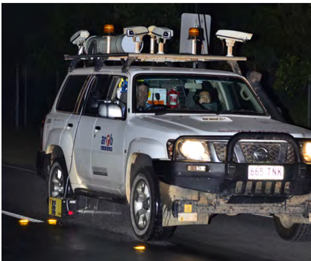
Evaluation vehicle measuring wet weather retro-reflectivity.
