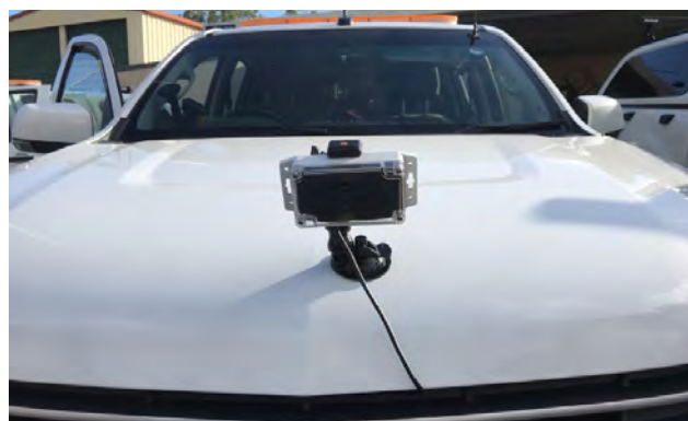
Vehicle-mounted camera capturing any potential defects on the road network as the vehicle drives by.
