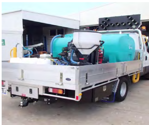
The purpose-built herbicide truck, reducing the risk of moving and mixing chemicals and making it easier for crews to work safely.
