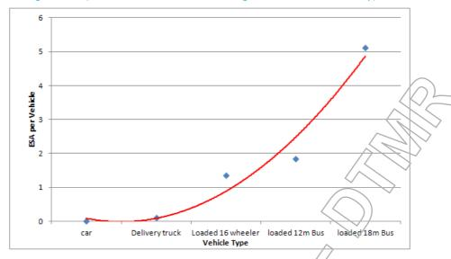
Figure 1: Equivalent Standard Axle Loadings for Different Vehicle Types
