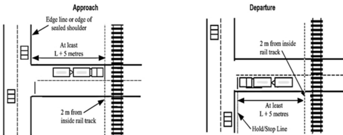
**Figure 4.9(c) – Minimum stacking distance requirement for intersections (Sources: NTC 2007 and AS 1742.7:2016)**
