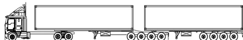
PBS-approved Level 2B B-doubles up to 30 metres overall length have on-road performance that is equivalent or better than conventional 26 metre B-doubles, with the exception of their low speed manoeuvrability and bridge loading impacts. As a result, PBS B-doubles are generally fitted with steerable trailer axles, and bridge capacity limits their gross mass.
