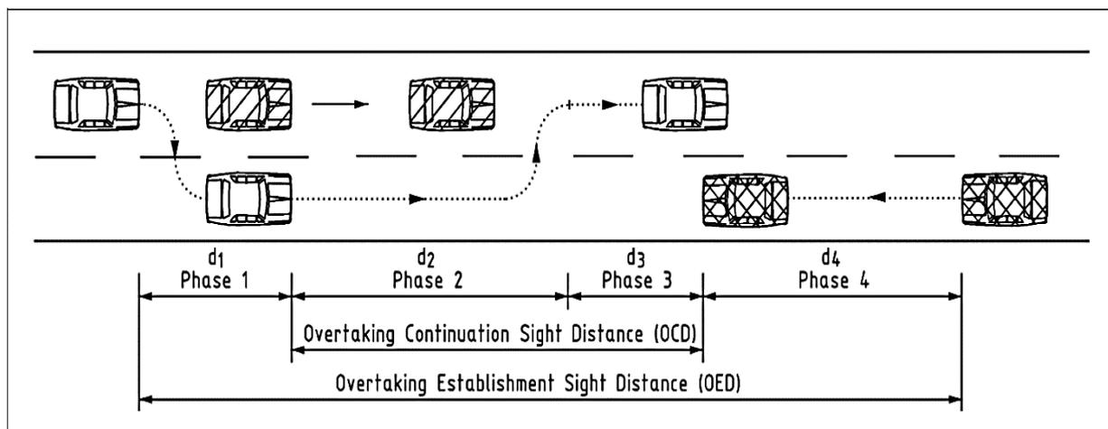
The establishment and continuation sight distances were studied by Transport and Main Roads (SMEC 2015), and the recommended minimum values are shown in Table 4.12(b) and Table 4.12(c) respectively.
