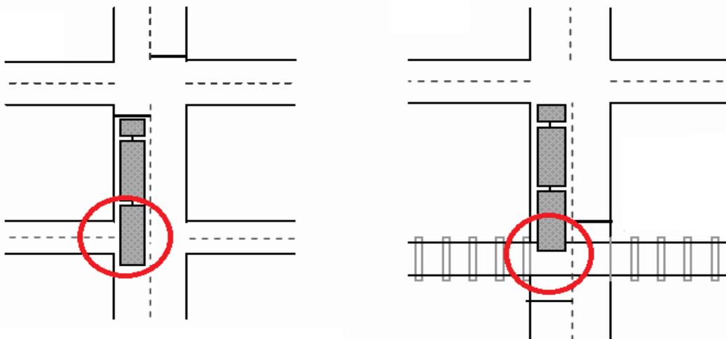
Stacking distance can be readily assessed as part of a desktop study using high-quality satellite imagery. Stacking distance can also be measured in a field test. In both instances, it should be
