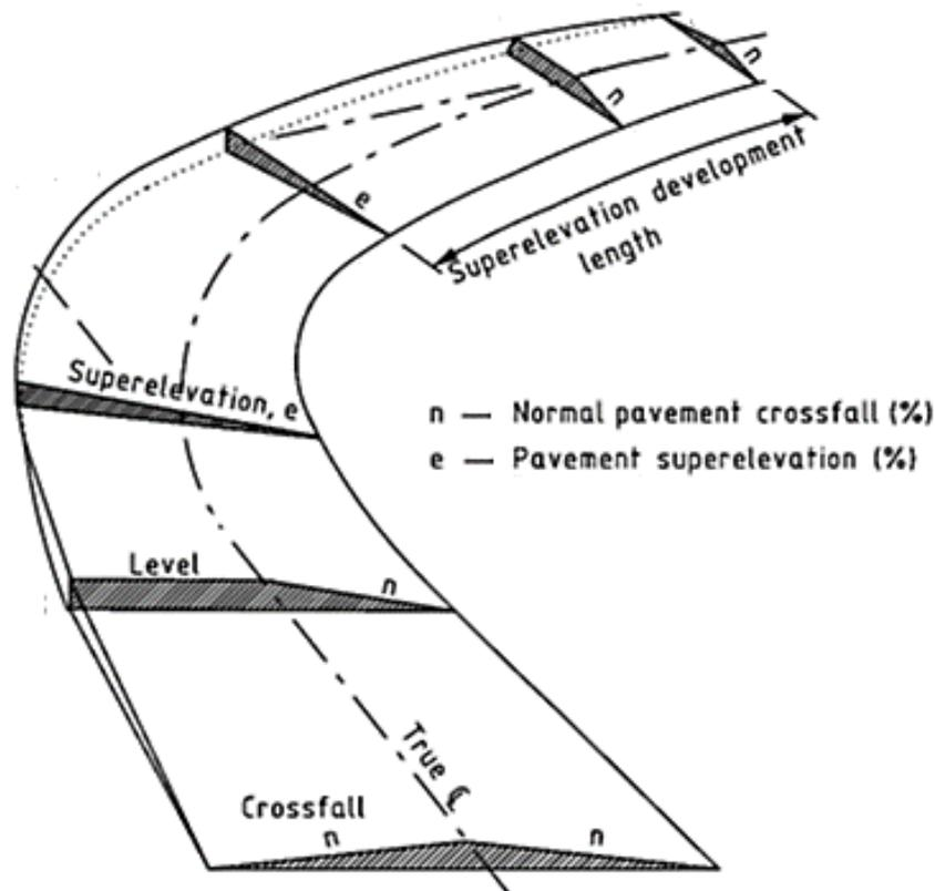
Some road train routes carrying a high proportion of high COG freight (for example, double-deck livestock) may have been constructed with a maximum curve superelevation of 4%, particularly for low speed environments.
