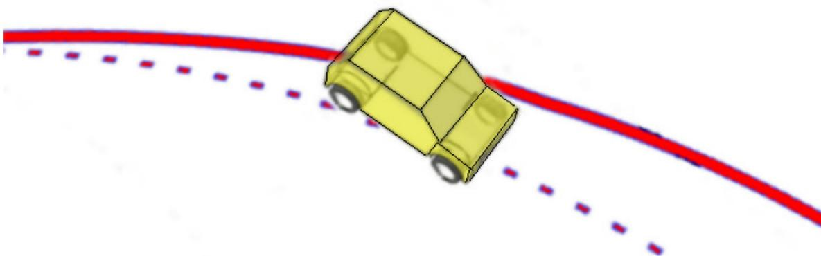
With a combination vehicle in a turning situation (without braking), if the sideways force on the trailer axle(s) exceeds that available from the road/tyre interface the trailer axle(s) tyres will slide outwards (in effect – oversteer) with the likelihood of the trailer leaving the road and in an extreme case come right around and jack knife with the prime mover or another trailer in the case of a B-Double or road train.
