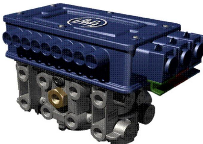
The unit is remotely mounted on the trailer and consists of a multiple port relay valve with internal pressure transducers to measure air tank, airbag and control line pressures. It also contains an internal accelerometer so that it can measure lateral acceleration and the valve is controlled by an internal electronic control unit (ECU) that is programmed to give appropriate braking performance.
