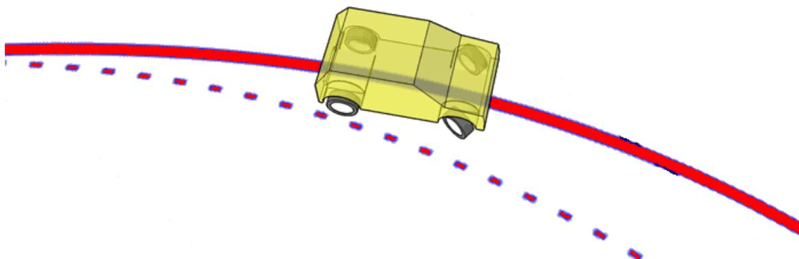
If the sideways force on the drive axle(s) exceeds that available from the road/tyre interface the actual path of the drive axle(s) tyres will be sharper than the steering input and the vehicle will oversteer. That is, the rear of the vehicle will run wide on the curve with the likelihood of the vehicle spinning out.
