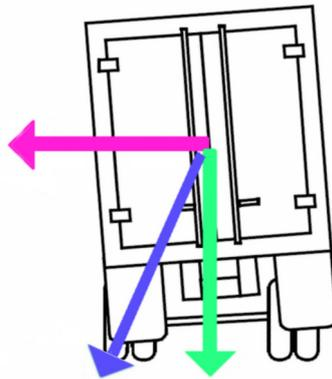
Consequently, if a vehicle is approaching the rollover threshold the risk of overturning can be reduced by reducing the speed or the sharpness of the turn or both. Nothing can be done about the cargo mass.
