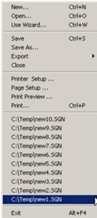
This option is used to select up to 10 previously designed drawings without needing to close a current drawing.
