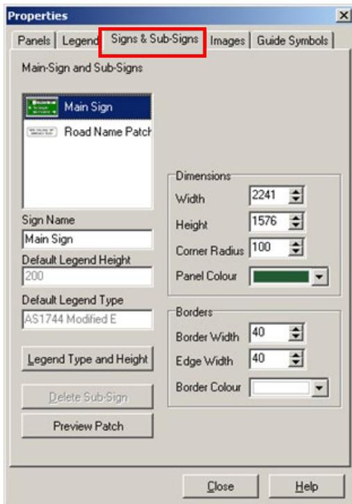
Selecting the main sign or any sub-sign in the list box will indicate all features associated with the makeup of those signs. This will allow control over panel positions, colours and dimensions as well as border widths and colours. It also indicates the default legend types and height of each panel.
