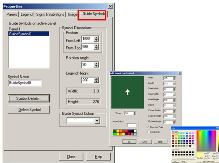
Note: Guide symbol colour options can be increased to full colour palette by selecting **Symbol Details** as shown in Figure 2.7.4.4 and double-clicking on any colour in the **Arrow Colour** box.
