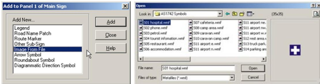
TraSiCAD accesses internal directories of .wmf or .emf symbol files to be directly imported onto the sign face. Selecting **Add: Image From File** will usually directly access the **Symbols** library within the TraSiCAD program. In a typical installation this file location will be C:\Program Files (x86)\TMR\TraSiCAD\Symbols.
