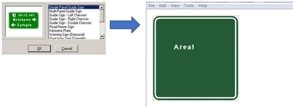
These options are used to develop new signs, using basic styles and backgrounds. There are up to 16 different styles that are selectable from this box.
