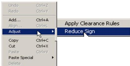
The **Reduce Sign** option completely reduces the sign to its smallest size, taking into consideration and applying clearance rules formulated in the rule sets previously mentioned in Section 2.4.1.1.
