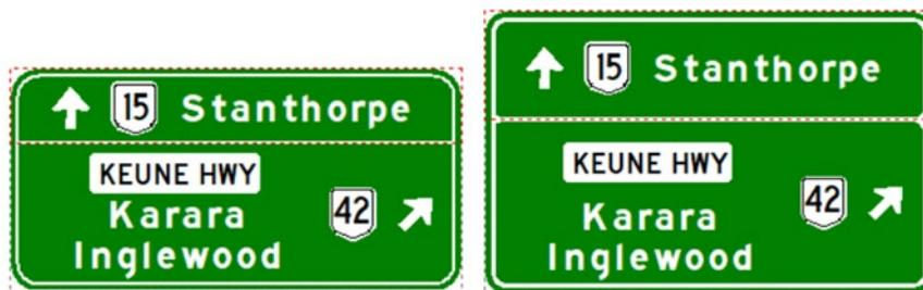
After clearance with AS 1743 Light\_on\_Dark ruleset, borders and external and internal corners are reset.
