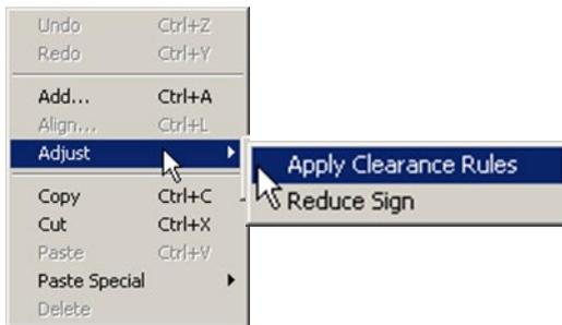
The **Apply Clearance Rules** option enforces an automatic clearance on all items on the drawing to give predetermined spacing from rules installed within TraSiCAD. These rules can be found in the **Rule Editor** in the **Options** directory (see Section 2.4.1.1).
