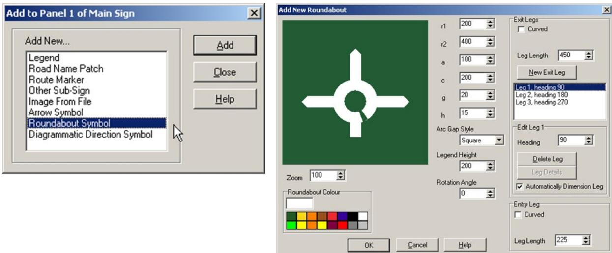
Various types and sizes of roundabouts can be designed in the **Add New Roundabout** dialogue box. Three sections are can be accessed through various boxes in each, where a number of options for specific designs can be entered, as detailed in Table 2.6.8.
