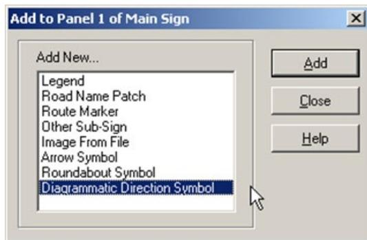
Various types and sizes of diagrammatic direction symbols can be designed in the created **Add New Diagrammatic Direction Symbol** dialogue box, shown in Figure 2.6.9(b).
