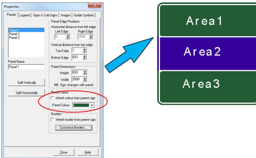
It is, therefore, not possible to achieve internal panel corners when a different coloured border is required in that separate panel, as shown in Figure 2.7.4.6(e).
