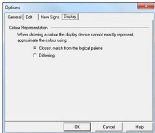
The options on this screen set the colouring characteristics of TraSiCAD when non-system colours are displayed and represented.
