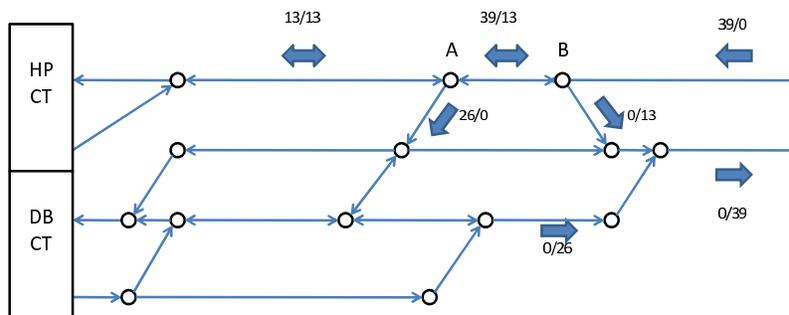
These charts show the current and proposed rail infrastructure feeding the two ports. Data above each arrow indicates the daily up and down train movements. Every two hours a train from Hay Point has to cross incoming trains into DBCT. There are two more crossover points between the port and Jilalan Yard.
