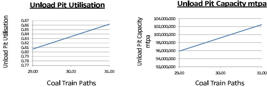
The charts below demonstrate the impact of train turnaround time, unloading time and train numbers on unload station capacity.
