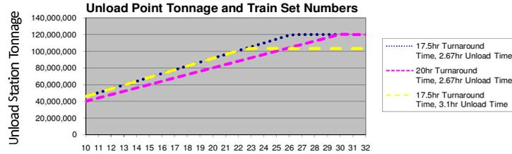
Increasing the number of train consists beyond the unload station capacity slows the system down with no increase in tonnes railed.
