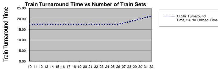
This chart shows the utilisation of train sets for a given system design (Coal train paths, train turnaround times). Demonstrates that 24 train sets are required to achieve target conditions (CTP 30, train T/T of 17.6hrs) with a utilisation of approximately 92%.
