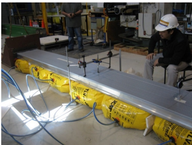
Figure C3.1(b) – Typical arrangement - Airbag
