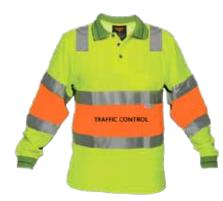
Bio-motion formation taping means that the retroreflective taping is placed on the clothing at either side of the movable joints of the body. This makes the traffic controllers far more conspicuous to drivers in low light situations.
