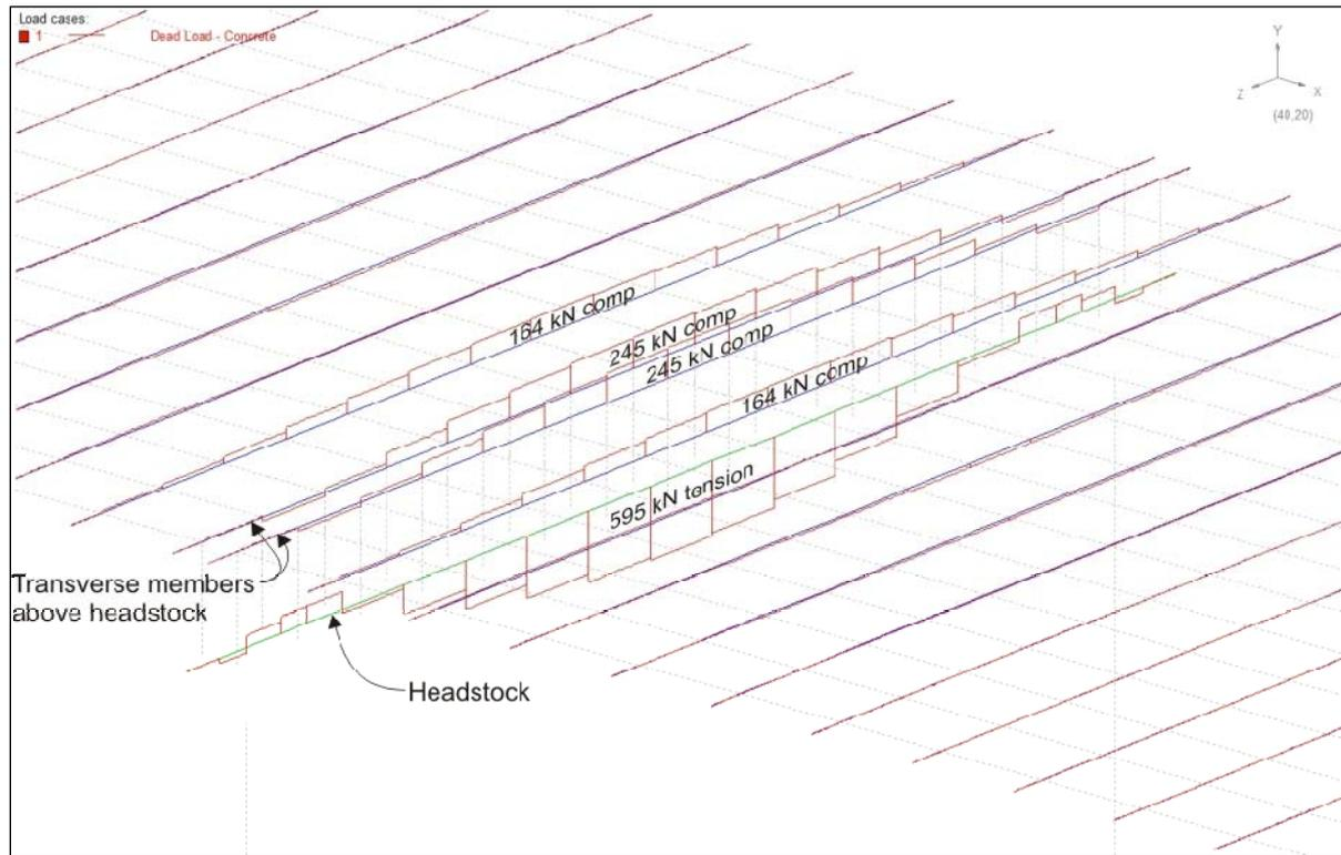
**Figure A.4: Transverse shear forces in links between headstock and superstructure**
