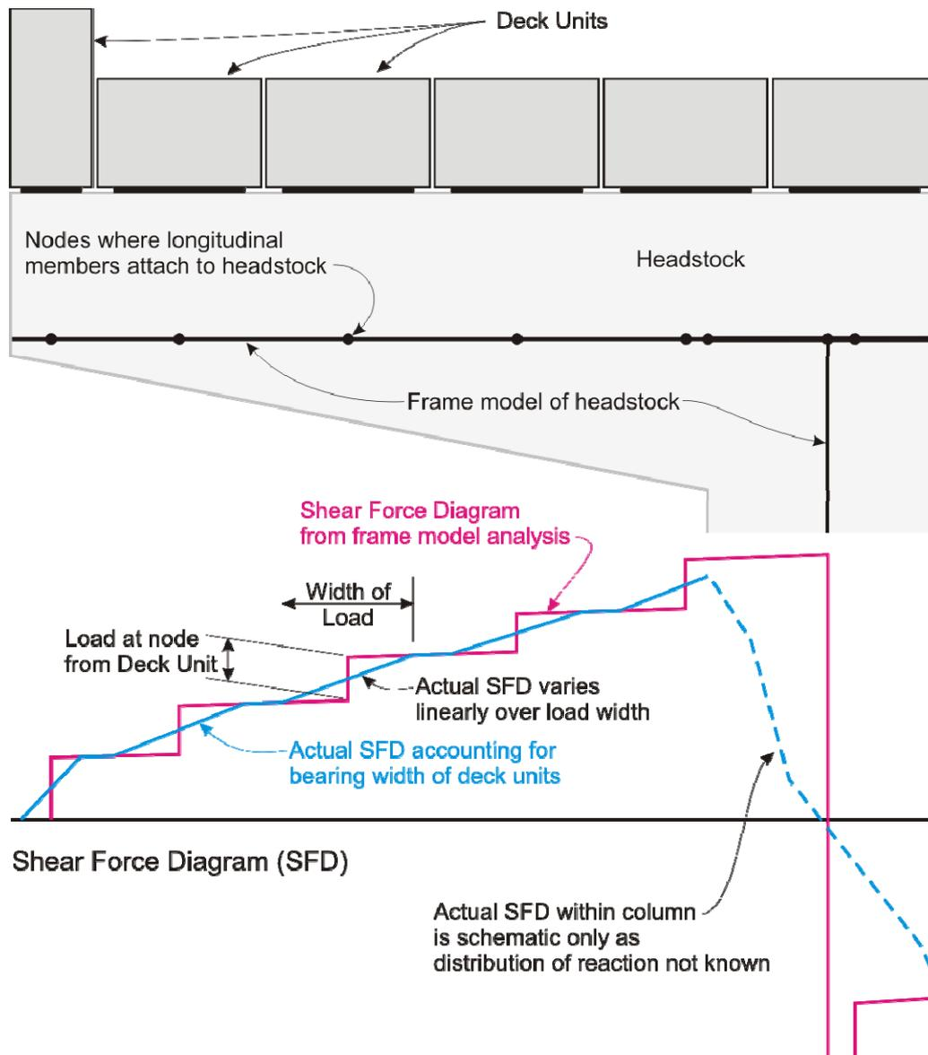
Figure A.16 shows the shear force diagrams for a cantilever headstock on a deck unit bridge. In this case the deck units are supported on bearings so the support is not quite continuous. In this example, it is assumed the ends of the deck units are torsionally released as recommended in Section A.4, so that there is no torsion to be transferred from the deck units into the headstock and the reaction from each deck unit is uniformly distributed over the width of the support.
