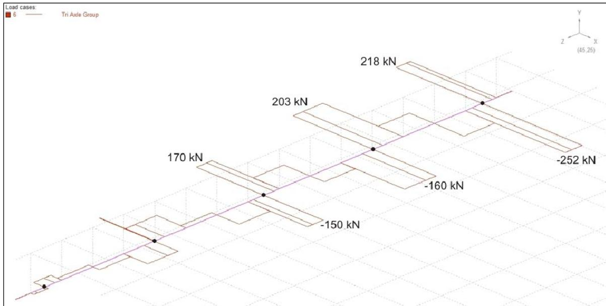
**Figure A.10: Bending moments in deck units showing negative end moments due to longitudinal restraint**
