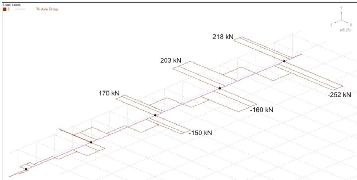
**Figure A.10: Bending moments in deck units showing negative end moments due to longitudinal restraint**
