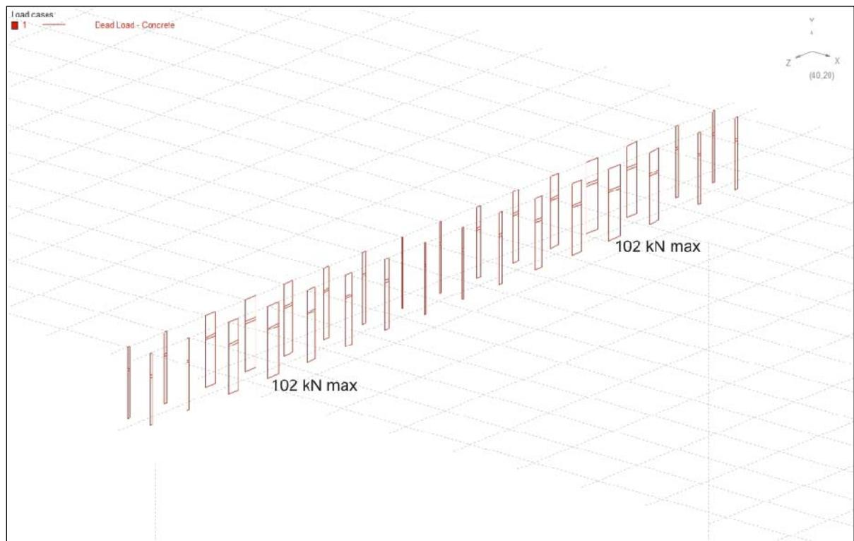
Figure A.4 shows the transverse shear forces in the links between the headstock and the superstructure. This is for unfactored dead load only and under factored dead load plus live load
