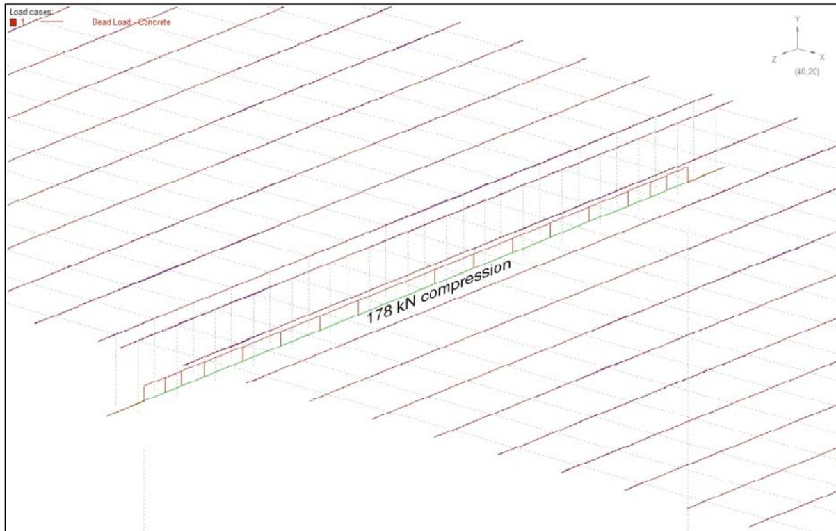
It can be seen from this example that if the bridge is to be modelled with the superstructure and the headstocks in their correct relative elevation, then it is important to ensure the properties of the links joining the two are such that composite action cannot be developed. Results should be checked to ensure this has been achieved.
