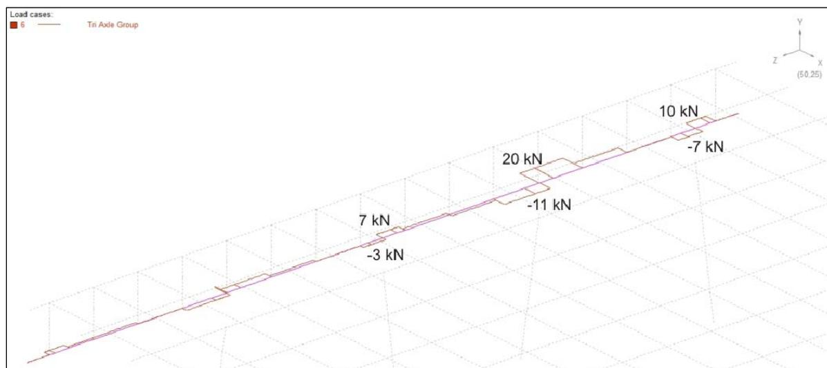
**Figure A.12: Deck unit moments in model with headstock supported on short piles**
