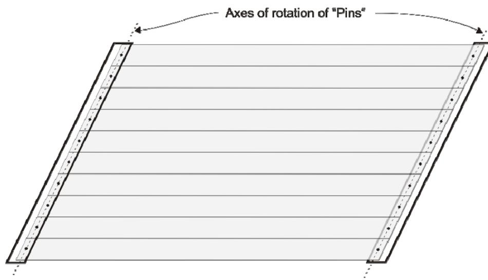
Skewed supports can complicate the modelling of such structures, as it means the pin cannot be simply modelled (in SpaceGass) as an end release on the member representing the deck unit. Rather, a more complicated model with stub members perpendicular to the pier containing the end release is required.
