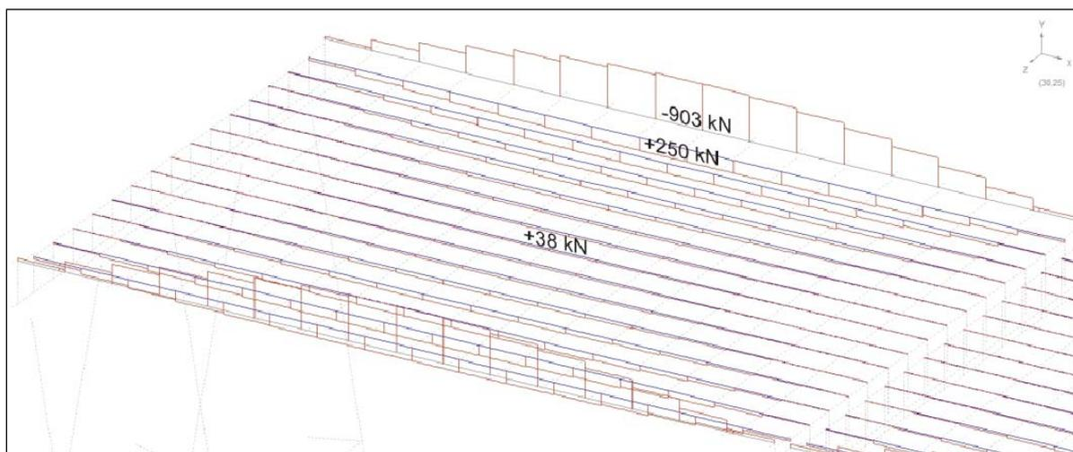
As can be seen this results in a significant compressive force in the kerb unit, and tensile forces in the deck units. These forces are large in the deck unit adjacent to the kerb unit and then reduce towards the middle of the bridge. As a result of this composite action, the bending moments in the deck units are lower.
