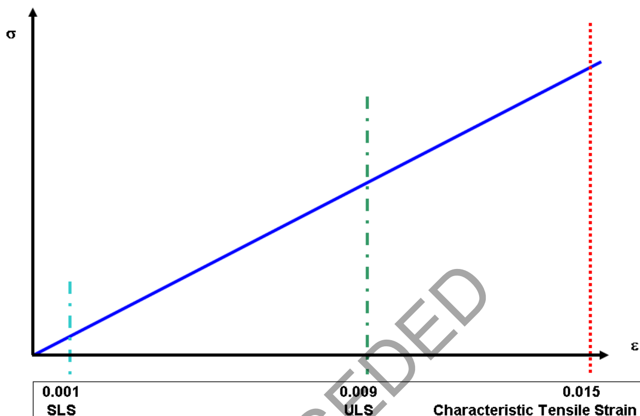
Figure 16.8.1 – ULS and SLS strain limitations
