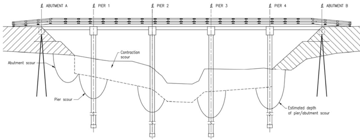
**Figure 1.2: Components of scour at a bridge**
