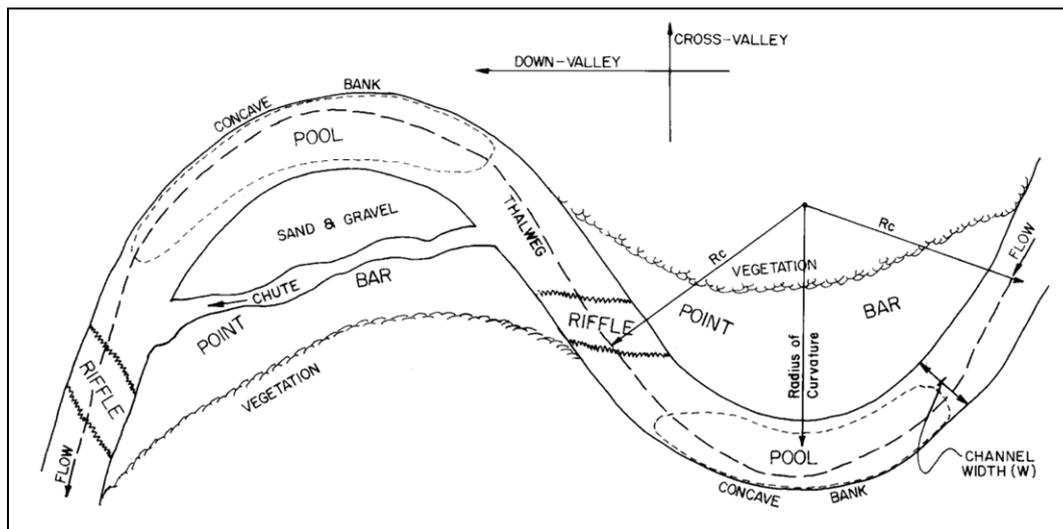
**Figure 1.3.3D: Plan view of a typical meandering stream (HEC20, 2012)**
