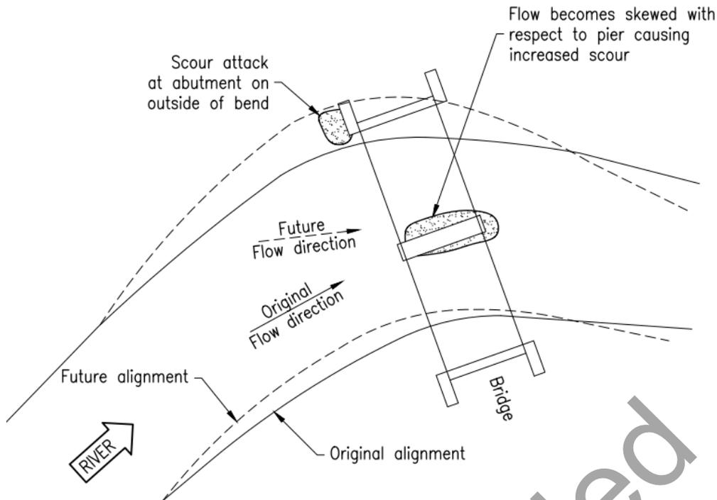
**Figure 2.4.4: Change in channel alignment causing skewed flow and scour potential (CIRIA 2005)**
