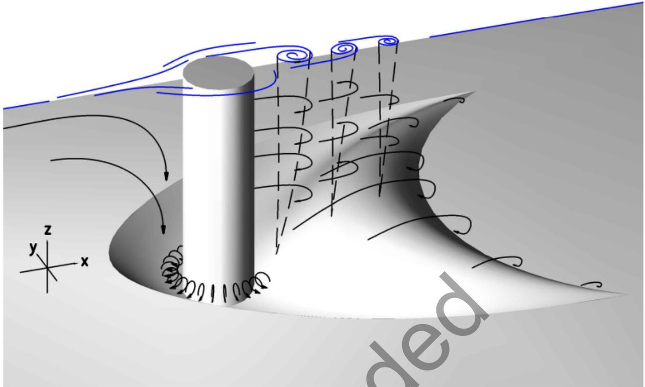
**Figure 1.5.1B: Flow profile around a circular bridge pier. Vortices form downstream. (HEC18, 2012)**
