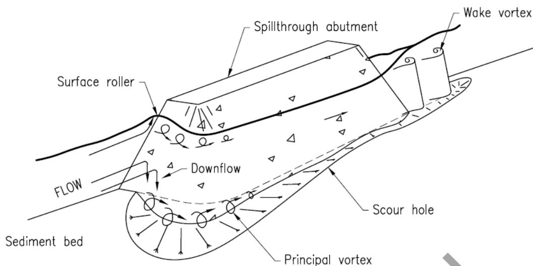
**Figure 1.5B: Scour at a bridge abutment (HEC-18, 2012)**
