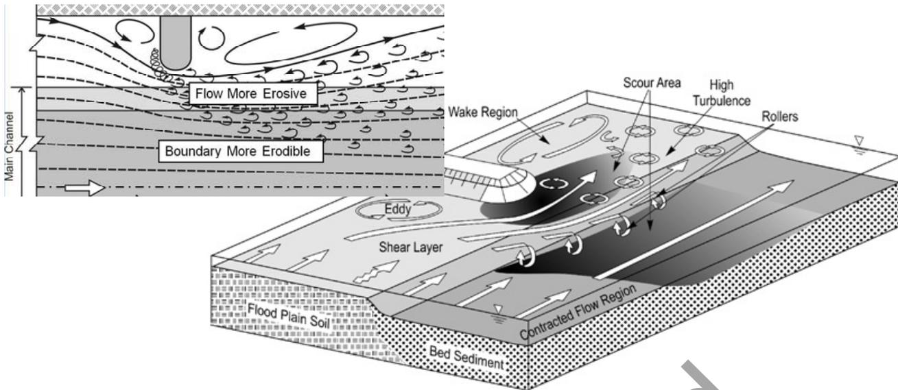
**Figure 1.5.3B: Flow structure generated by floodplain/main channel flow interaction (NCHRP 2011b)**
