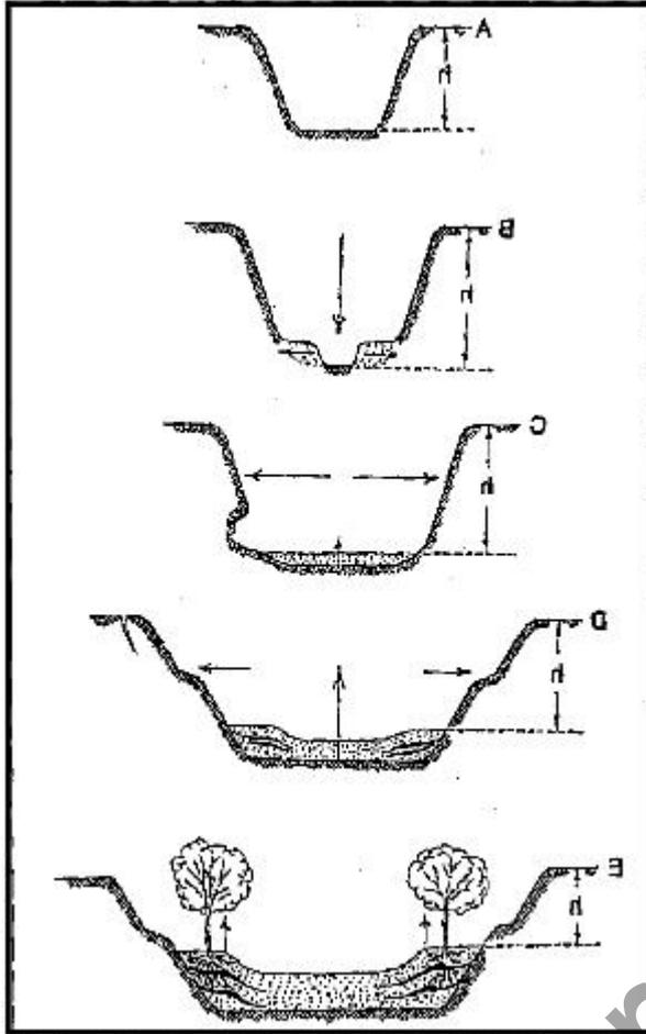
**Figure 1.3.3A: Evolution of incised channel from initial incision (A, B) and widening (C,D) to aggradation (D,E) and eventual relative stability (Schumm et al 1984)**
