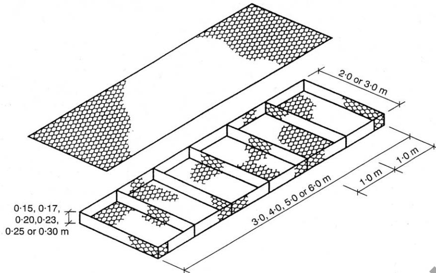
**Figure 3.5.1: Typical gabion mattress dimensions**
