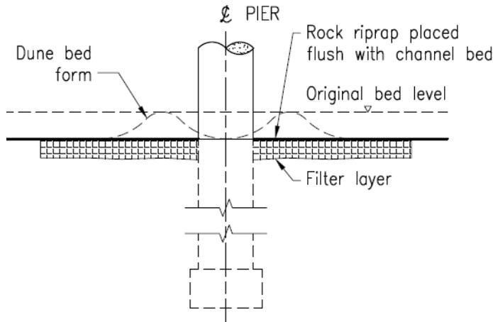
**Figure 3.4.2D: Schematic diagram showing sand filled geotextile container beneath pier riprap**
