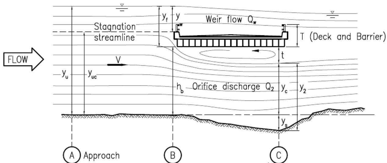
**Figure 1.4.3B: Vertical contraction and definition for geometric parameters (HEC-18, 2012)**
