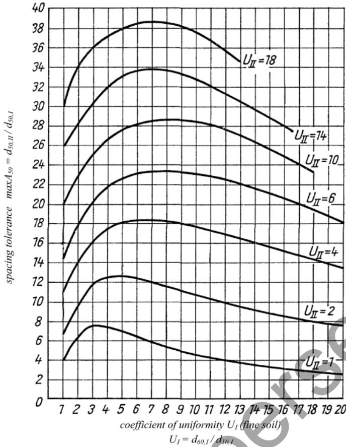
**Figure 3.3.2A: Selection of  $D_{50}$  size for overtopping granular layer**
