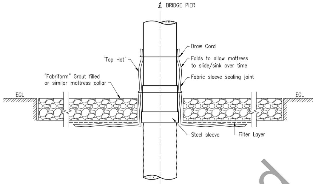
**Figure 3.5.4: A possible flexible collar arrangement at a pile to seal joint with a mattress**
