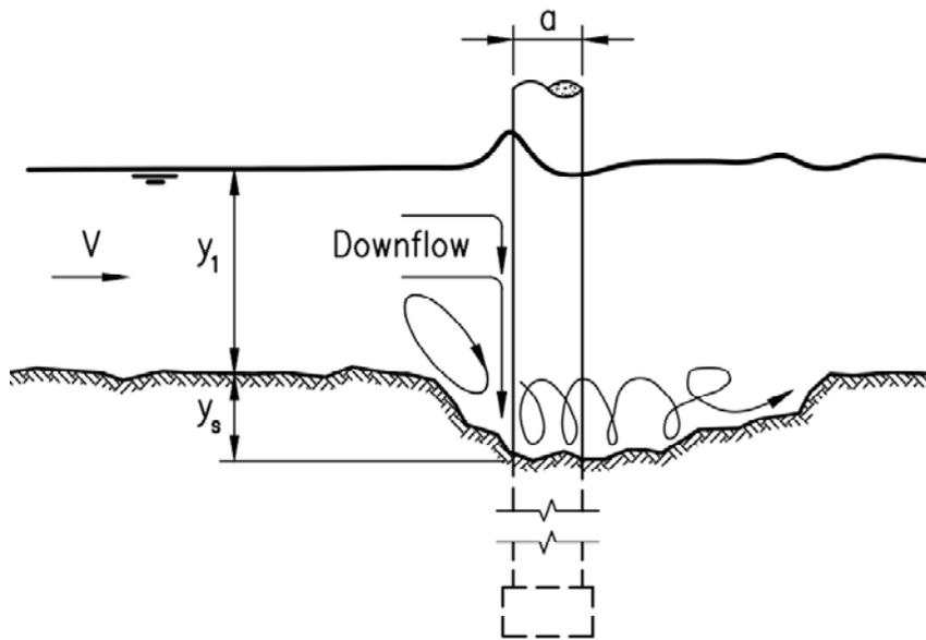
**Figure 2.5.6A: Definition sketch for circular pier scour**
