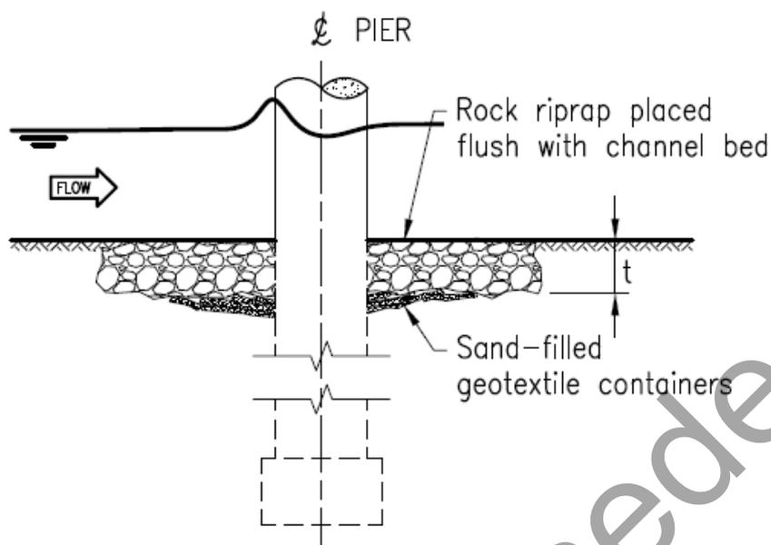
**Figure 3.3.4: Schematic diagram showing the use of sand filled geotextile as a filter**
