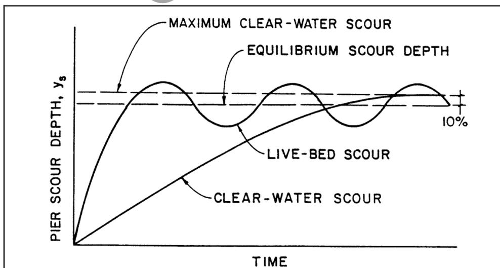
**Figure 1.4.2: Pier scour depth as a function of time**
