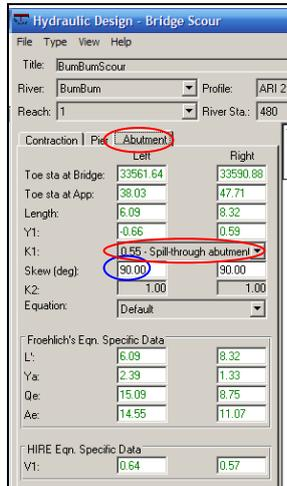
**Figure 2.7D: Bridge Scour module – Abutment Scour**
