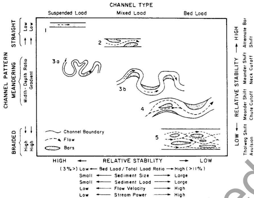
**Figure 1.3.3B: Channel pattern and relative stability (Shen et al, 1981)**
