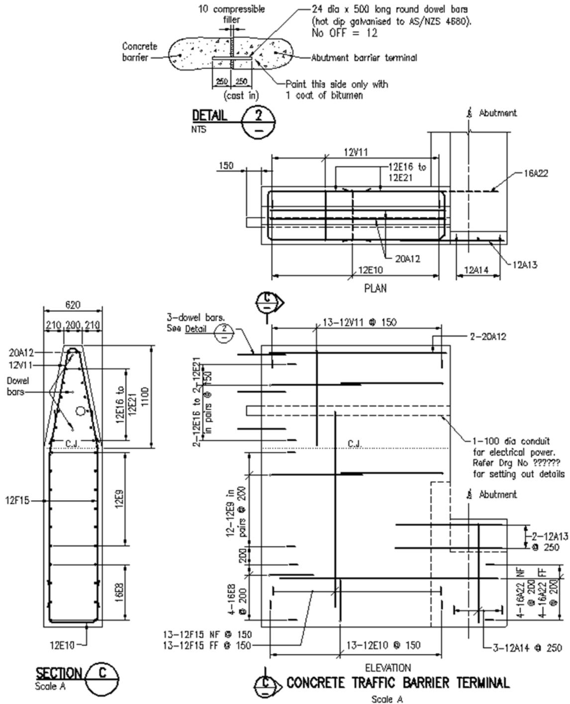
**Wingwall (concrete traffic barrier type) connection to guardrail**
