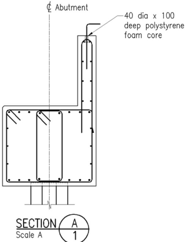
**Wingwall reinforcement (bridge steel traffic barrier type)**
