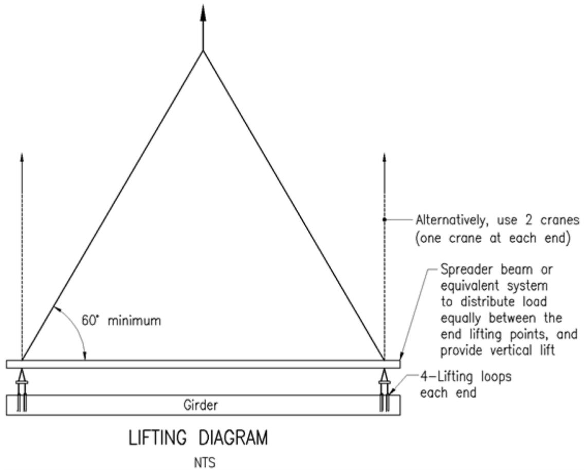
Figure 14.11(b) - Lifting loop details
