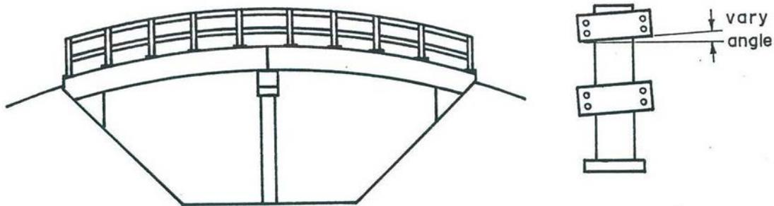
In the transverse direction, posts are to be set vertical except on bridges where the deck super elevation/crossfall slope exceeds three per cent. In these cases posts are to be set normal to the super elevation/crossfall. Refer Figure 19.4-4 *Post Orientation in Transverse Direction*.
