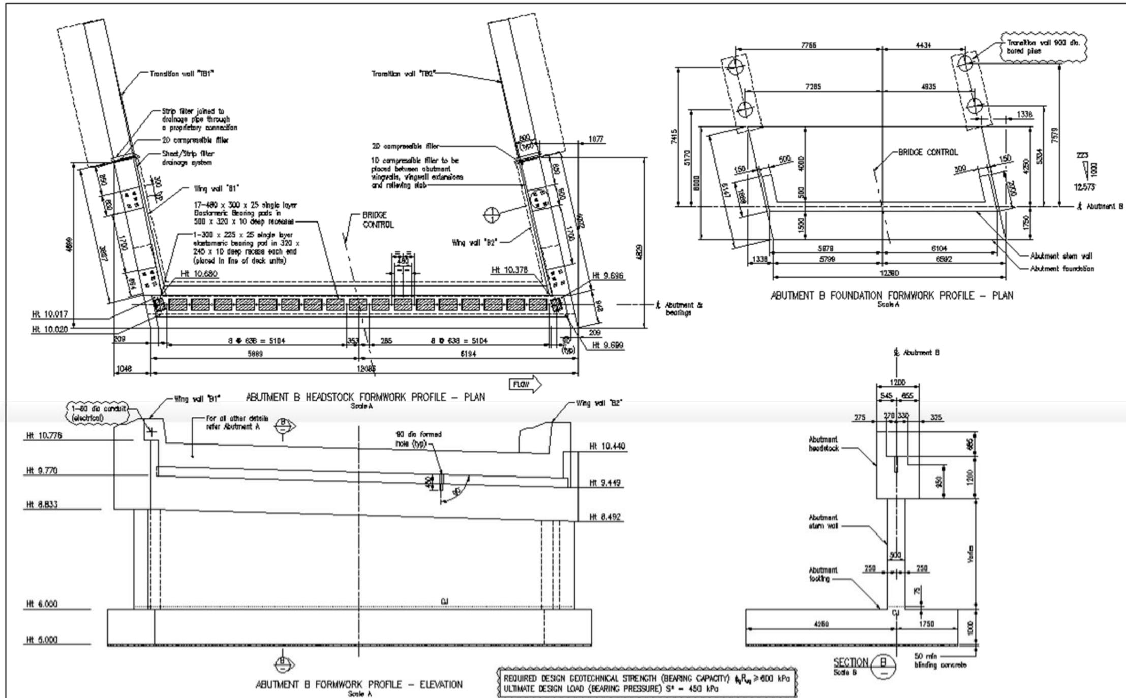
REQUIRED DESIGN GEOTECHNICAL STRENGTH (BEARING CAPACITY)  $f_{d,R_{90}} \geq 800$  kPa
