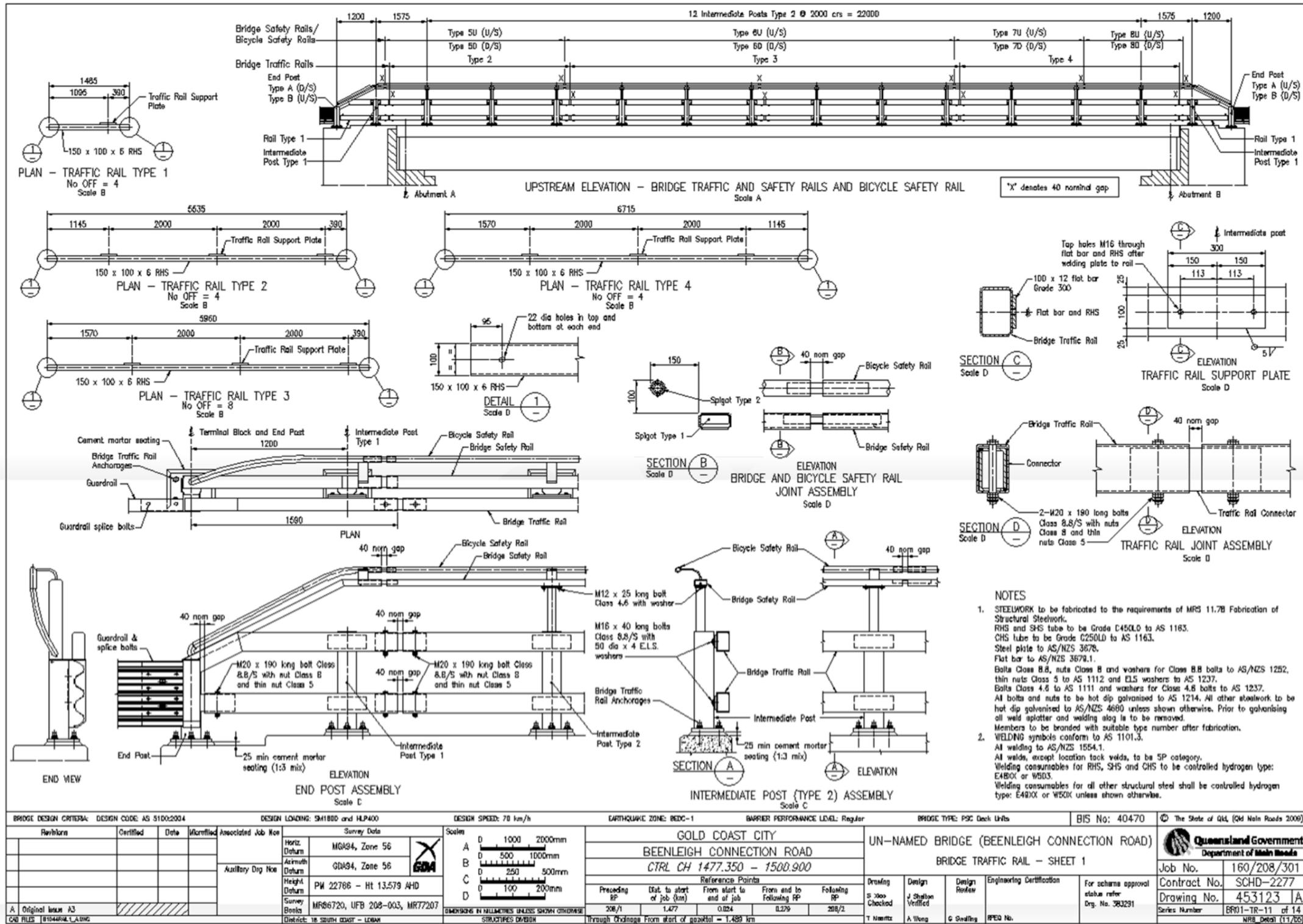
Appendix G – Example Steel Bridge Traffic Barrier with Bicycle Safety Rail Drawing – Sheet 2
