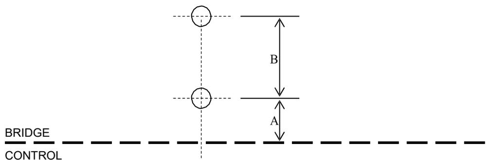
Where raked piles are used, a note shall be added to the drawing stating that the location shown is at the underside of the headstock / pilecap into which the pile is bonded. Raked piles are also to have the slope of the rake noted together with an arrow showing the direction of the rake.
