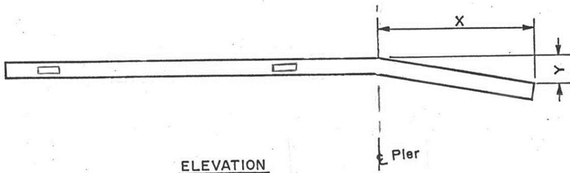
**Bending of Rails for Horizontal Curves**
