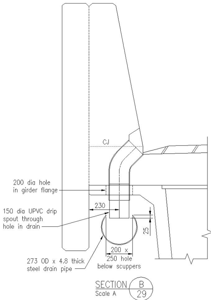
The drain pipe is supported by a steel drain bracket which passes through 20 mm diameter holes in the girder flange. Refer *Figure 14.10(a) - Plan view of hole layout* and *Figure 14.10(c) - 200 mm diameter holes in girder flange drain bracket*.
