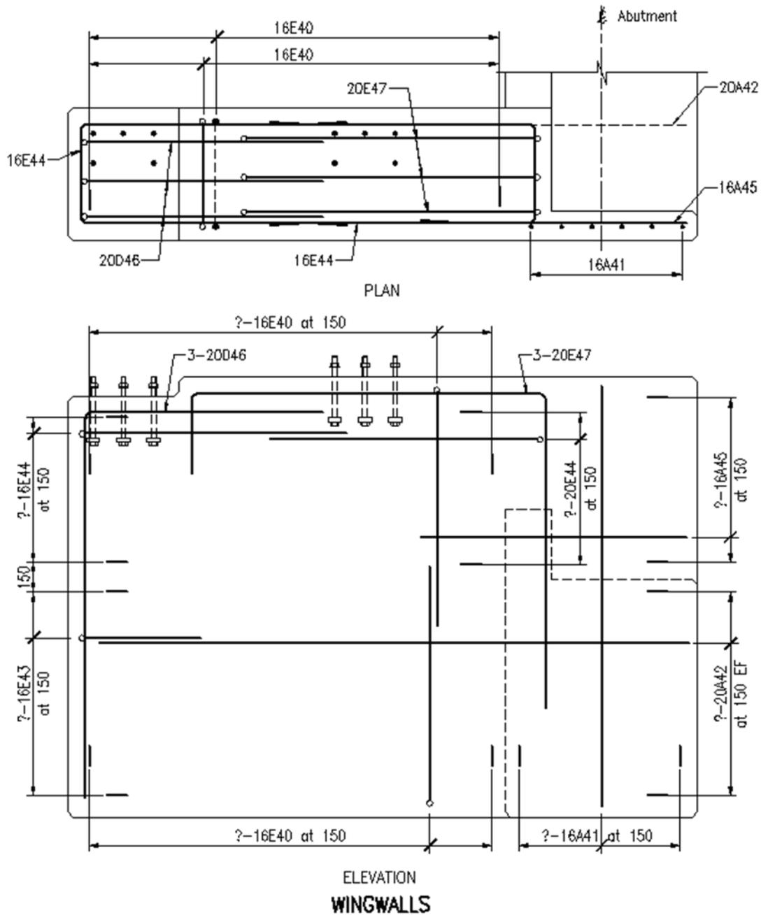
**Wingwall reinforcement (concrete traffic barrier type)**
