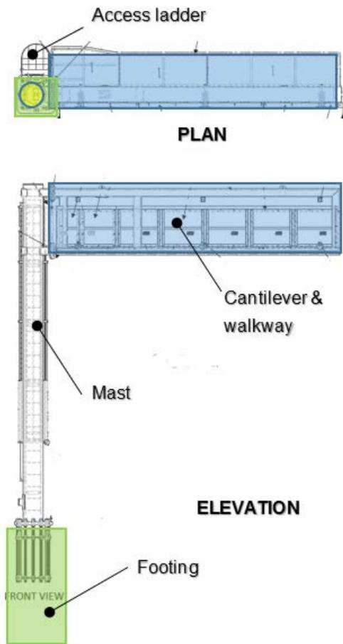
Figure 21.6(b) - Multi Post Gantry (lightweight gantry shown)
