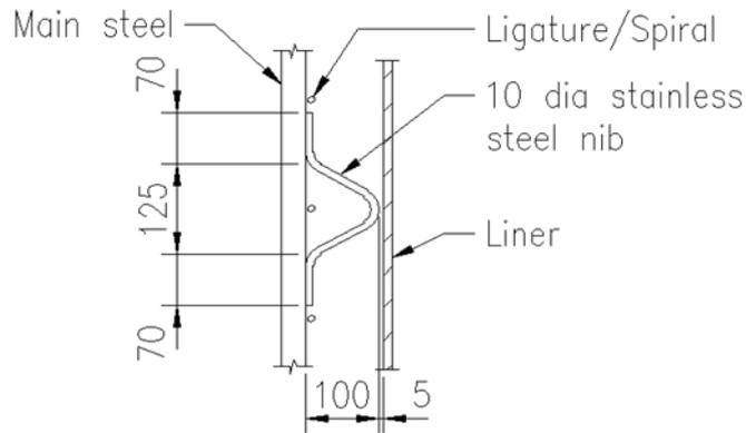
1 set of 4 stainless steel nibs (equally spaced around the circumference of the cage) to be welded securely to main steel at intervals of 4000 maximum on welded cages and 2500 maximum on unwelded cages. There must be at least 2 sets of stainless steel nibs per cage. Stainless steel nibs shall be placed approximately in line and straddle the ligature/spiral as shown
