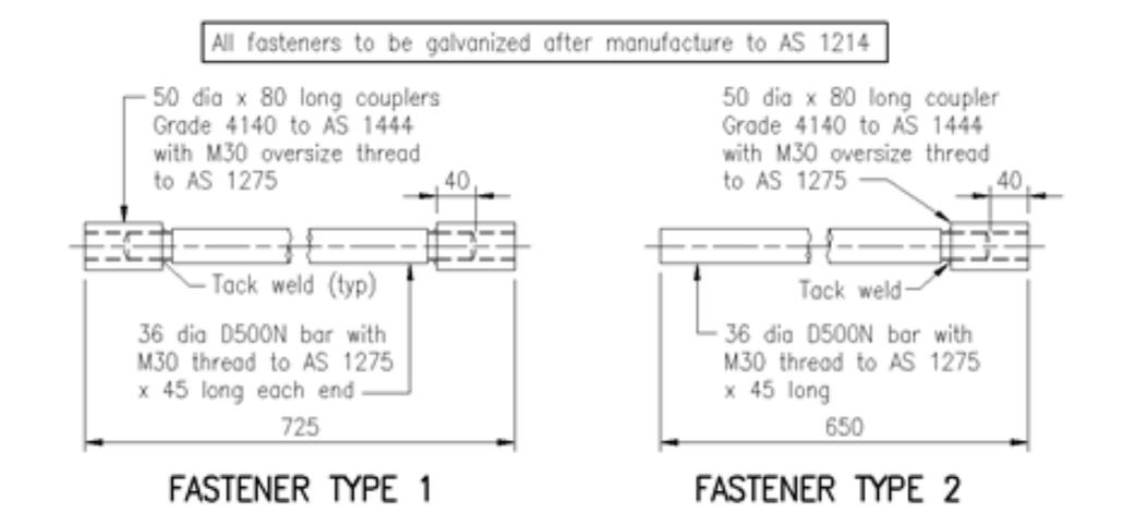
A detailed view (minimum scale of 1:10 on an A1 drawing) shall show how the fasteners, top attachment plate and reinforcing steel fit together in the end block.
