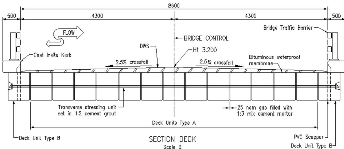
**Figure 11.5(d) - Concept GA Drawing - Typical section girders**
