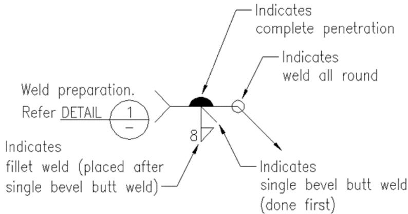
**Figure 6.8-8 - Bridge Traffic Barrier Post to Anchor Plate**
