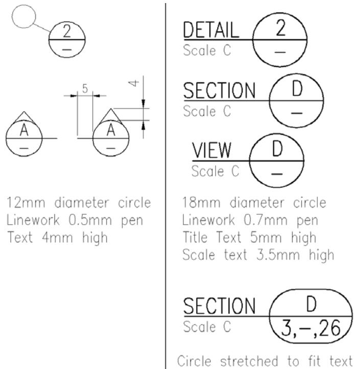
**Figure 2.7-2 - Examples of Sections and Details**
