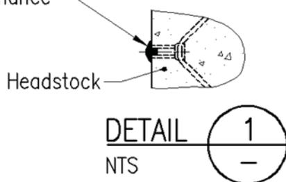
The details shown in Figure 12.18(b) *Eyebolt Details* shall be shown on the maintenance and inspection drawings. It refers back to the abutment drawing for the insert details.
