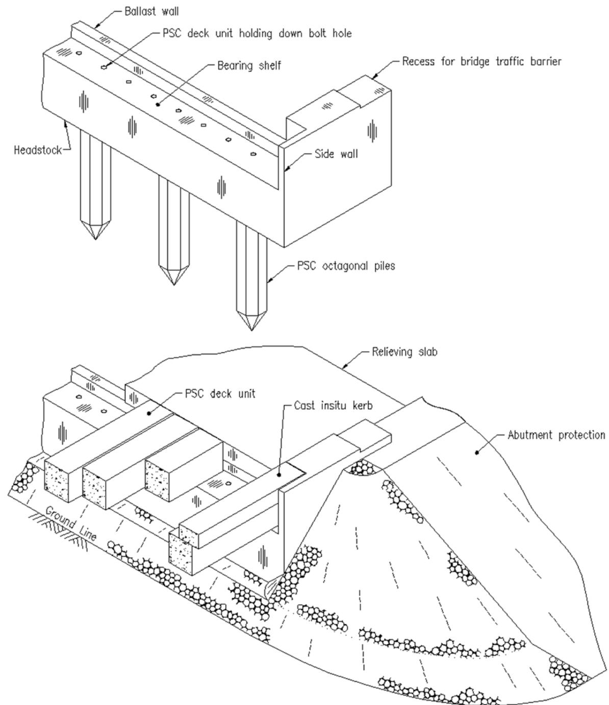
FIXED ABUTMENT WITH PSC PILES, PSC DECK UNITS AND CAST INSITU KERBS
