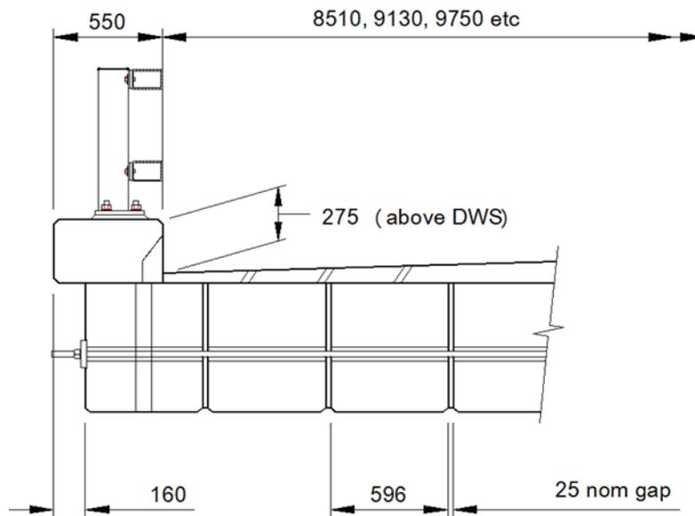
**Gap between deck units (Transversely Stressed)**
