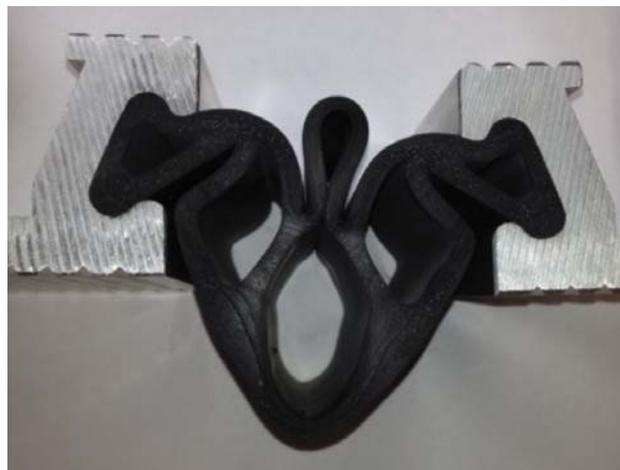
*D* seal glands are not as bulky as *F* seal glands, and can therefore close to zero gap. Refer Figure 18.3-2 *Draped (D) Seal Minimum Closed Gap*.
