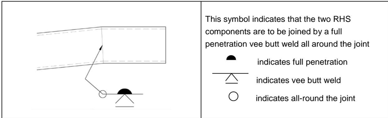
The weld shown in Figure 6.8-6 - Bridge Traffic Barrier Post to Base Plate is a critical structural weld and its conformance to specification is vital to the performance of bridge traffic barrier posts under load. This is a complete penetration butt weld (compound butt weld placed first followed by a fillet weld). Refer Figure 6.8-8 - Combination Butt and Fillet Welds for description.
