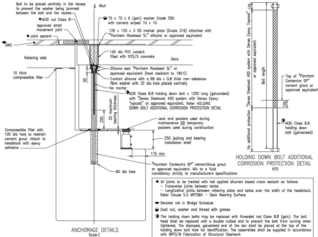
★ All joints to be treated with hot applied bitumen based crack sealant as follows:
