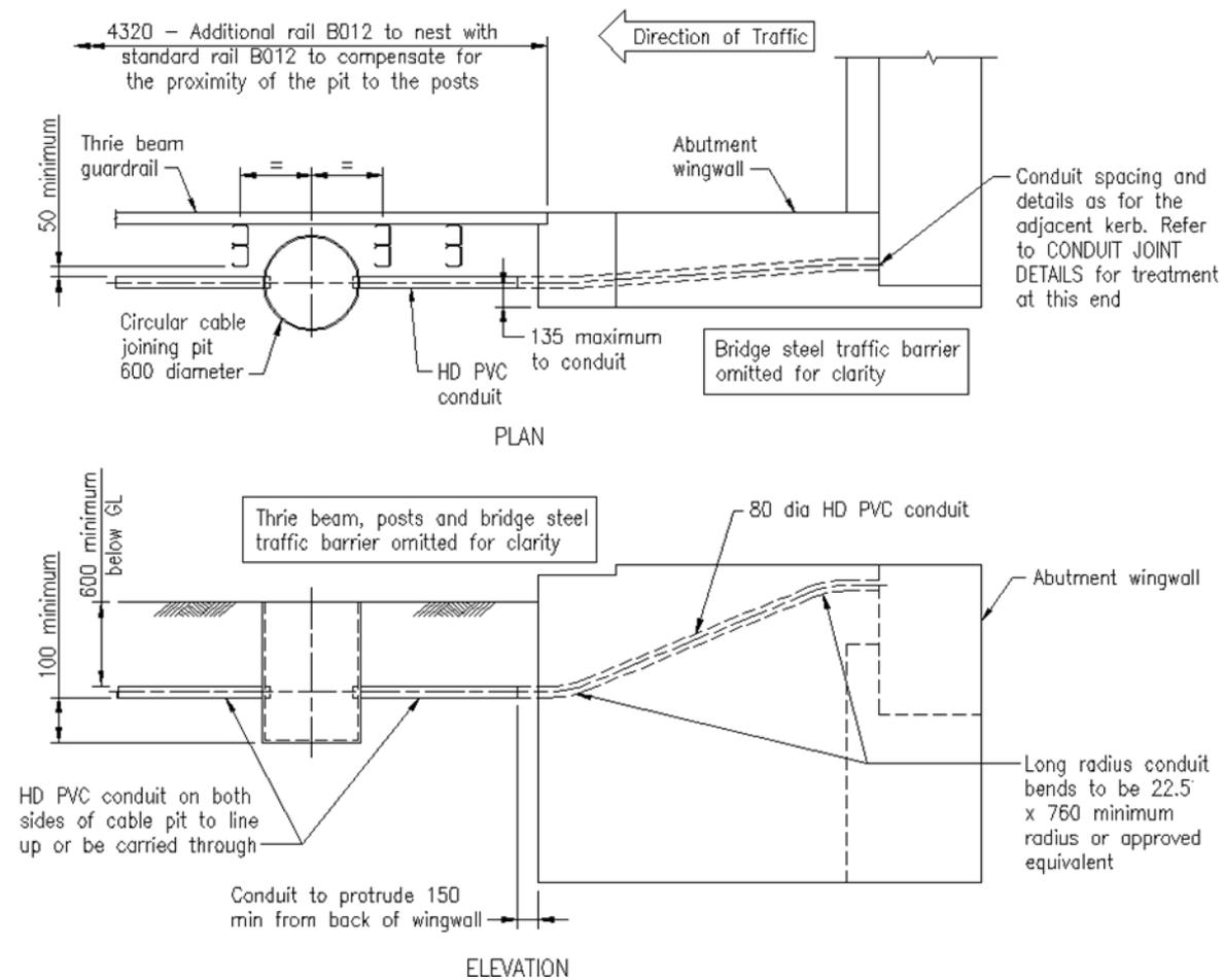
**12.12 Abutment headstock additional details****Abutment headstock drainage**
