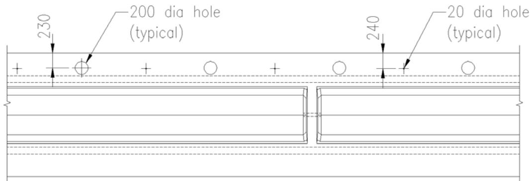
**Figure 14.10(b) - 200 mm diameter holes in girder flange for scuppers**
