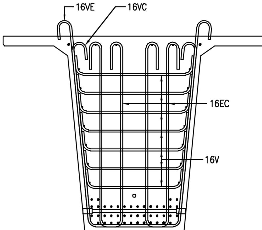
Note: The 16V bars sit inside the 16VE bars so that the set is only two bars wide ( $16EC + 16VE + 16VC$ ) and not three ( $16EC + 16V + 16VE$  or  $16VC$ ).
