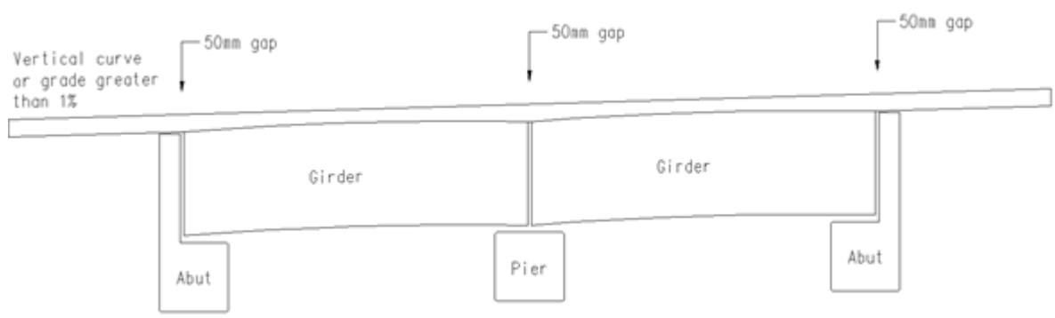
When end incline dimensions are shown on a drawing, three sets of distances are required. These are the distances at transfer, at 30 days, and at 100 days after casting. The transfer figure tells the casting yard what offsets the girder ends must have immediately after it has been cast and is leaving the form.
