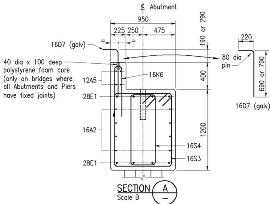
If the bridge deck has crossfall both ways from the bridge centreline and the abutment ballast wall ignores the crossfall, the relieving slab will require end thickening. The highest bar and lowest bars must be dimensioned on the abutment drawing. The starter bars shall all be the same size and shall be bonded a minimum of 500 mm into the ballast wall. Refer Transport and Main Road's Standard Drawings 1505 and 1506 and Figure 12.17(c) *Variable Relieving Slab Starter Bars*.
