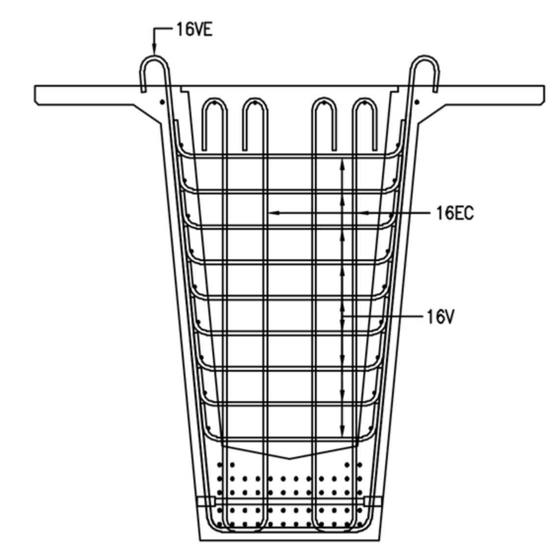
Note: The 16V bars sit inside the 16VE and 16EC bars so that the set is only two bars wide (16EC and 16VE) and not three (16EC and 16V and 16VE).
