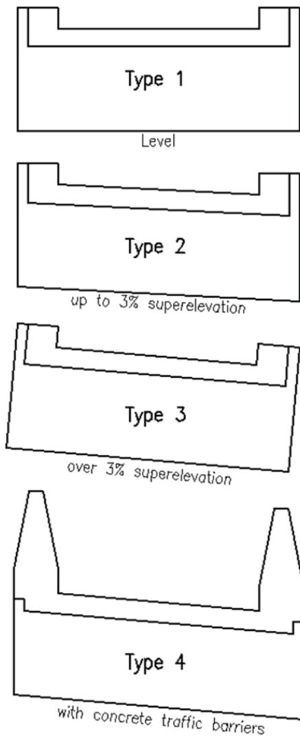
**Abutment wingwall recess for regular performance level bridge steel traffic barrier connecting to thrie beam guardrail**
