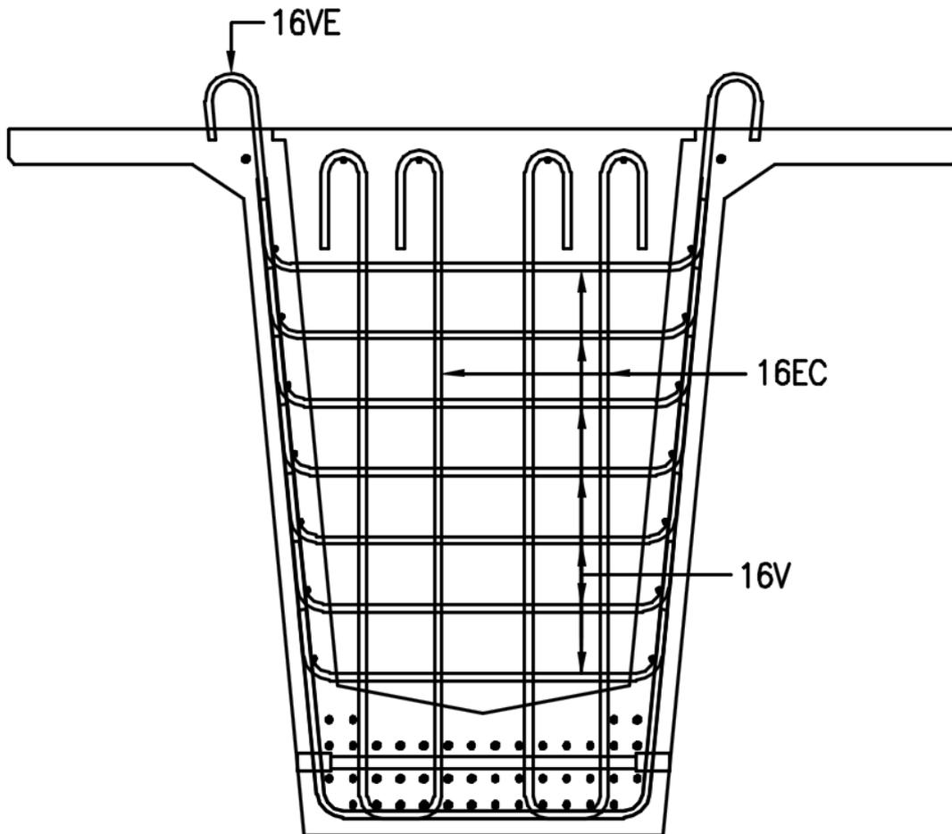
Note: The 16V bars sit beside the 16VE and 16EC bars so that the 12A longitudinal bars have sufficient cover to the void. The reinforcing set is three bars wide, however the sets are not spaced as closely as they may be in the end block.
