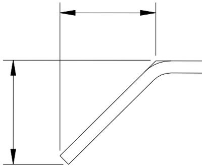
When the angle for a bar shape can be either acute or obtuse, for example bar shape U, the computer calculates the angle and dimension C.
