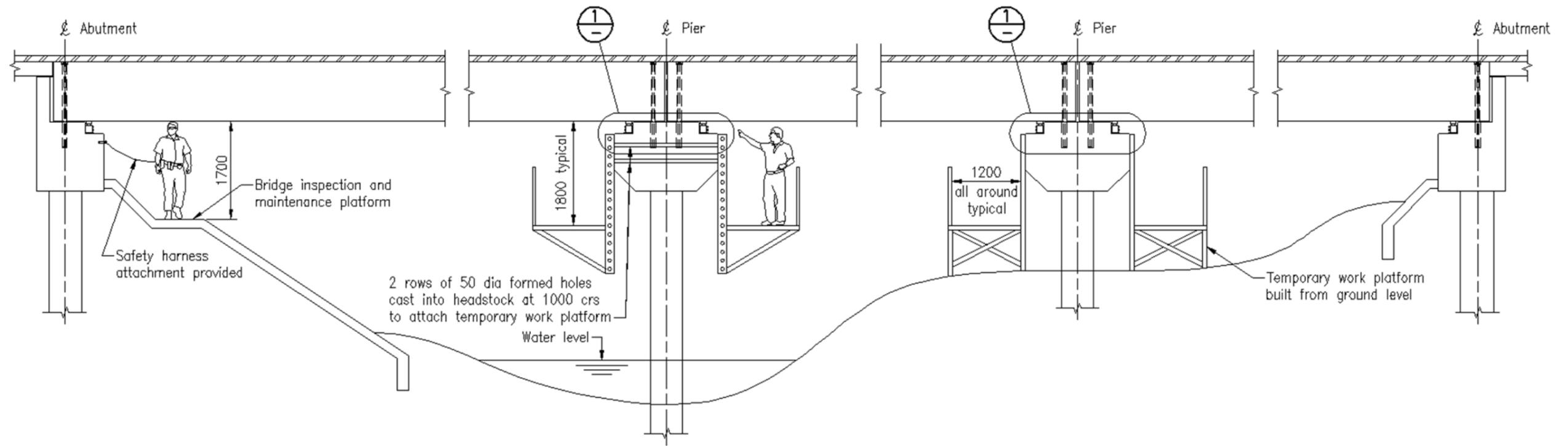
Appendix A – Example Bridge Jacking, Inspection and Maintenance Drawings
