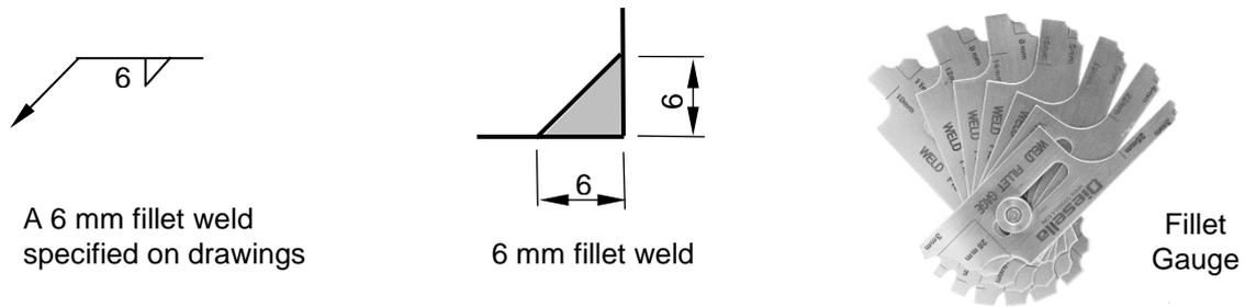
**Figure 6.8-3 - Weld on Arrow Side of Joint**
