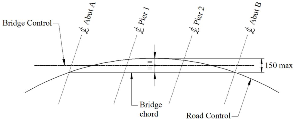
**STEP 2** - If the combination of small radius curve and length of bridge makes it impossible to maintain a straight bridge alignment, then it is necessary to locate the bridge around the curve with each span set out as a parallelogram. Refer Figure 10.4-3 - Span Offset 75 mm Maximum and Figure 10.4-4 - Span Offset 150 mm Maximum.
