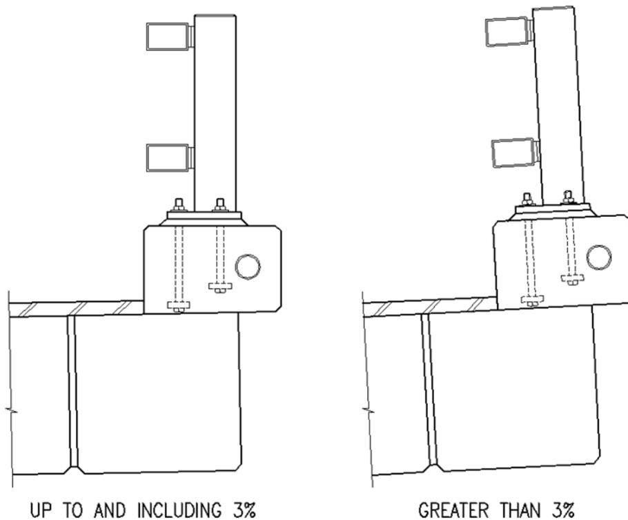
**Bending of Rails for Vertical Curves**
