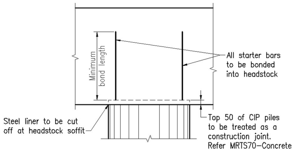
**Bonding of column / stem / blade steel**
