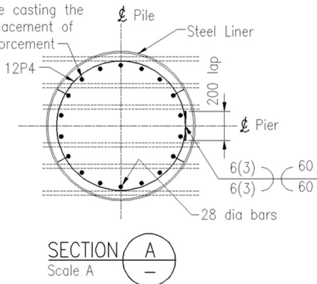
**Lap position of main reinforcement in headstock / pilecap**
