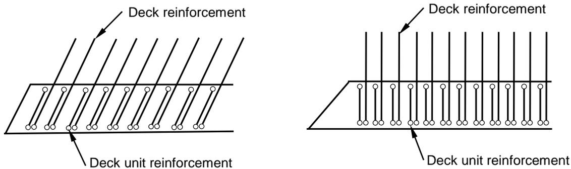
The starter bars that protrude into the deck can be one of two shapes. When there are only small gaps between deck units (up to 50 mm), the bars can be vertical as shown in Figure 15.12-3 *Close Gaps between Deck Units*.
