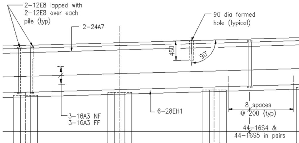
**Bonding of PSC pile steel**
