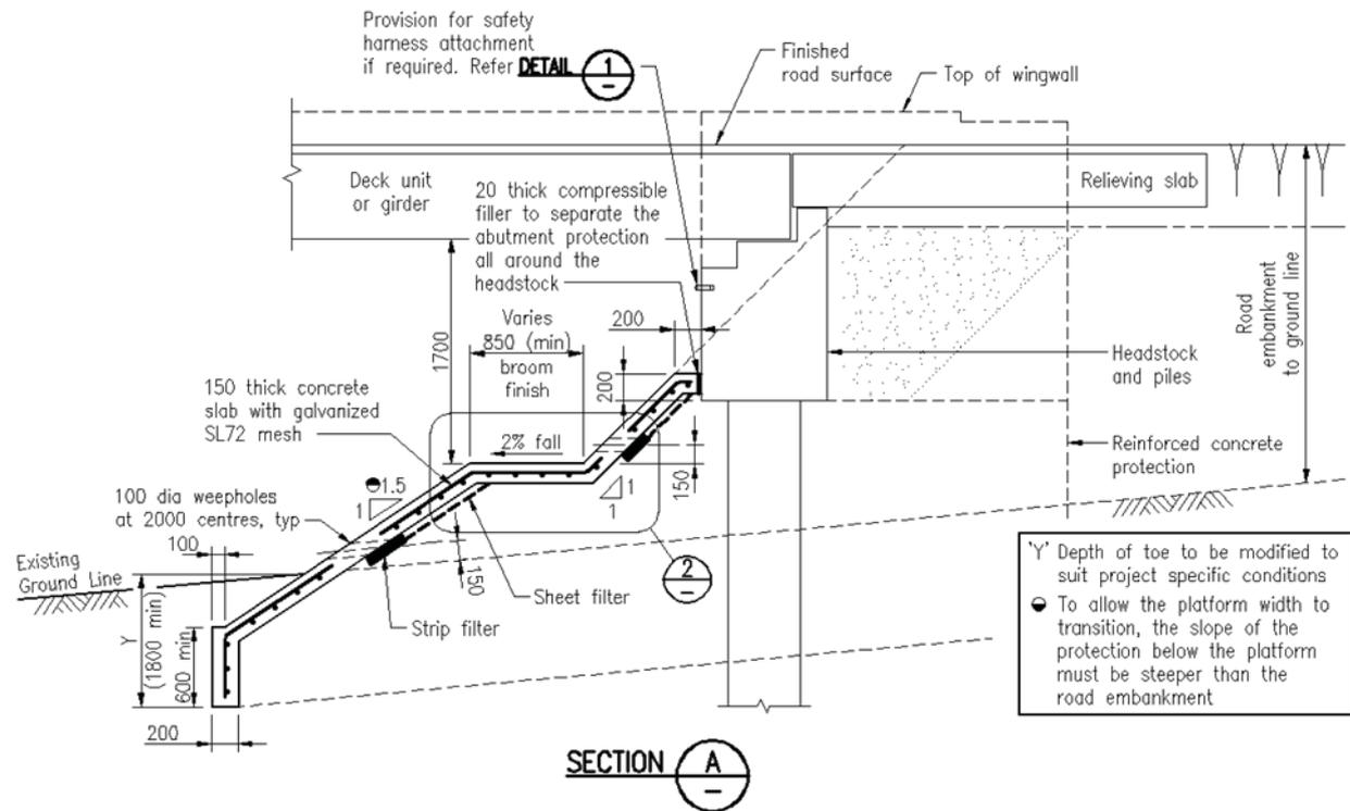
**Staircase Access to the Inspection & Maintenance Platform**
