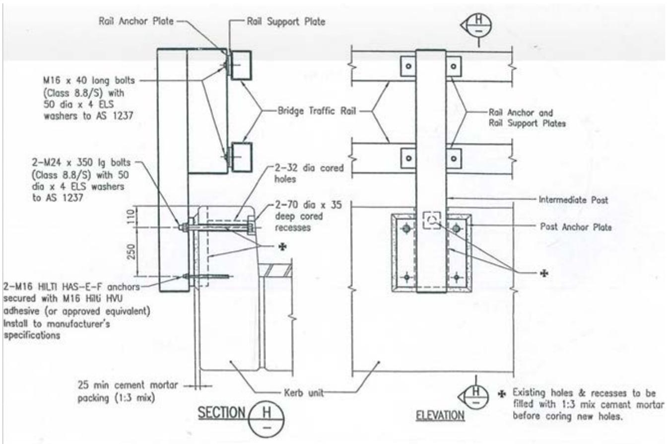
Usually the existing wingwalls need to be extended to provide an anchorage for the bridge traffic barrier end posts to be attached. Refer Figure 19.8-3 *Example Wingwall Extension* for typical details.
