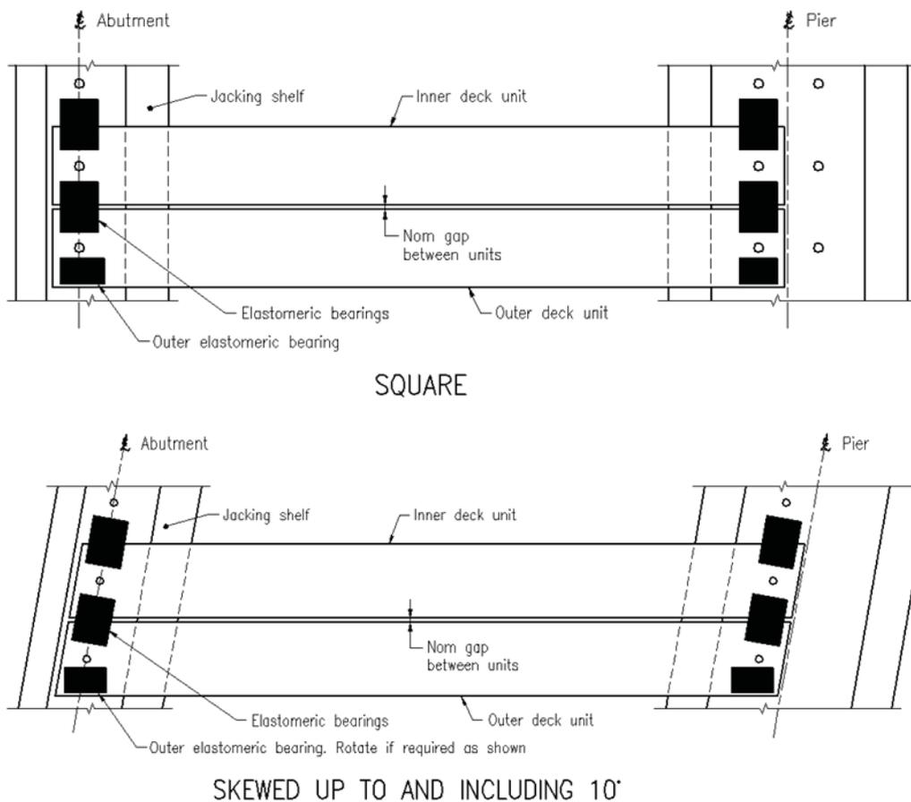
On bridges skewed more than  $10^\circ$  or bridges that have a nominal gap between the deck units greater than 40 mm, the bearings shall be positioned in front of the deck unit holding down bolt holes, and square to the longitudinal axis of the deck unit. They are positioned in this manner to avoid unequal loading of each half of the bearing which would happen if it was positioned between the deck units. Refer Figure 12.15(b) *Alignment of Bearings on Deck Unit Bridges Skewed  $>10^\circ$* .
