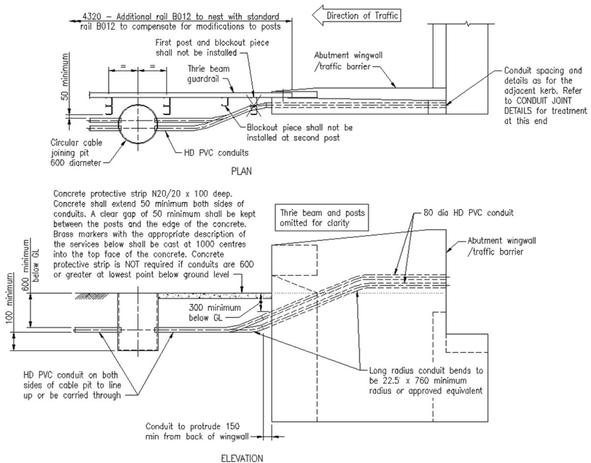
**Figure 12.11(b) - Thrie beam connecting to bridge steel traffic barrier**
