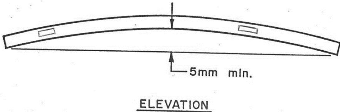
On bridges with a VC or changing grade and with linear kerbs, rails shall be bent at the pier and abutment centrelines if necessary. Refer Figure 19.4-6 *Rail Bent for Linear Change of Grade Vertically*.
