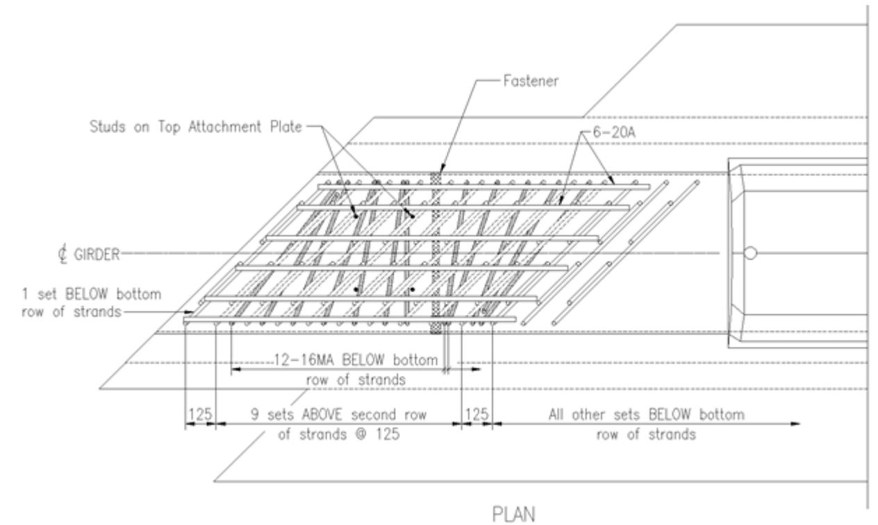
**Figure 14.7(e) - Girder reinforcement around fastener (2)**
