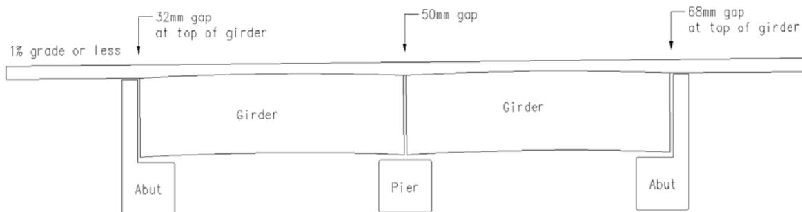
For bridges on a grade of 1% or less, the ends of the girders are not vertical, but are perpendicular to the bottom of the girder (after 100 days).
