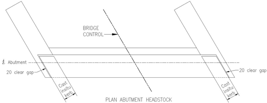
On skewed bridges the Drafter must check that the abutment side walls will not interfere with the transverse stressing of the deck units. The side wall may need to be terminated to provide sufficient working room between it and the jack. Refer Figure 12.4(e) *Abutment Side Wall and Transverse Stressing Jack Clearance*.
