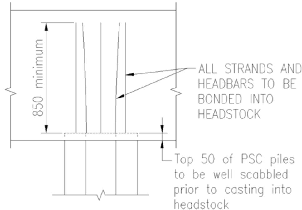
**Bonding of Cast-in Place (CIP) pile steel**
