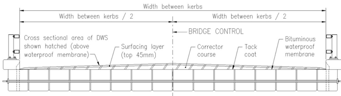
The mass of DWS for a span is measured in tonnes and is calculated as follows:
