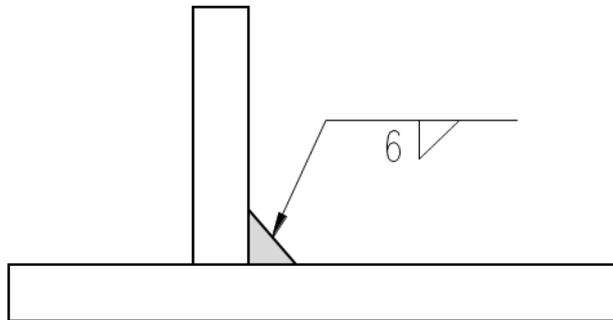
**Figure 6.8-4 - Weld on Both Sides of Joint**
