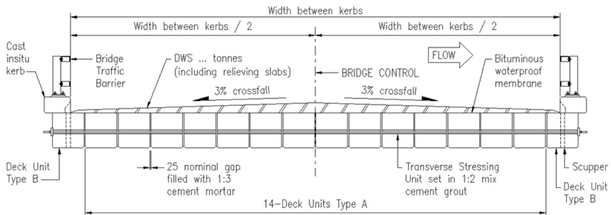
**Decks with Constant Crossfall or Superelevation.** Refer Figure 7.4-2 - Decks with Constant Crossfall/Superelevation.
