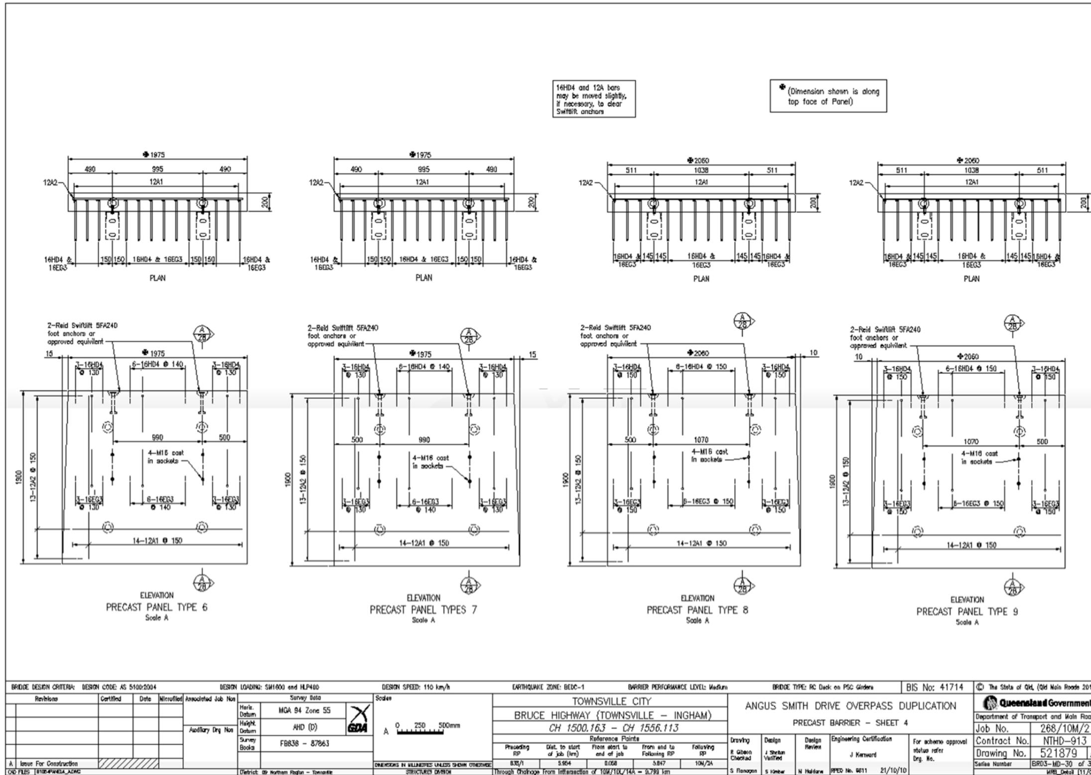
Appendix H – Example Precast Barrier Panel and Deck Drawings – Sheet 5
