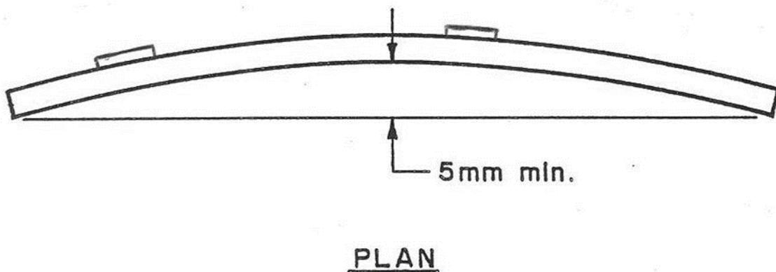
On bridges with a HC and with linear kerbs, rails shall be bent at the pier and abutment centrelines if necessary. Refer Figure 19.4-8 *Rail Bent for linear change of Direction Horizontally*.
