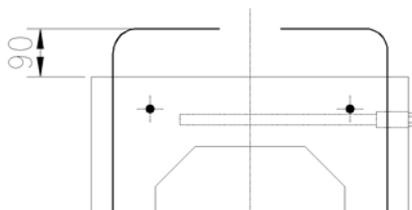
**Figure 15.12-4 Large Gaps between Deck Units**
