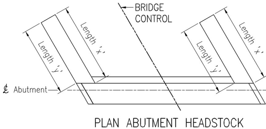
Refer to Design Criteria on Transport and Main Road's Standard Drawing No. 2200 for bridge traffic barrier post spacings and recess depth to be provided at the end of the wingwalls.
