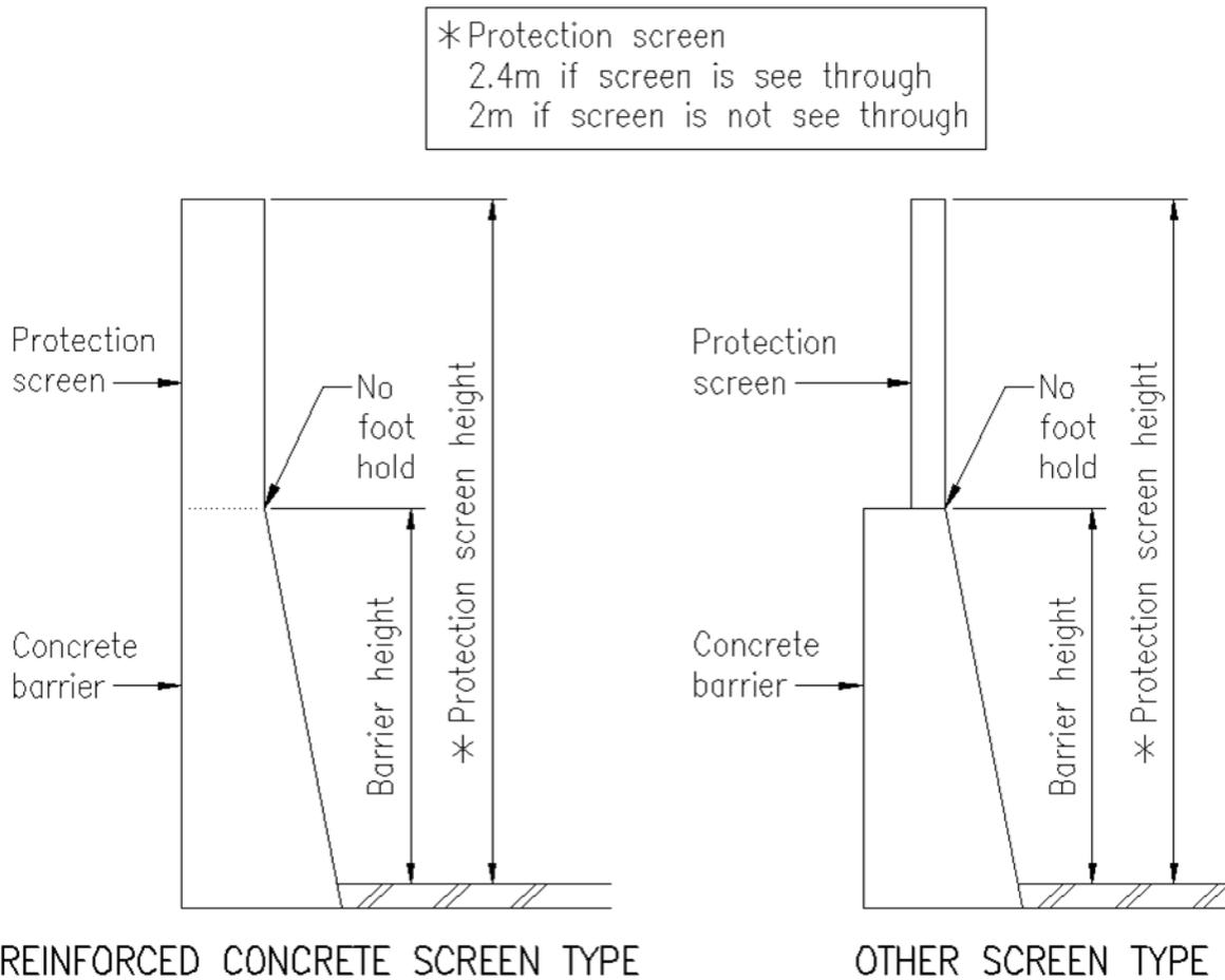
**Additional Design Criteria for Barriers on Bridges over QR Railway that is Electrified**
