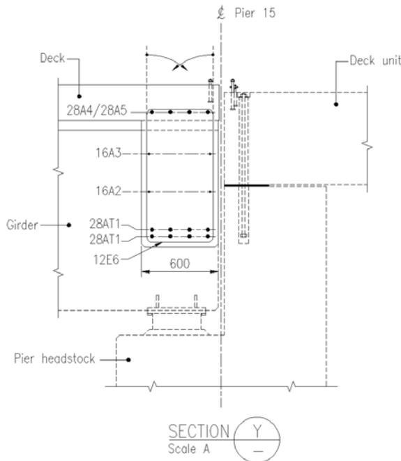
**Welded laps of reinforcement**
