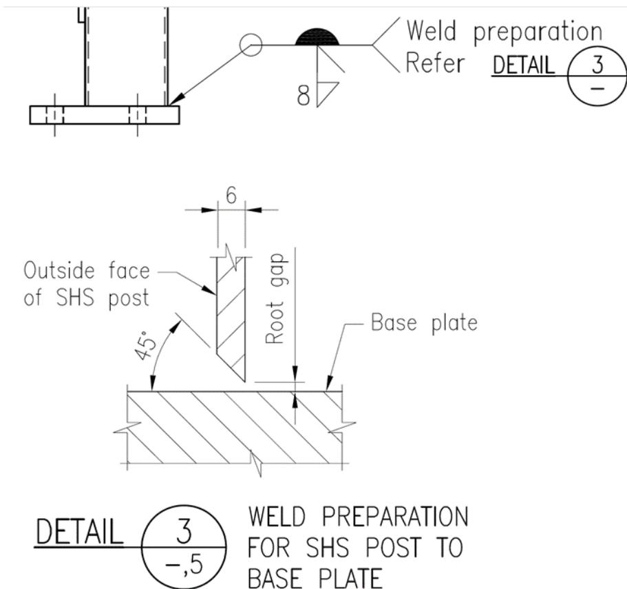
**Figure 6.8-7 - Combination Butt and Fillet Welds**
