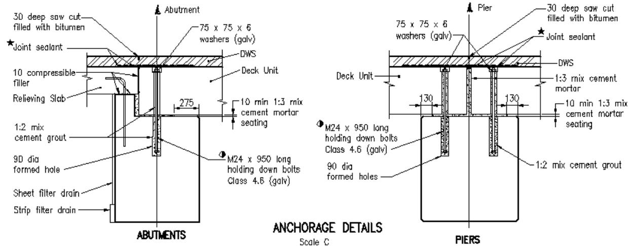
★ All joints to be treated with hot applied bitumen based joint sealant as follows:
