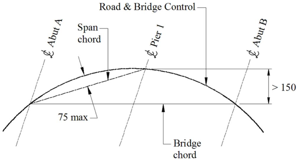
**Figure 10.4-4 - Span Offset 150 mm Maximum**
