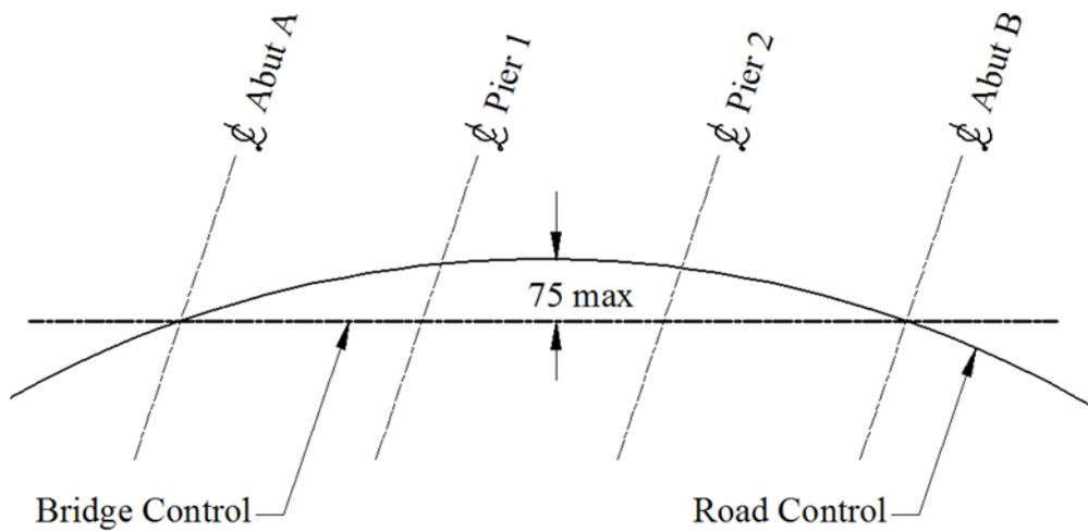
Bridge offset from the chord to the Road Pier is greater than 75 mm but less than 150 mm
