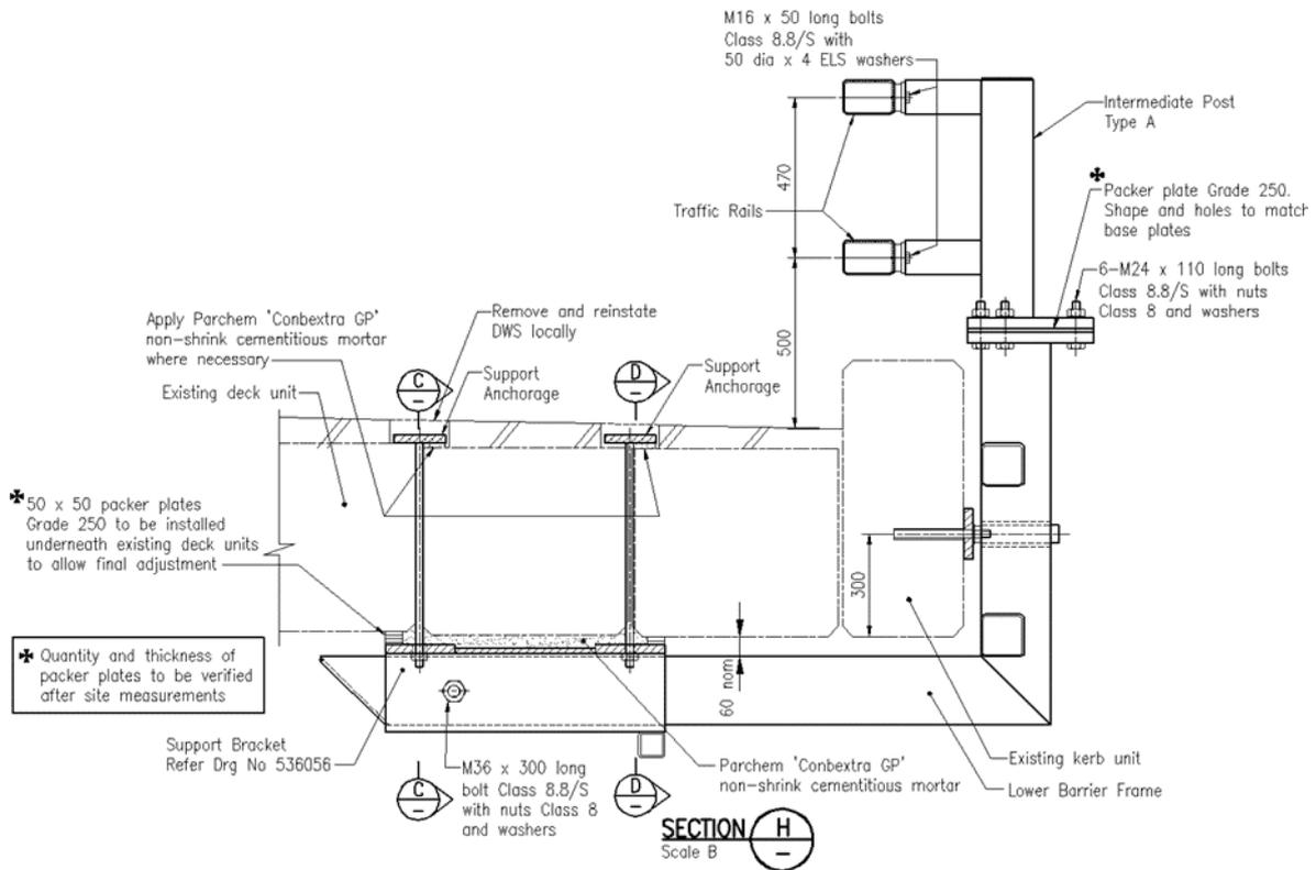
Figure 19.8-2 Example Re-railing (2)
