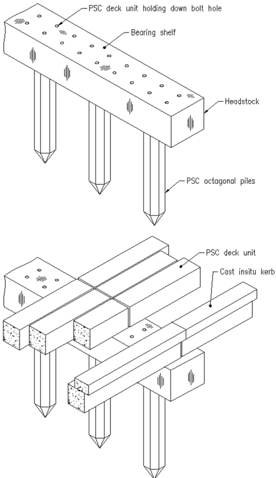
FIXED PIER WITH PSC PILES, PSC DECK UNITS AND CAST INSITU KERBS
