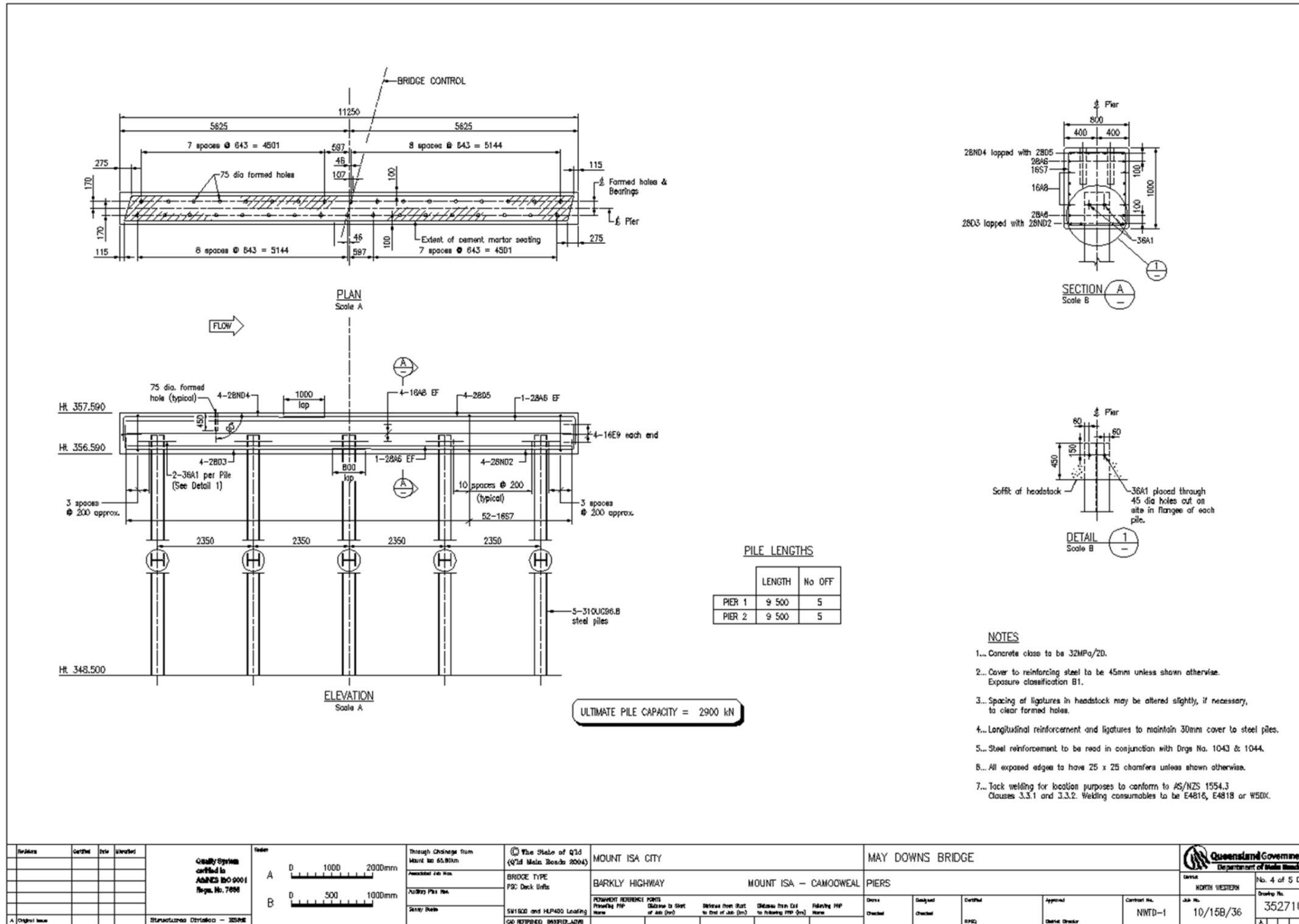
Appendix F – Example Steel Pile and Precast Headstock Drawing
