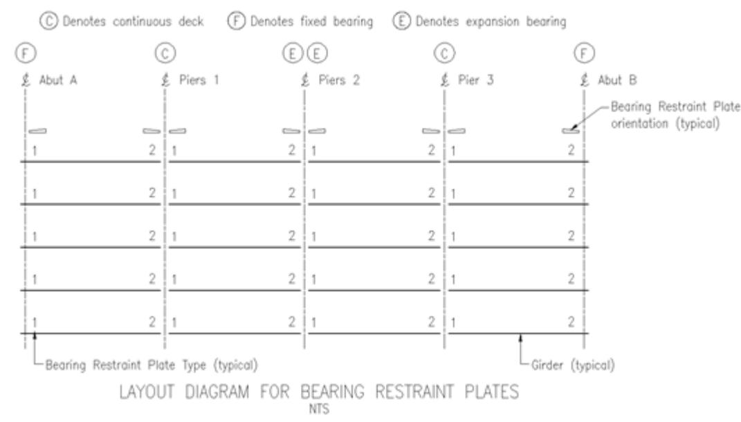
Figure 14.6(b) - Bearing restraint plates
