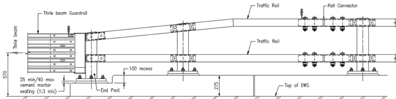
**Bridge steel traffic barrier connecting to W beam guardrail**
