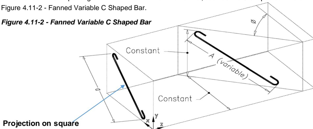
*C bar without dimensions parallel to x and y axis cannot be solved by the steel program*
