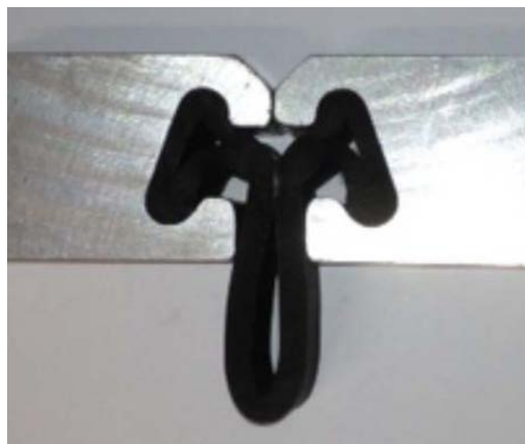
Figure 18.3-2 Draped (D) Seal Minimum Closed Gap
