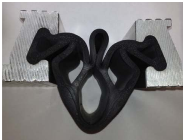
Figure 18.3-1 Flush (F) Seal Minimum Closed Gap
