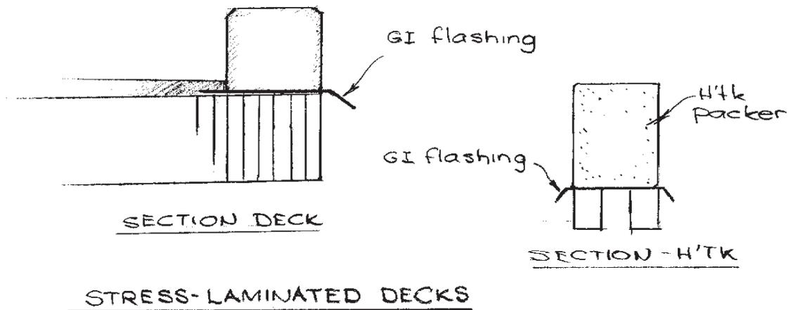
Figure 7.7(b) - Flashing
