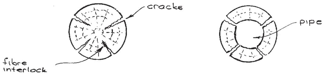
Figure 4.2(c) - Cracked Girder Sections
