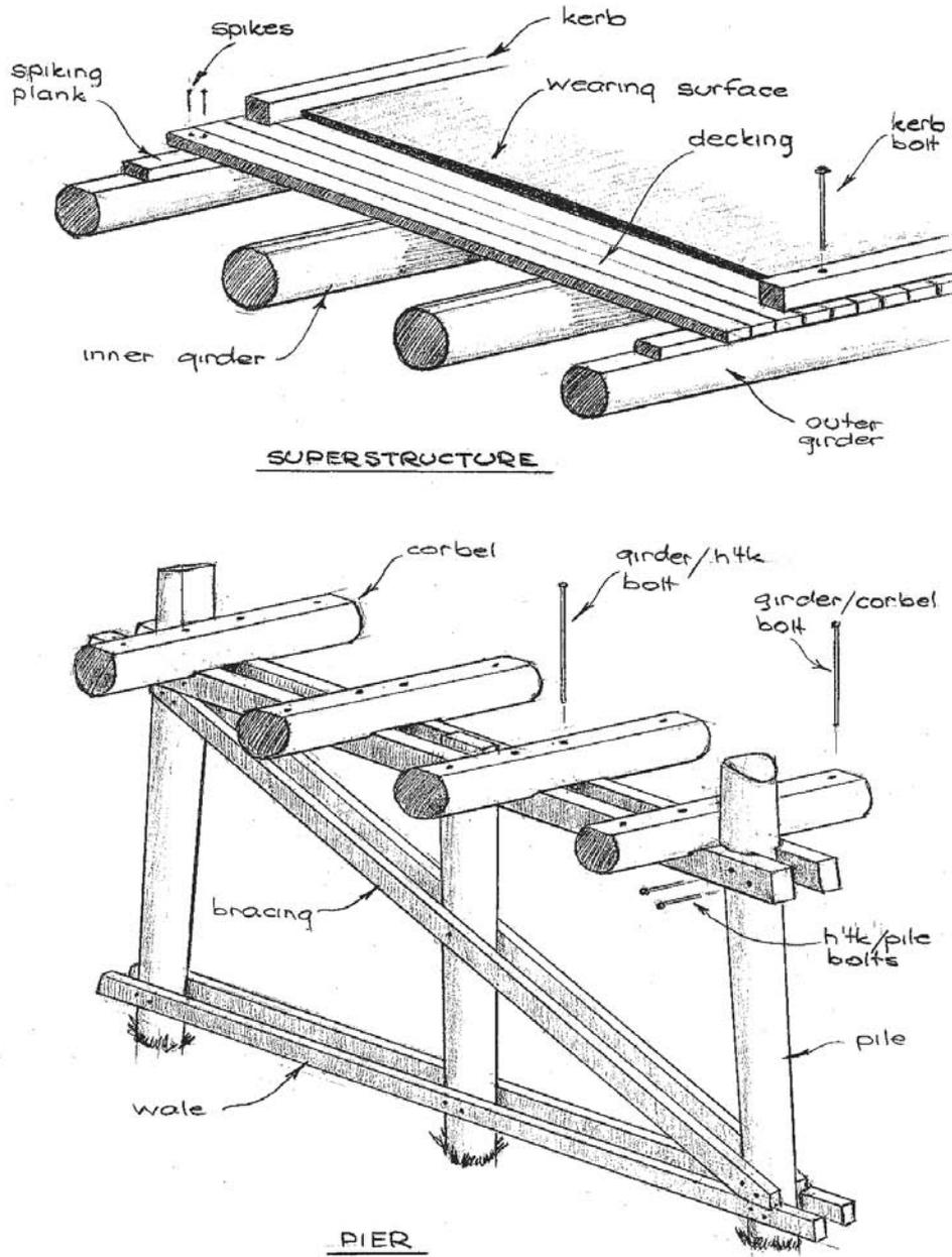
Figure 3.3(b) - Timber Bridge Details
