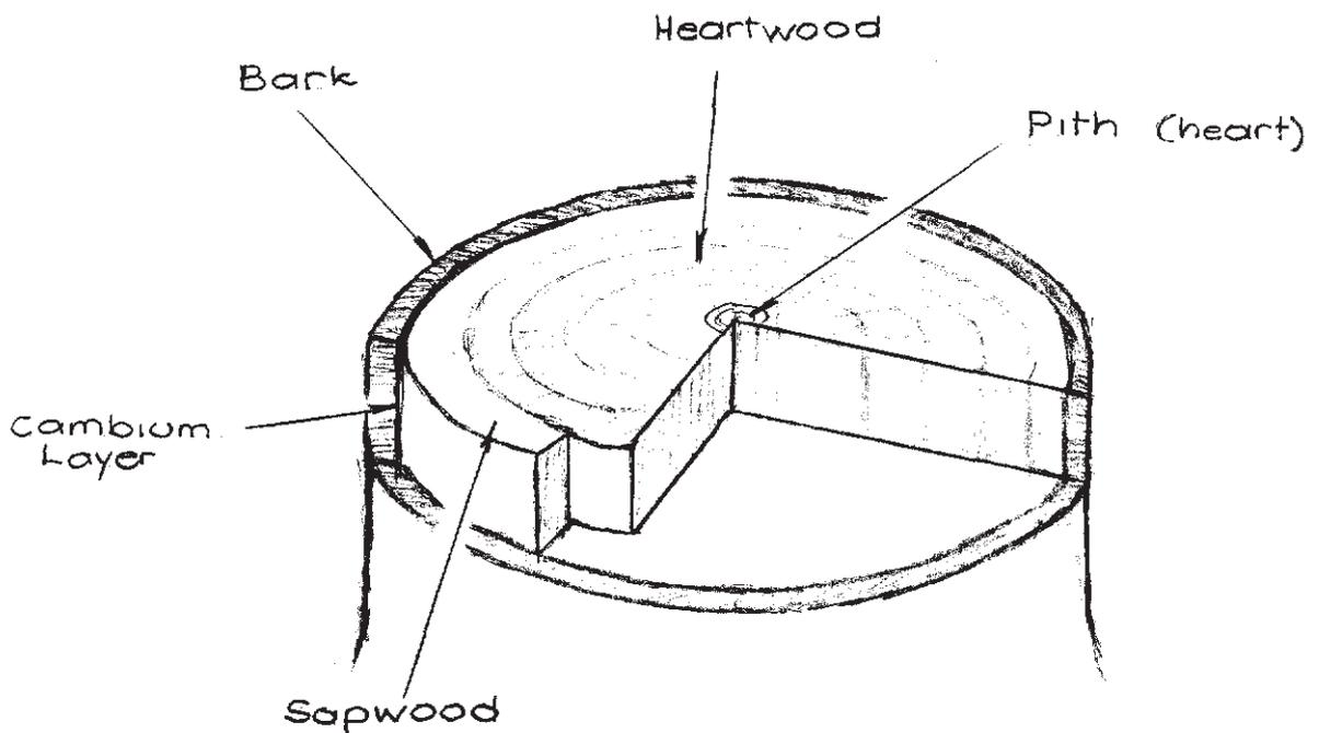
Figure 4.1(b) - Section - Tree Trunk
