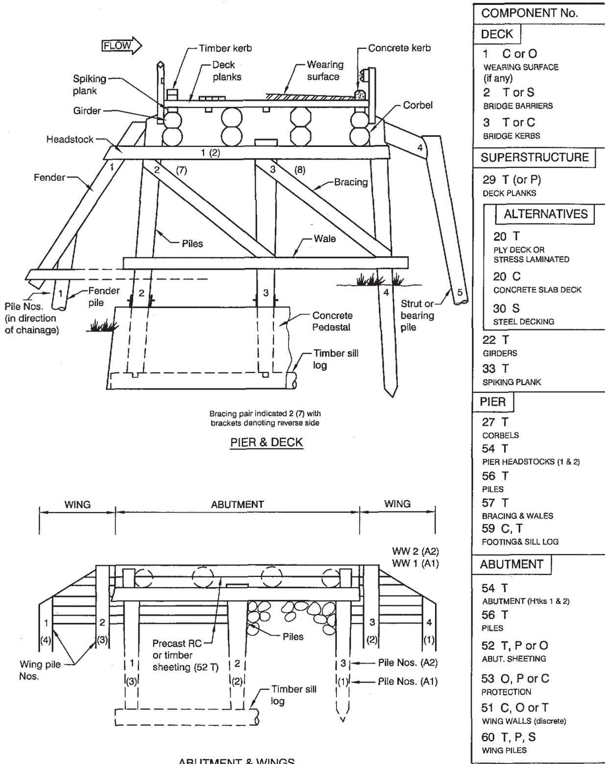
Figure 3.5(b)- Typical Timber Bridge
