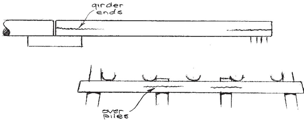
Figure 4.2(b) - Expected Shear Failure Locations
