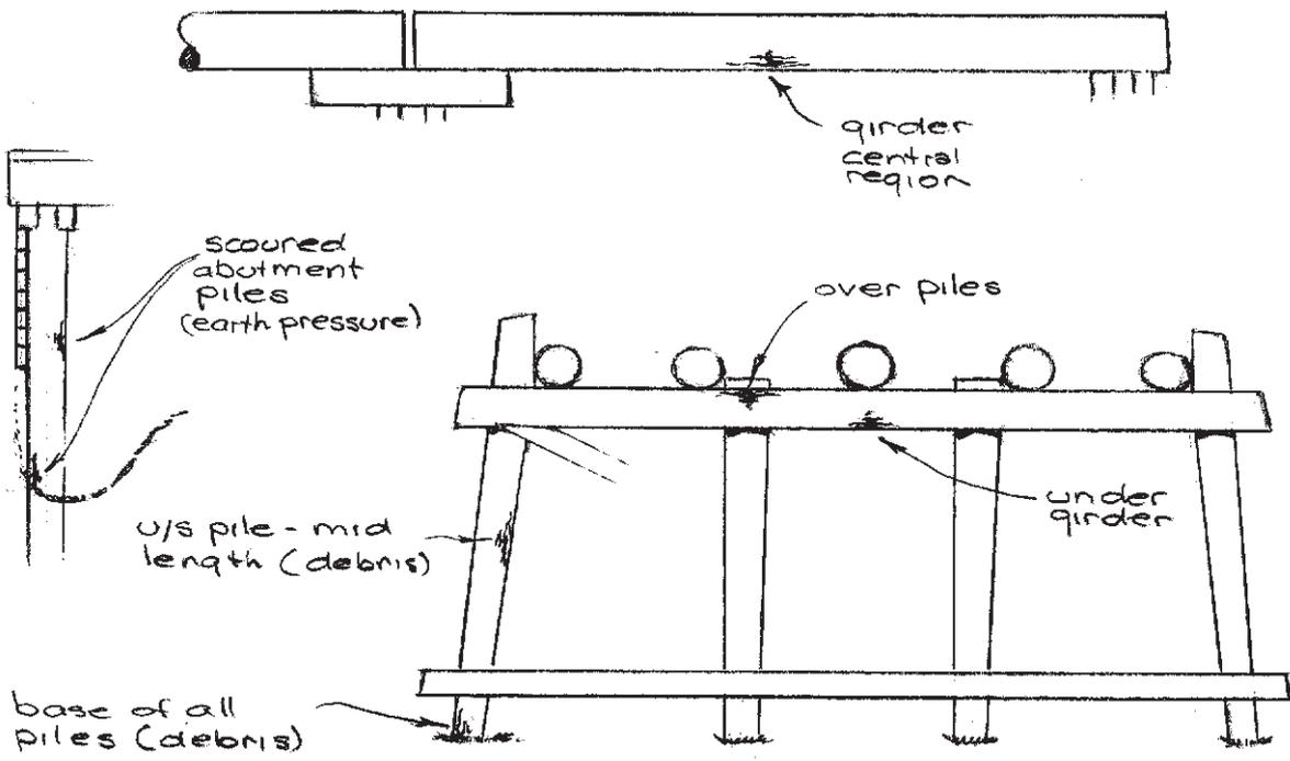
Figure 4.2(a) - Expected Bending Failure Locations
