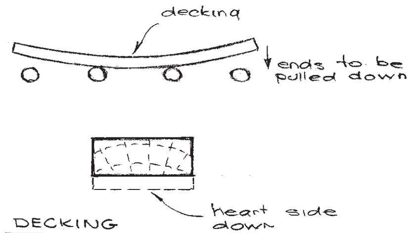
Figure 4.5 - Cuts For Sawn Timber
