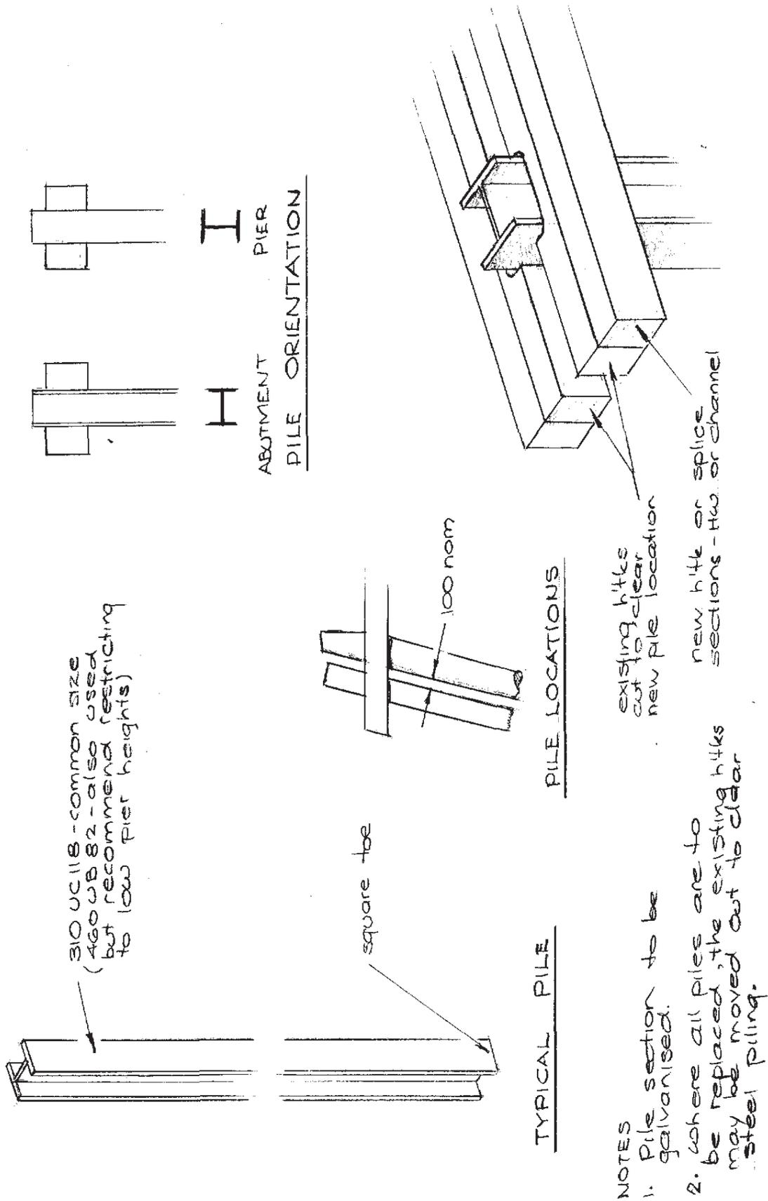
Figure 11.2(a) - Steel Piles (1)
