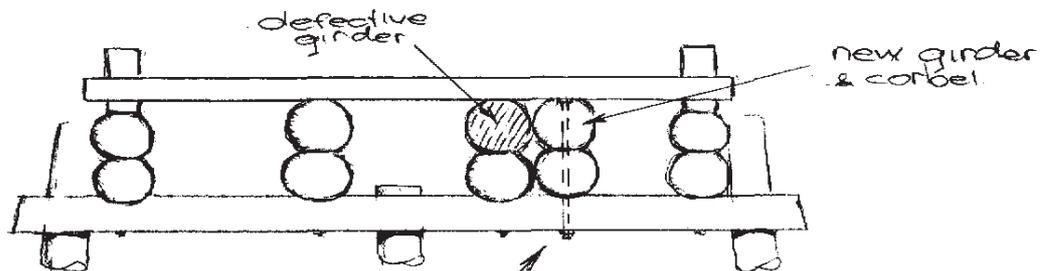
\* Note that additional girder lines can produce increased bending in h/les. A structural assessment is required before installation.
