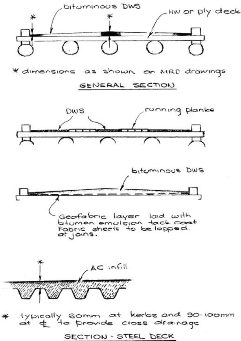
Figure 2.1 - Bituminous Wearing Surface
