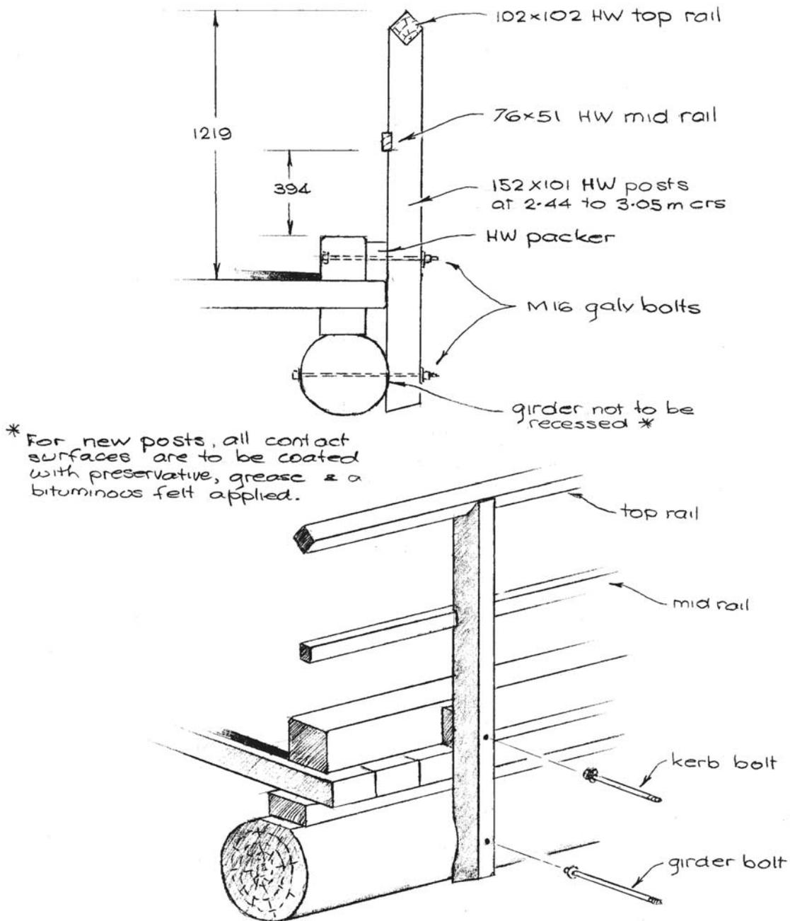
Figure 3.1 - Timber Barrier
