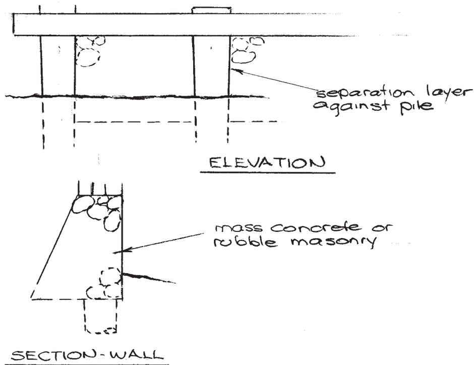
Figure 15.3 - Concrete / Masonry infill walls
