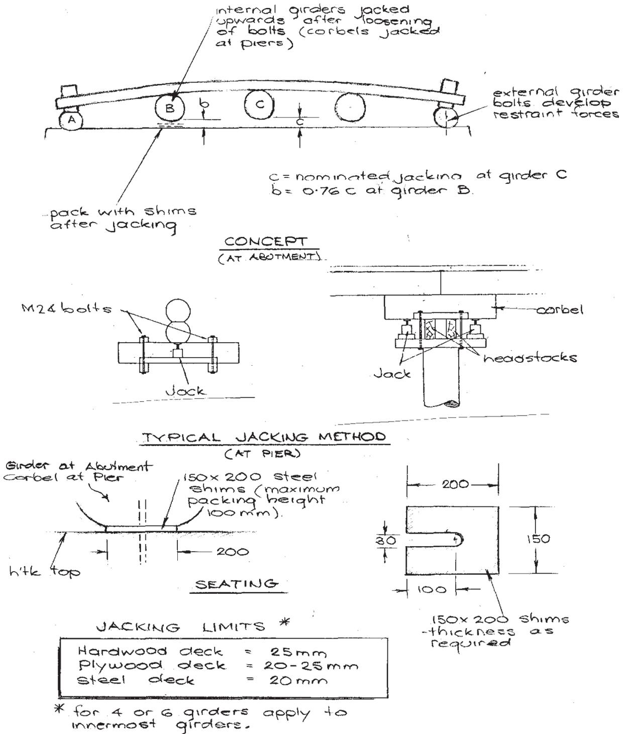
Figure 17.9 - Deck Recambering
