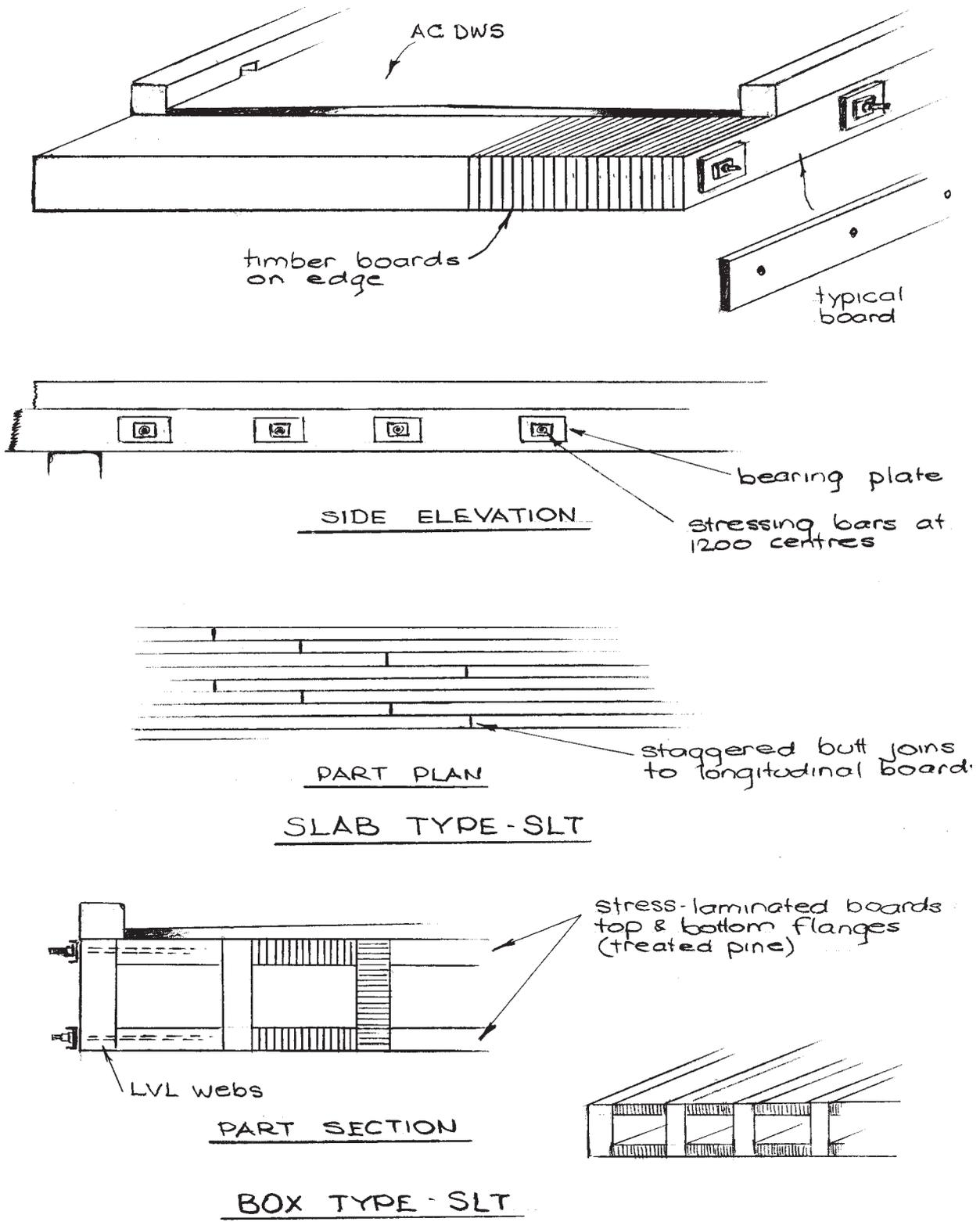
Figure 5.9(a) - Stress-laminated Timber Deck
