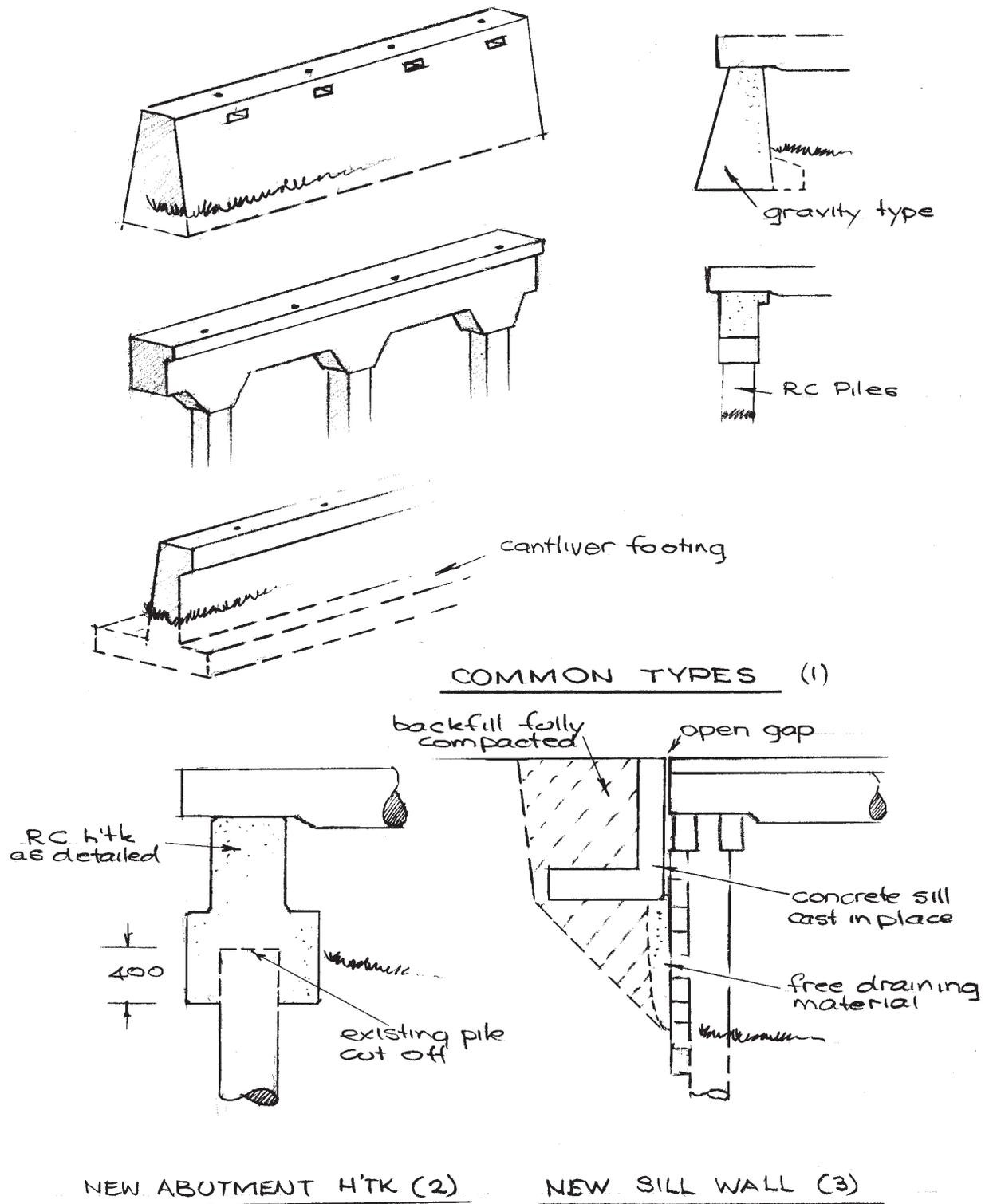
Figure 14.1 - Concrete Abutment
