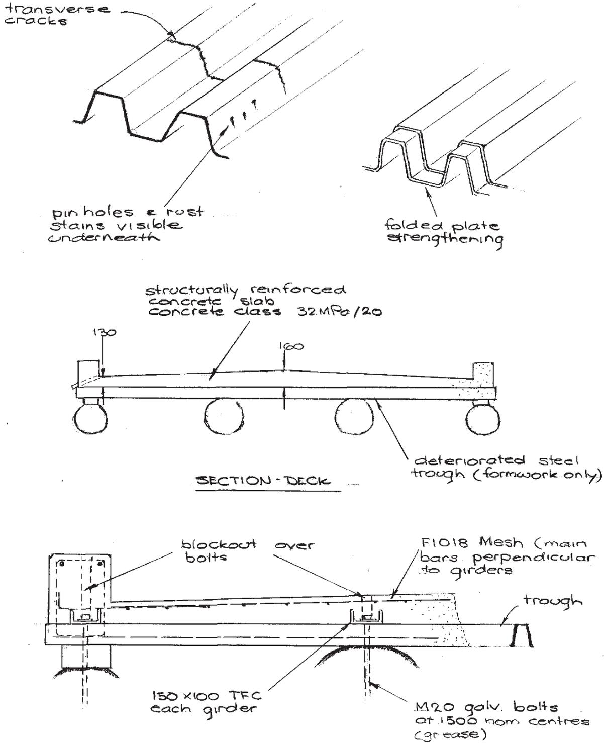
Figure 5.5(c) - Concrete Slab
