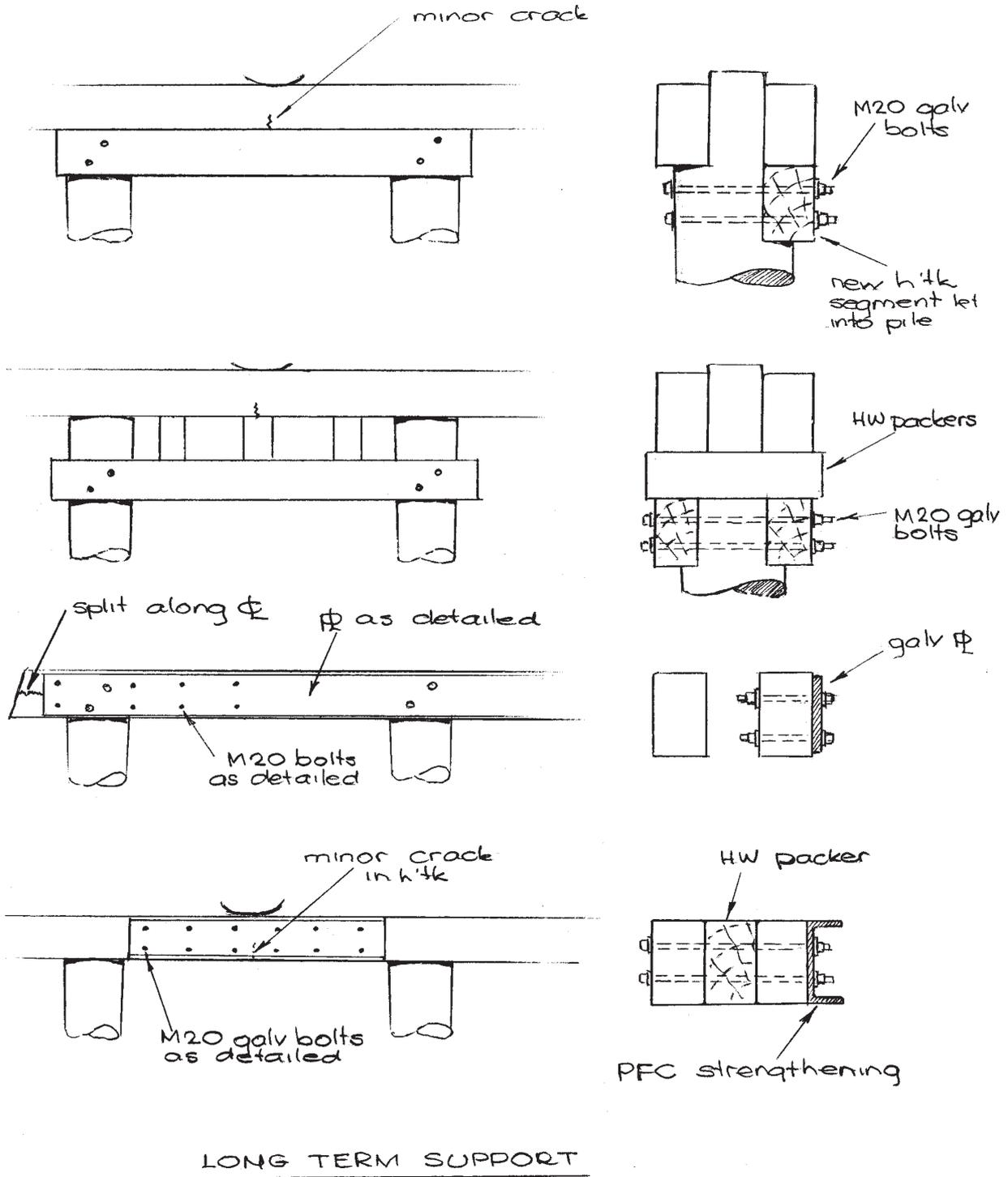
Figure 10.1(d) Headstocks - Supplementary Supports
