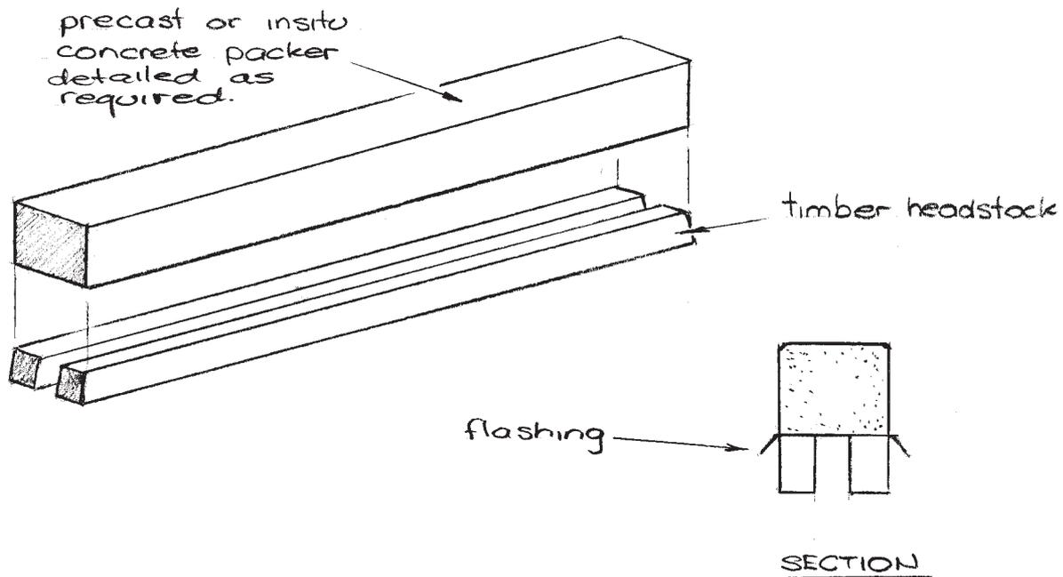
Figure 10.4 - Concrete Packers
