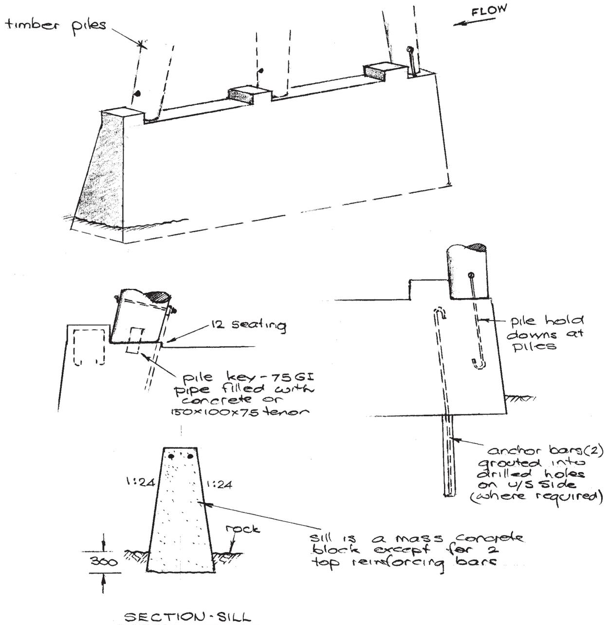
Figure 13.2 - Concrete Sill
