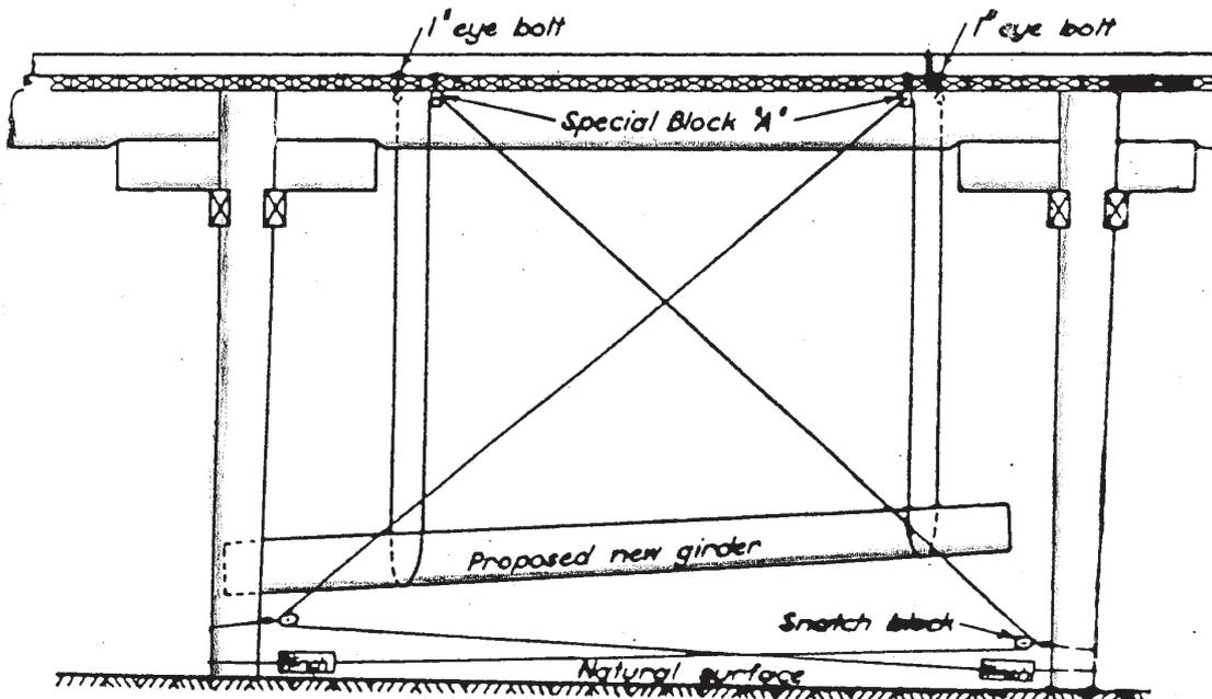
SHOWING METHOD OF LIFTING GIRDER
