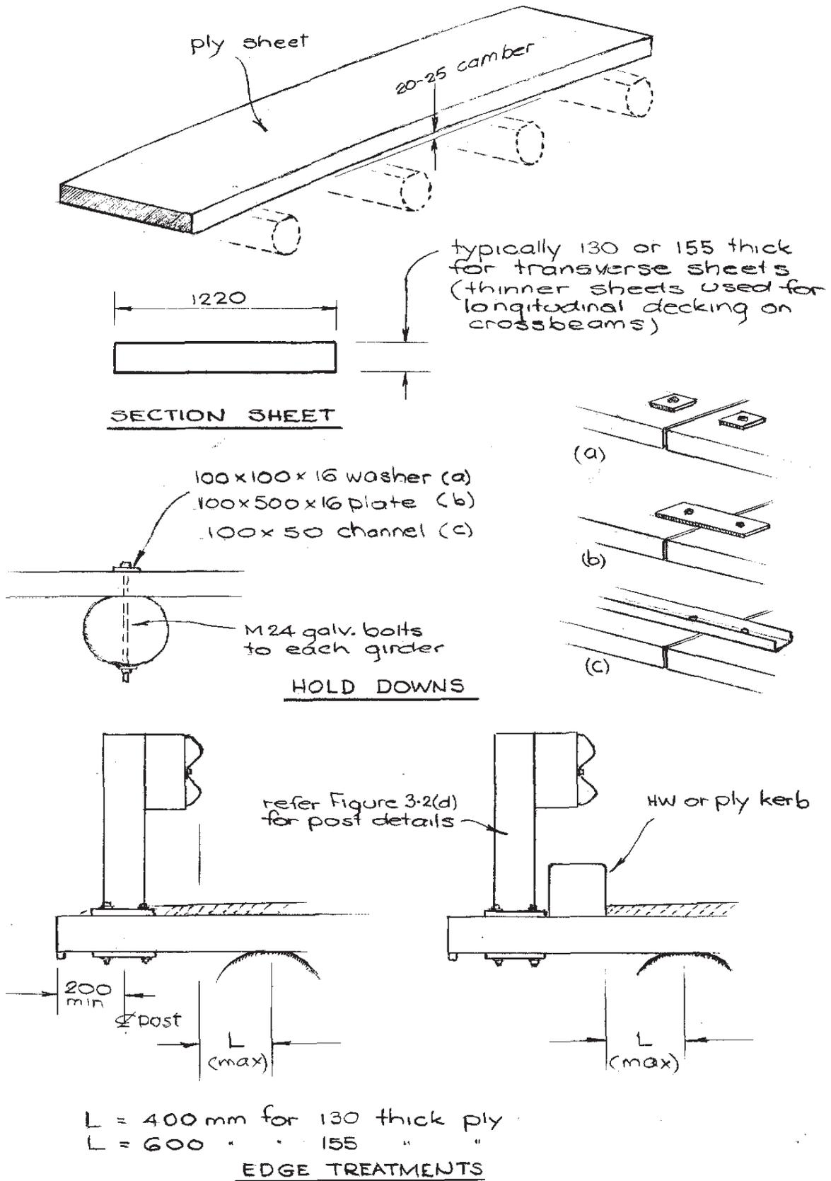
Figure 5.2(a) - Plywood Decking
