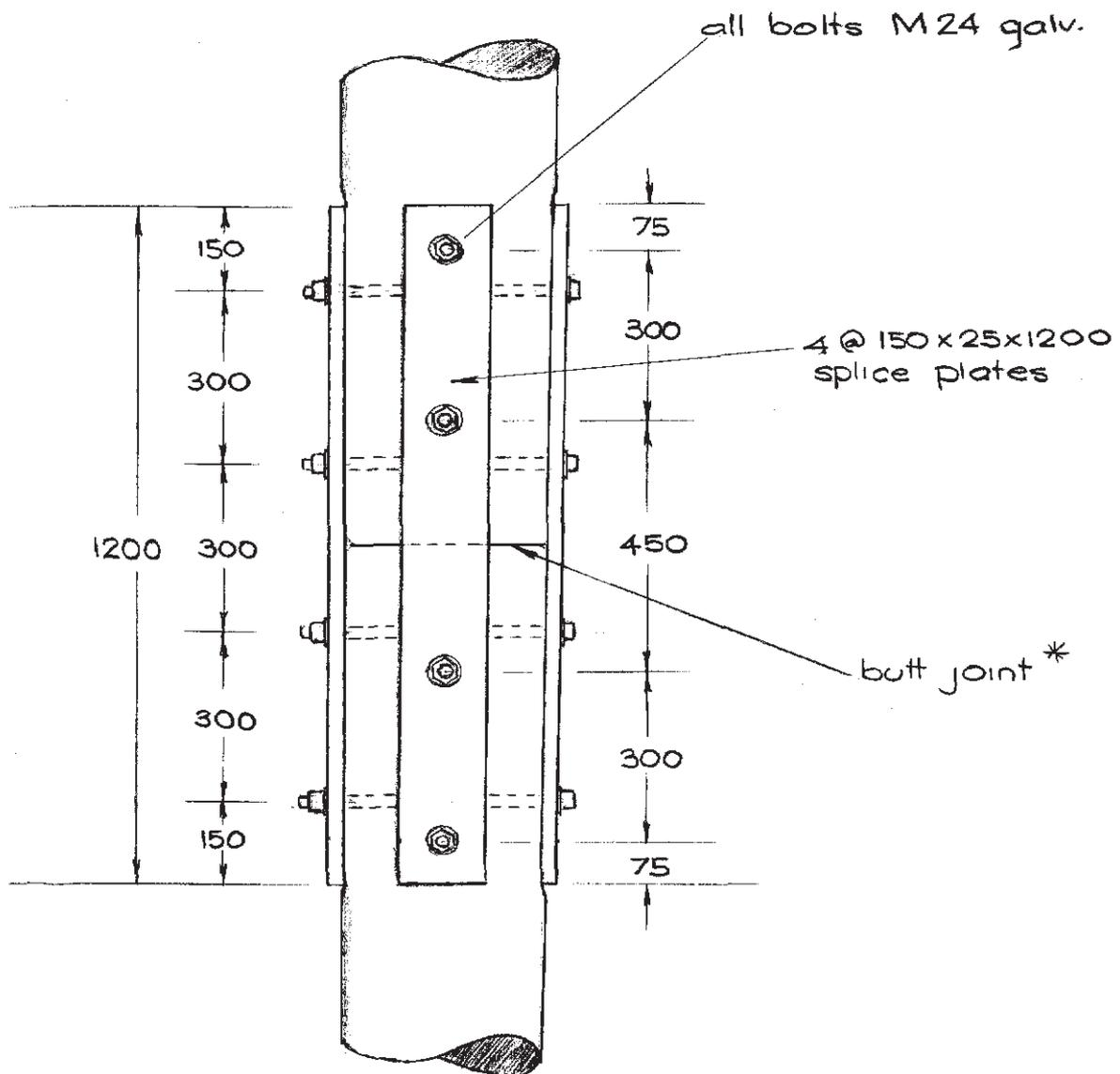
\* butt joint surfaces to be coated with an anti-fungal preservative & grease. It is recommended that a bituminous felt is also placed.
