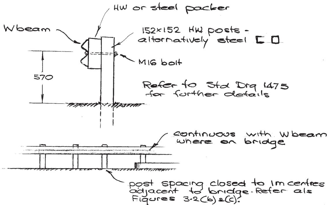
Figure 3.4 - Approach Guardrail
