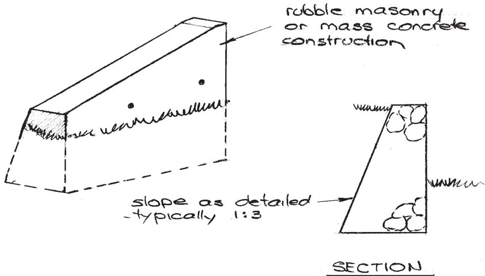
Figure 16.3 - Concrete / Masonry Wing
