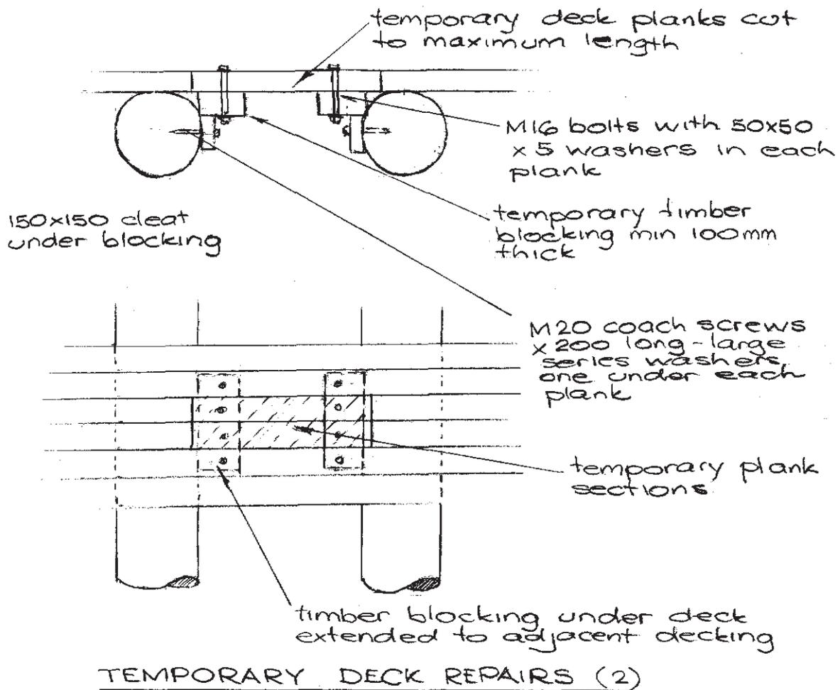
Figure 5.1(c) - Deck Repairs
