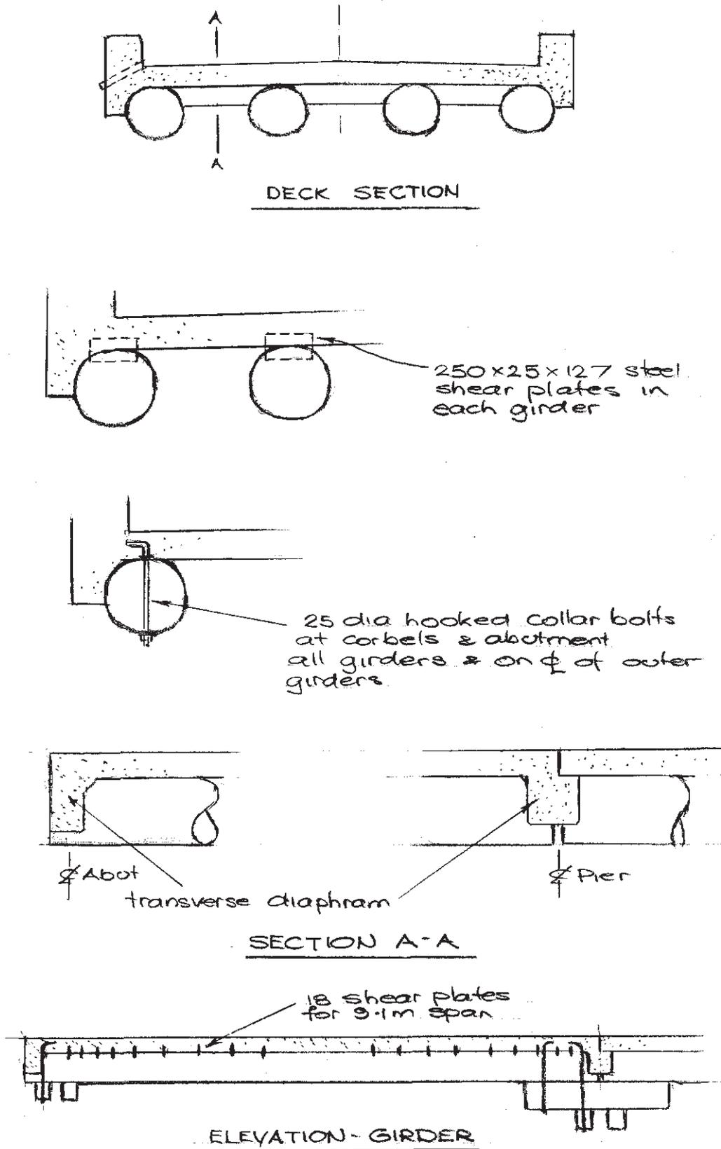
Figure 5.3(b) - Concrete Slab Deck - Type 2
