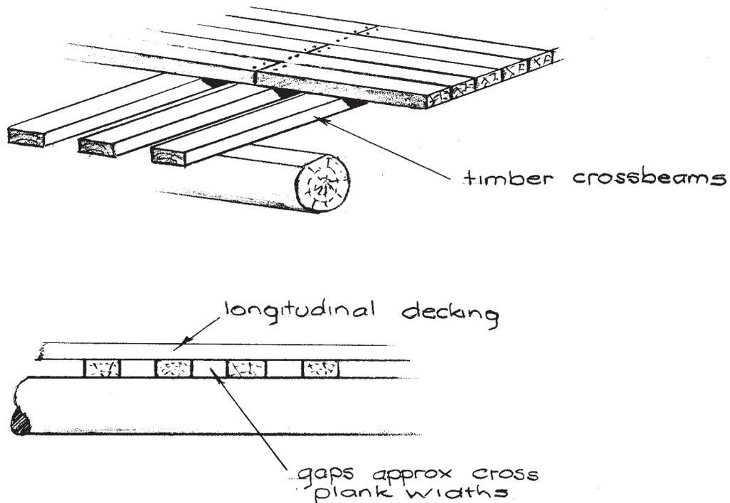
Figure 5.6 - Timber Crossbeams
