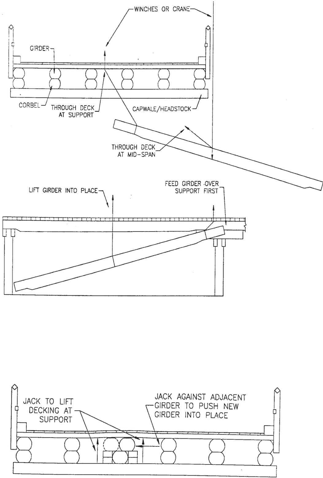
Figure 8.1(j) - Girder Erection 2
