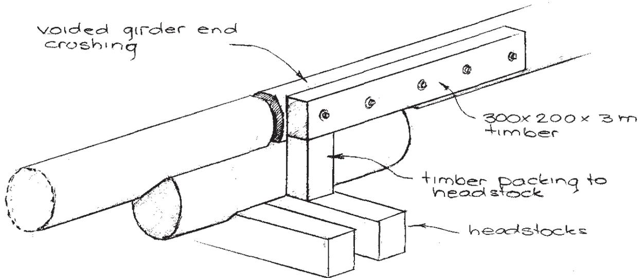
This procedure provides temporary support only & is effective only as long as the girder carries some load.
