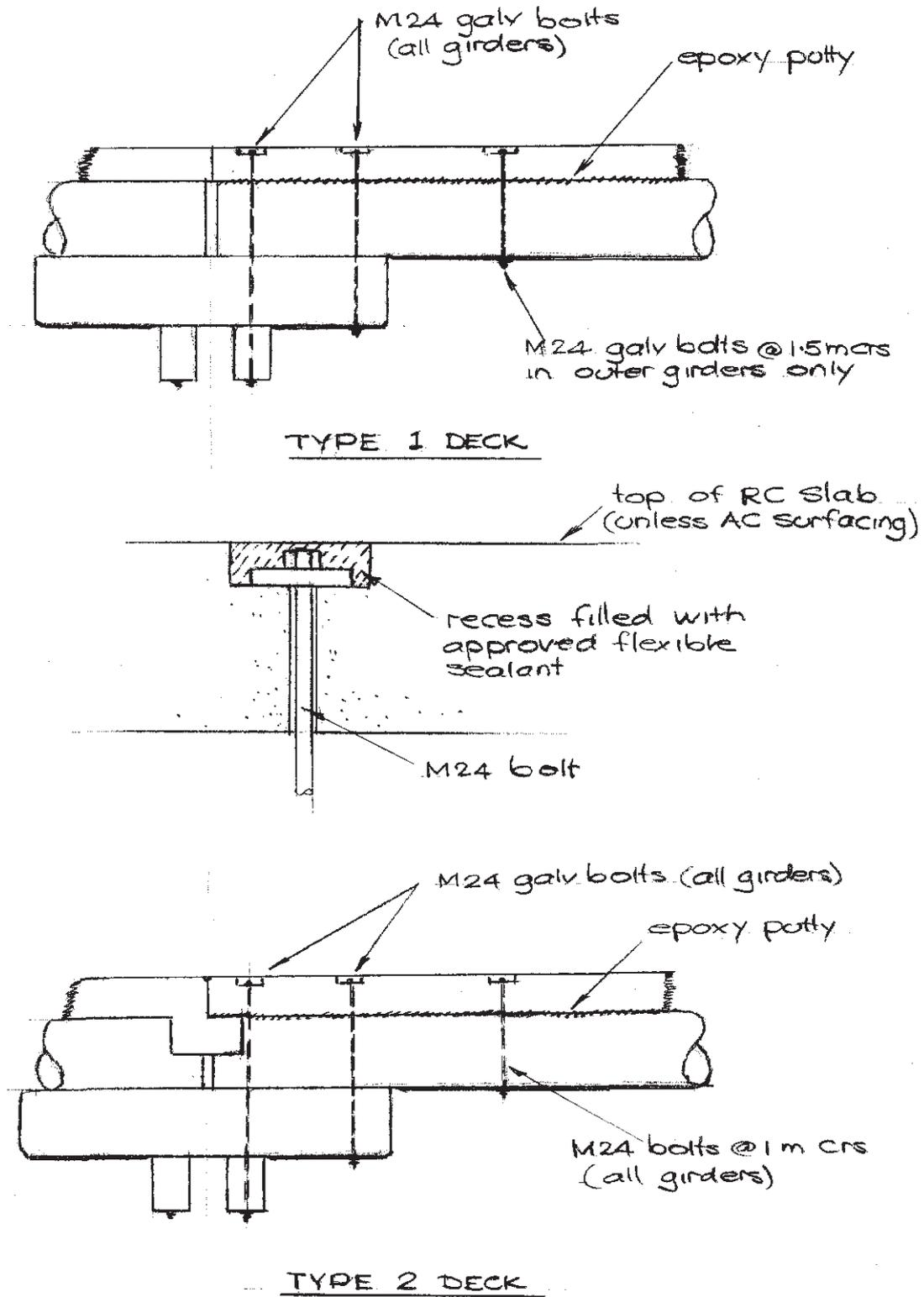
Figure 8.1(k) - Girders - RC Deck
