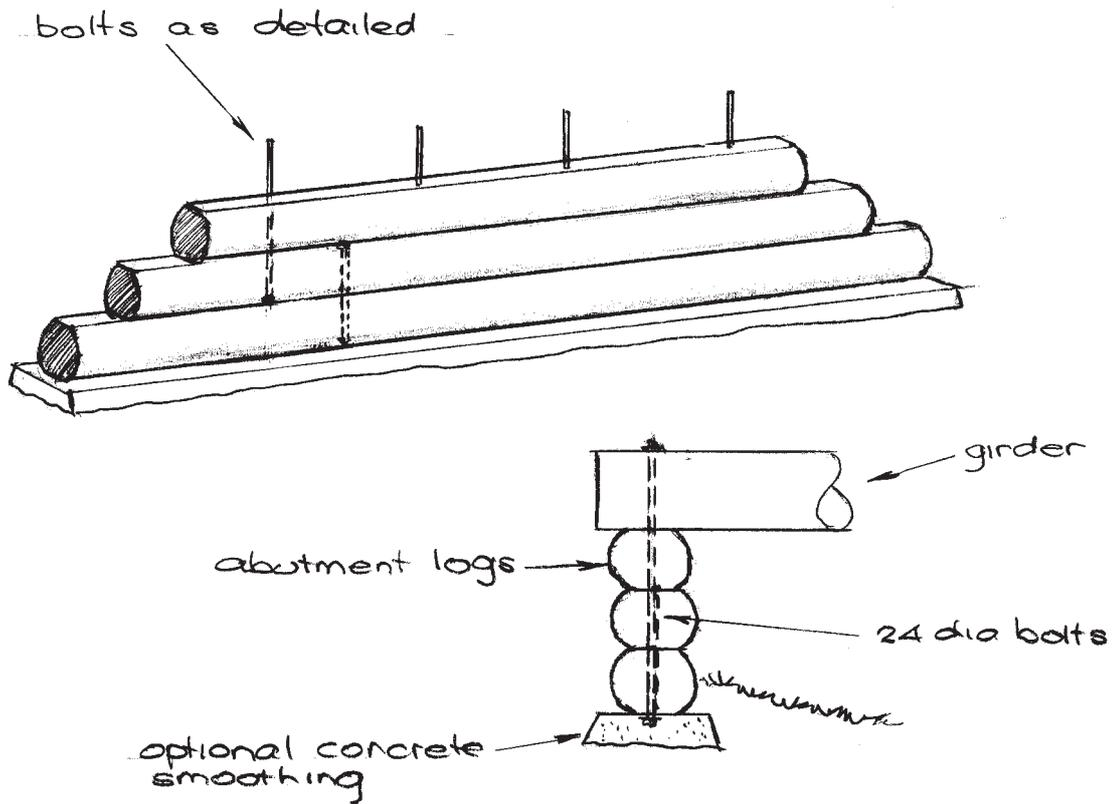
Figure 15.6 - Timber Sill Abutment
