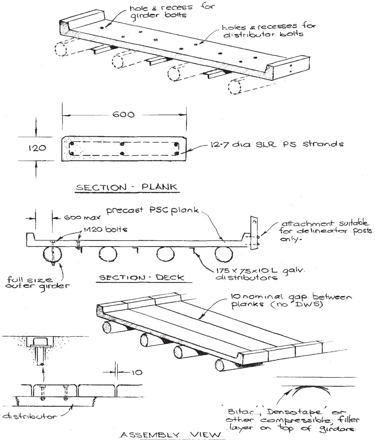
Figure 5.4 - PSC Plank Decking
