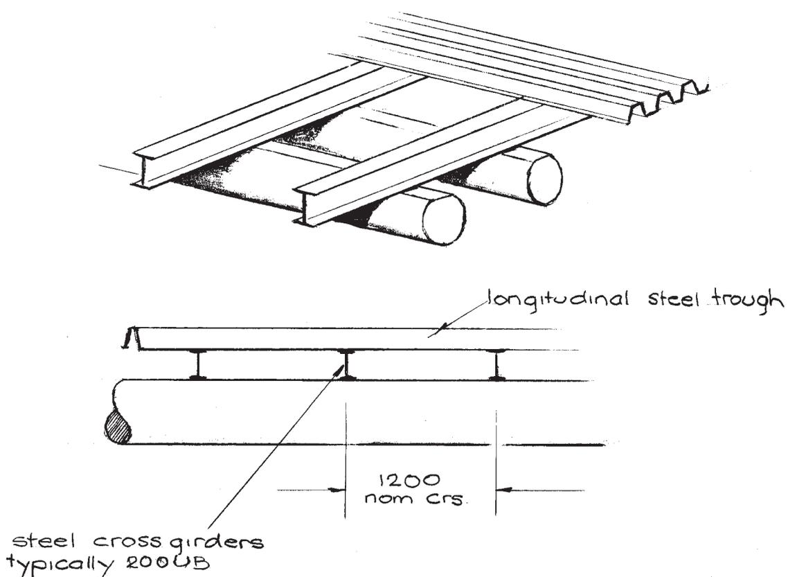
Figure 5.7 - Steel crossbeams
