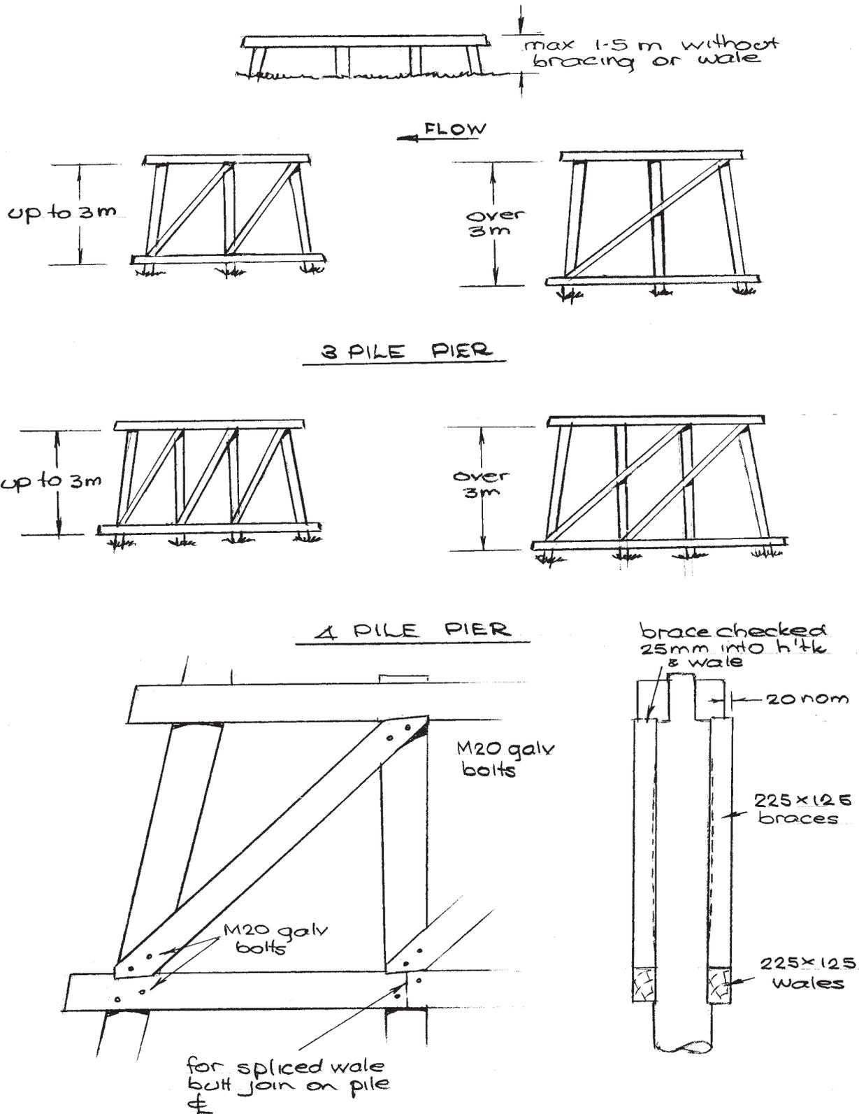
Figure 12.1 - Timber Bracing & Wales
