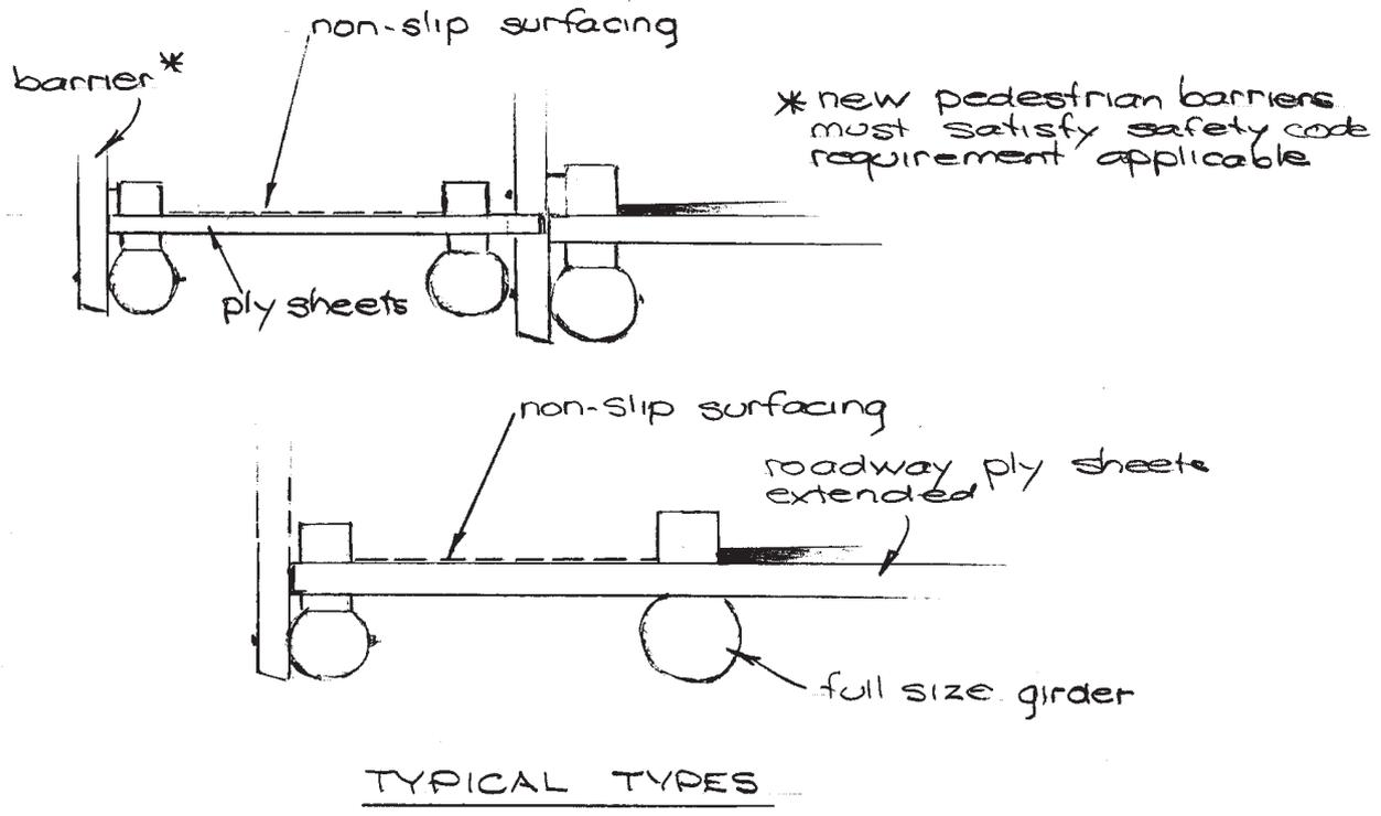
Figure 6.2 - Plywood Footpath
