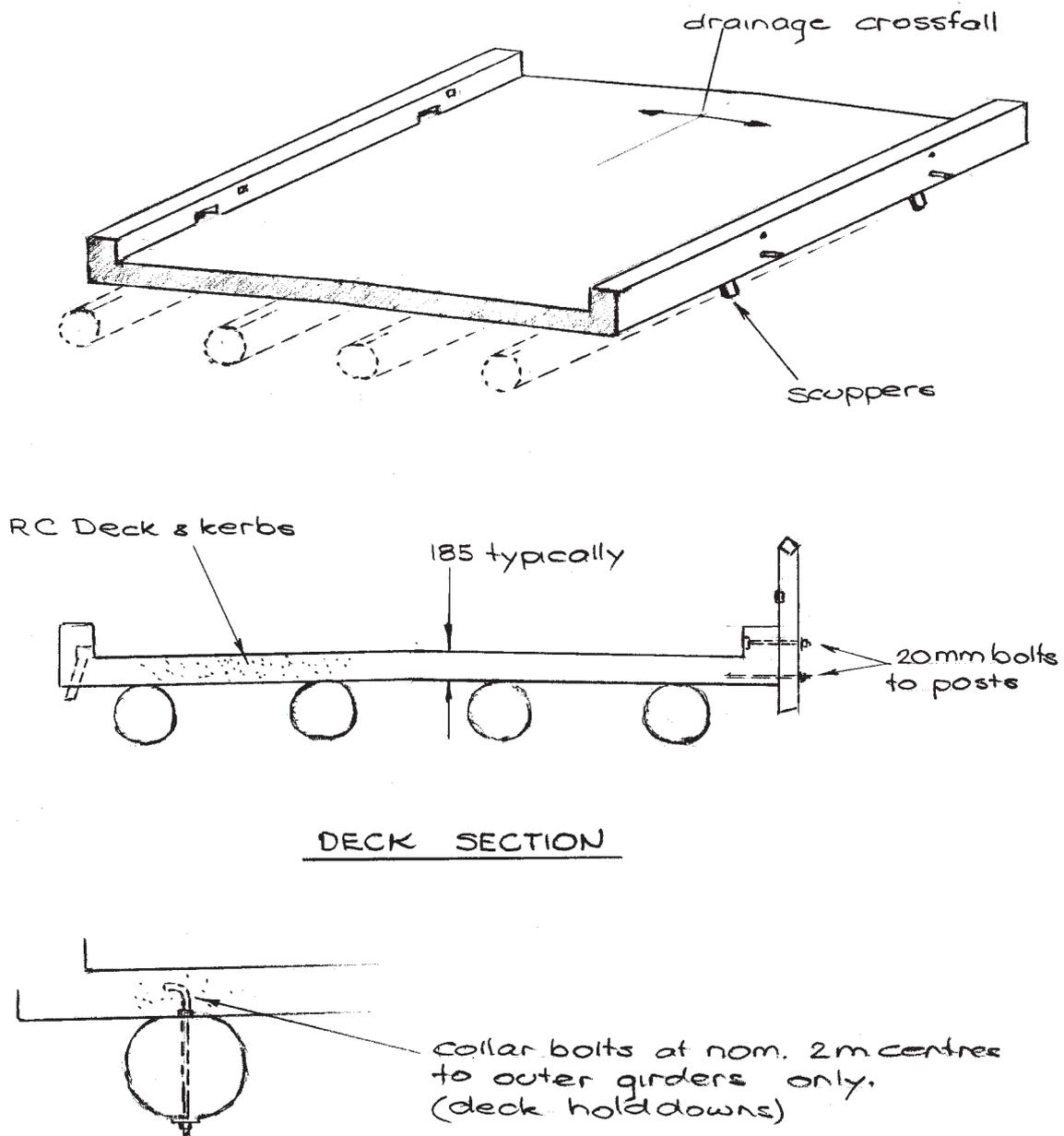
Figure 5.3(a) - Concrete Slab Deck - Type 1
