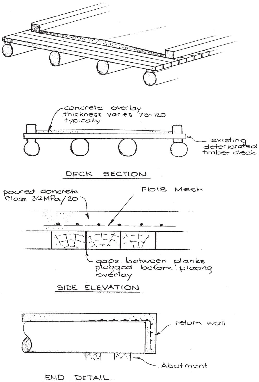
Figure 5.8 - Concrete Overlay
