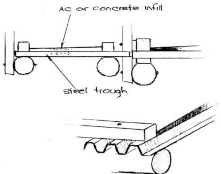
Figure 6.3 - Steel Trough Footpath
