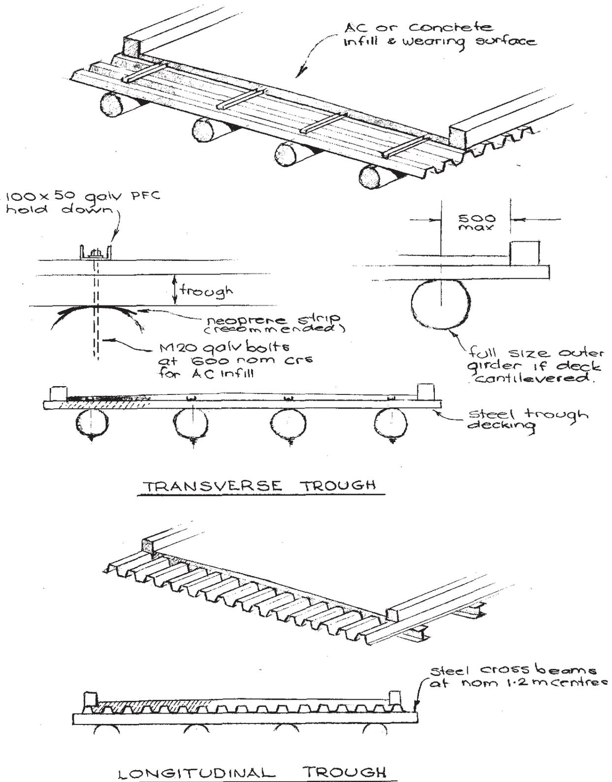
Figure 5.5(a) - Steel Trough Decking
