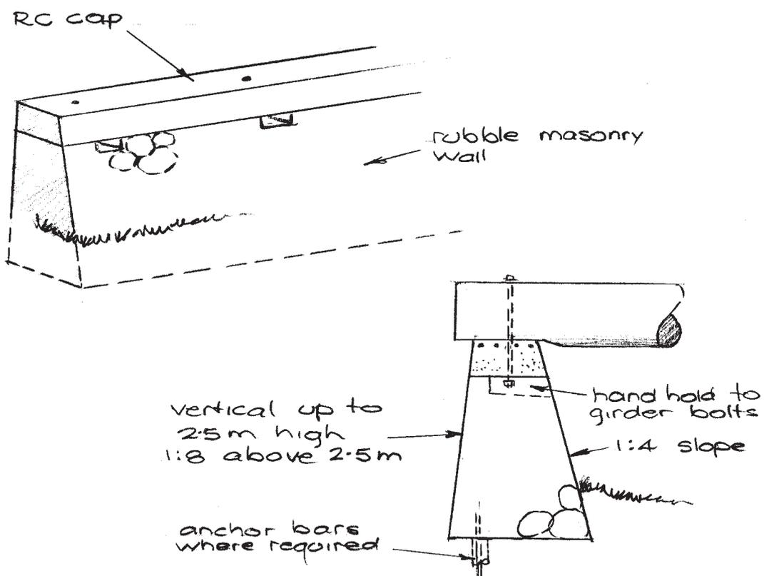
Figure 14.2 - Masonry Abutment
