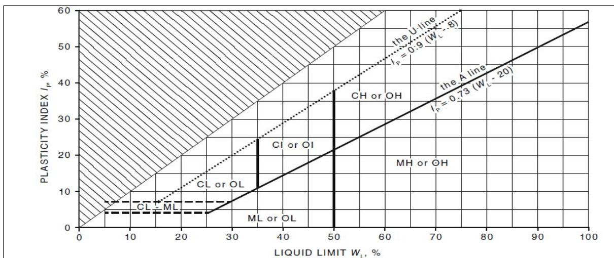
Note: The U line is an approximate upper bound for most natural soils. Data which plot above the U line may represent unusual / problem soil behaviour, or unreliable data and should be considered carefully.
