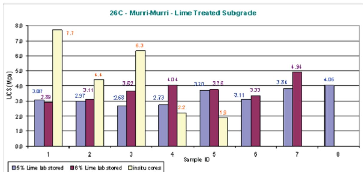
For the 20 cores tested, all results were above 2.0 MPa except for one. It was noted that the exception had the largest length to diameter ratio of all cores.
